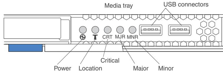
The system-status panel on the front of the BladeCenter T system has five system-status LEDs and two USB connectors.
