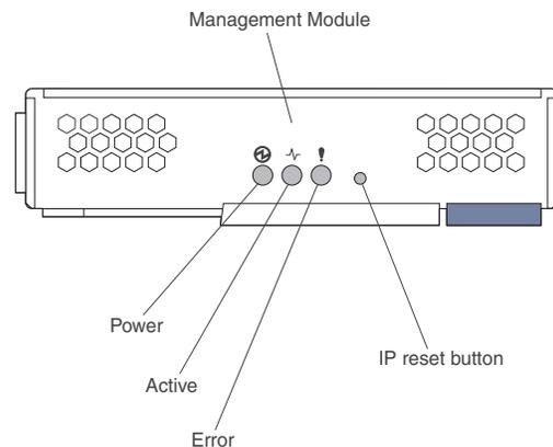
**Management module LEDs:** These LEDs provide status information about the management module and remote management connection.
