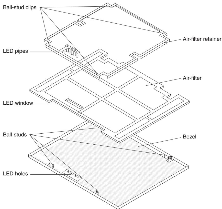
6. Align the LED window of the filter with the holes for the LEDs on the bezel and lay the filter into the bezel frame.
