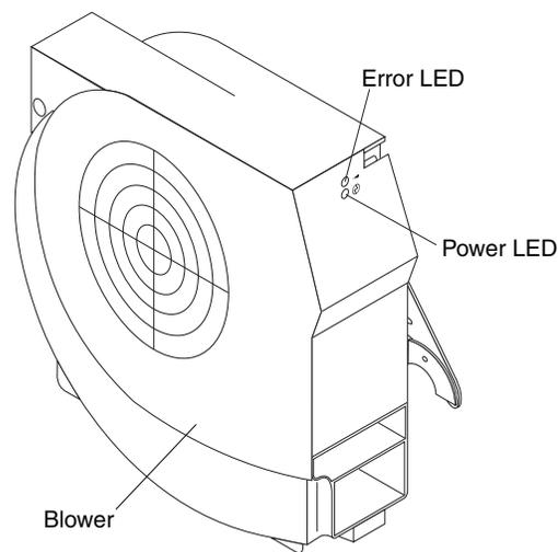
**Important:** Replace a failed blower as soon as possible to restore cooling redundancy.
