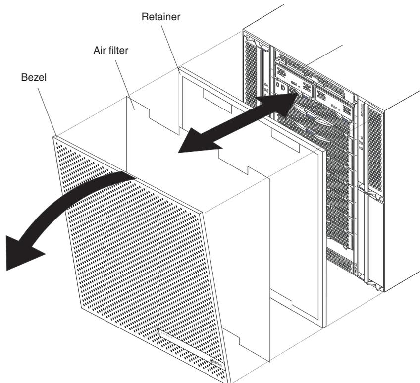
Complete the following steps to replace the front bezel air filter in the BladeCenter T unit:
