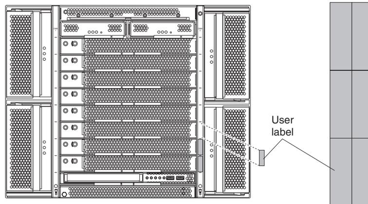
**Important:** Do not place the label on the blade server itself or in any way block the ventilation holes on the blade server.
