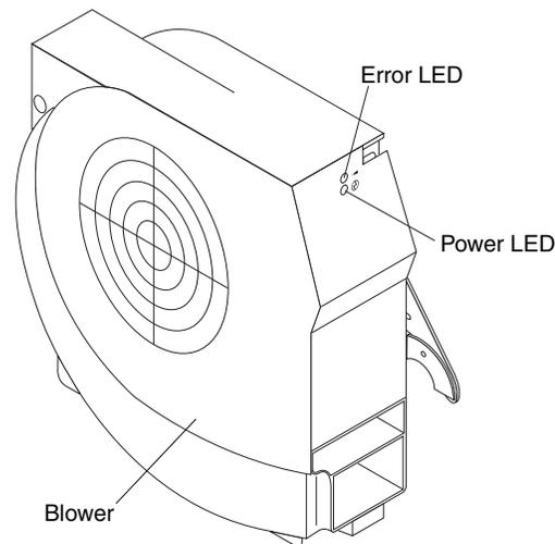
**Blower LEDs:** The LEDs on each blower provide status information about the blower.
