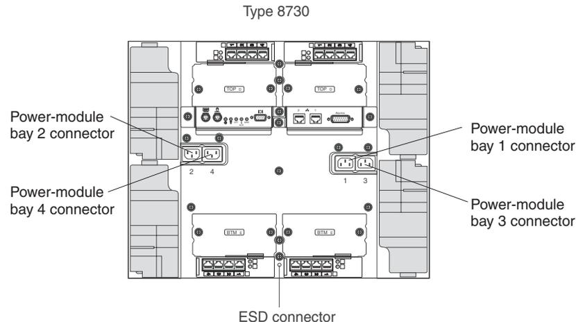
There are four IEC320 power connectors on the rear of the Type 8730 (ac power) unit, marked 1-4 on the rear panel. Power is applied to the corresponding power modules according to the numbering convention on the rear panel. (For example, power connector 1 supplies power to power module 1, and so on.)
