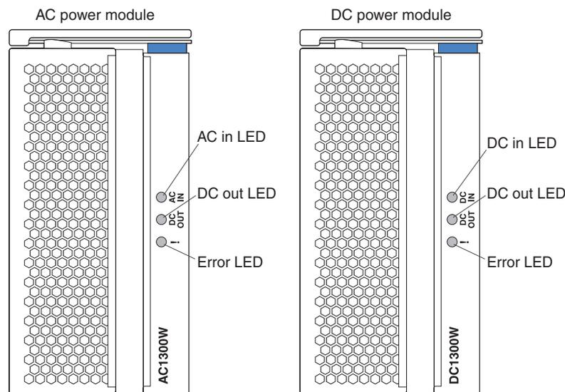
**Power module LEDs:** Each power module has three LEDs to indicate the status of the power module.
