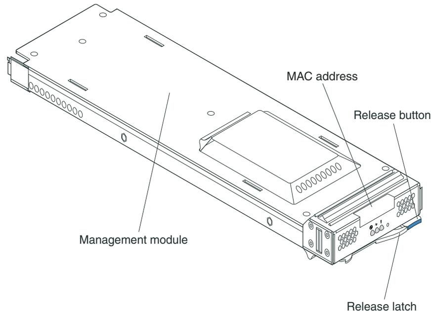
The management module functions as a service processor for the multiple blade servers. The management module configures the BladeCenter T unit and modules, configuring information such as switch module IP addresses. The management module also performs USB-to-PS/2 conversions for the system keyboard and mouse and can send the VGA signal stream to a remote console for viewing. See “Management module controls and indicators” on page 52 for information about the controls and indicators.
