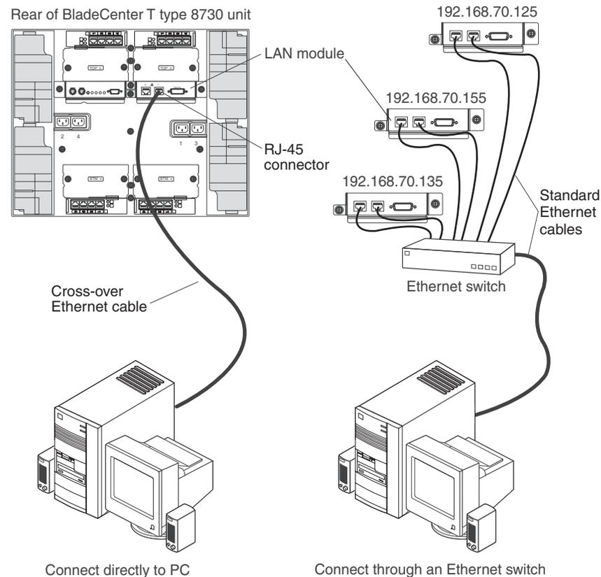
1. Connect one end of a Category 5 or higher Ethernet cable to an Ethernet connector on the LAN module. Connect the other end of an Ethernet cable to the network.
