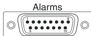
**Note:** The service processor, management module, or systems-management function must monitor the alarm reset inputs to maintain the fault condition that you set for the unit. The alarm reset inputs can be voltages in excess of standard logic levels, so you must electrically or optically isolate them from the monitoring logic.
