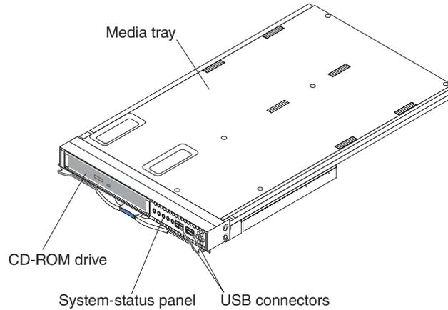
Use the instructions in this section to remove or install the media tray at the front of the BladeCenter T unit.
