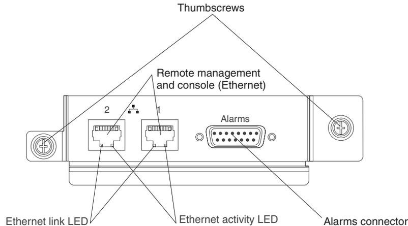
**LAN-module LEDs:** These LEDs provide status information about the LAN connection:
