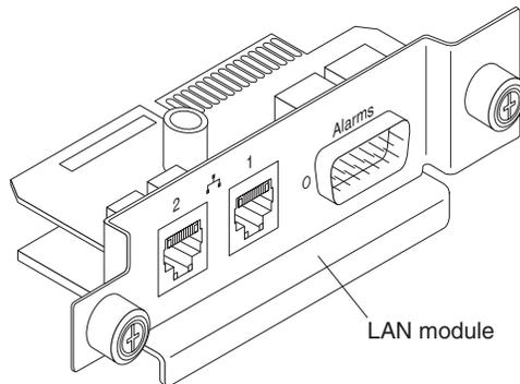
Use the instructions in this section to remove or install the LAN module into the rear of the BladeCenter T unit (see the illustration of the KVM and LAN modules on page 40). The LAN module is held in place by captive thumbscrews. You can either use your fingers or a screwdriver to install or remove the LAN module. If you use a screwdriver, make sure that you do not overtighten the thumbscrews.
