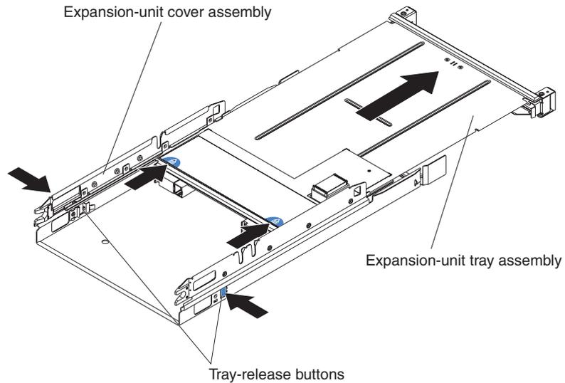
3. Remove the expansion-slot cover from one of the adapter slots by rotating the adapter-retention latch and pulling the slot cover away from the expansion-unit tray assembly as shown in the following illustration.
