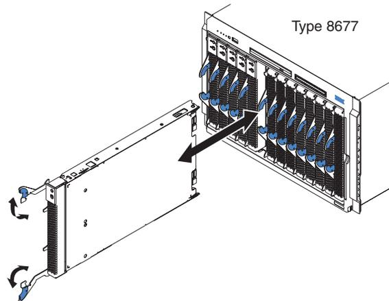
3. Carefully lay the blade server on a flat, static-protective surface.
