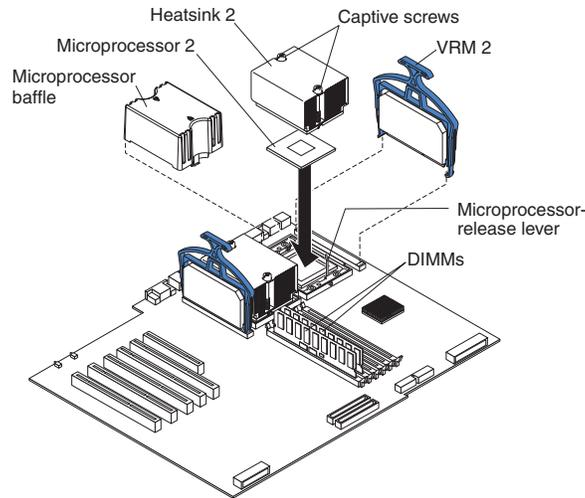
7. Install a VRM in the corresponding VRM connector (J1):
