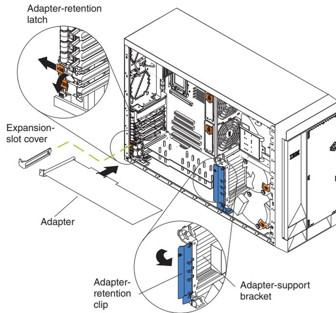
Complete the following steps to install a hot-plug PCI or PCI-X adapter:
