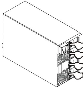
**5** Reinstall and secure the battery doors with captive screws. Make sure that the cords are positioned so that they do not get pinched. Attach the top panels.
