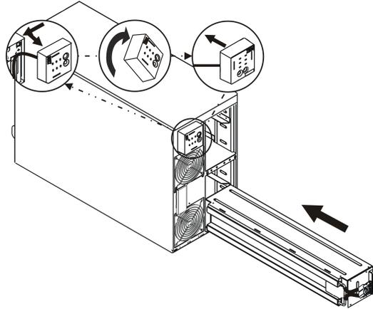
**3** Reinstall the remaining three battery modules.
