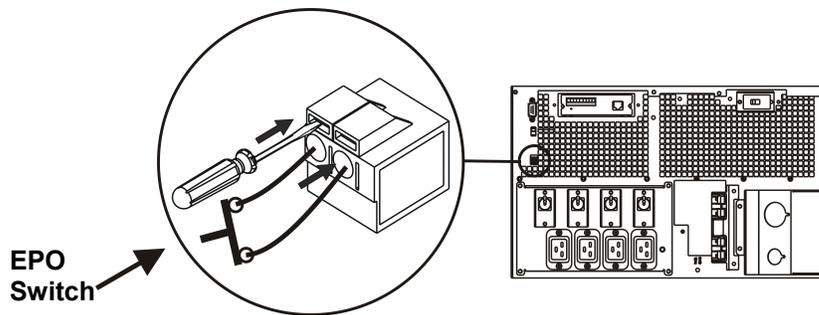
Both Class 2 and SELV circuits must be isolated from all primary circuitry. Do not connect any circuit to the EPO terminal block unless it can be confirmed that the circuit is Class 2 or SELV.
