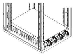
**3** Reinstall the battery door. Make sure that the cords are positioned so that they do not get pinched.
