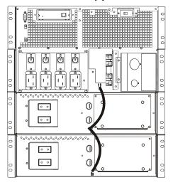
2 Connect to the uninterruptible power supply battery pack outlets (indicated below) using rear panel battery connectors. For multiple battery packs, connect the rear panel battery connectors to the outlets on the nearest battery pack.
