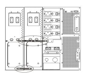
4 Connect the green/yellow ground wire hanging from the battery pack to the TVSS screw on the uninterruptible power supply. For multiple battery packs, connect the wire to the TVSS screw on the nearest battery pack.
