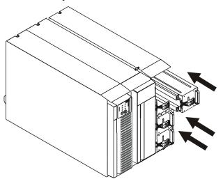
**3** Reinstall the battery door. Make sure that the cords are positioned so that they will not get pinched.
