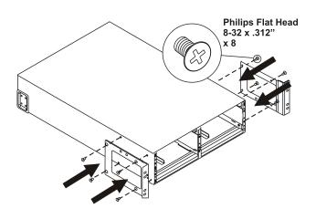
2 Install the rails per the rail installation diagram in the Rail Kit. Install the cage-nuts (or clip-nuts) and mount the battery pack in the rack. **Note:** The battery packs must be mounted below the uninterruptible power supply.
