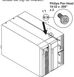
3 Install the rear tie brackets. **Note:** Tie brackets on the center battery pack share a common screw.
