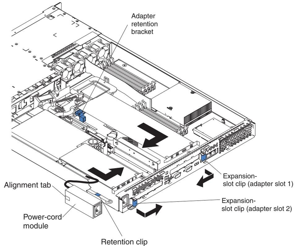
**Attention:** Avoid touching the components and gold-edge connectors on the adapter. Ensure that the adapter is completely and correctly seated in the slot. Incomplete insertion might cause damage to the system board or to the adapter.
