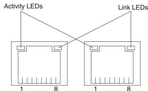
Connect Category 3, 4, or 5 unshielded twisted-pair cables to these connectors. The 100BASE-TX and 1000BASE-T Fast Ethernet standards require Category 5 or higher cabling.
