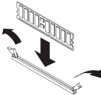
7. Insert the DIMM into the connector by aligning the edges of the DIMM with the slots at the ends of the DIMM connector. Firmly press the DIMM straight down
