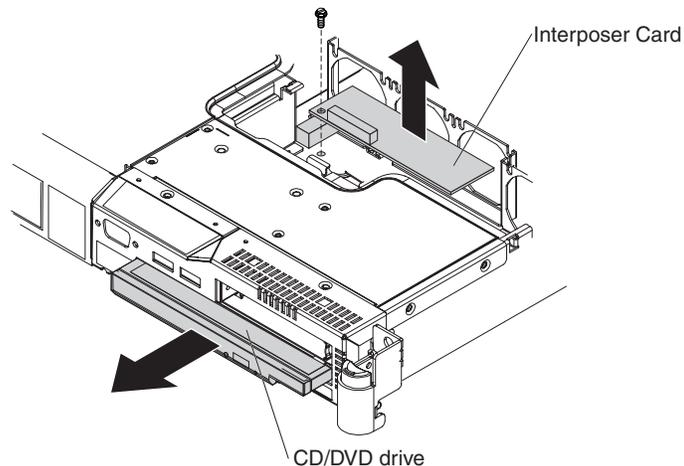
6. Remove the mounting screw from the interposer card and disconnect the CD-RW cable; then, remove the interposer card.
