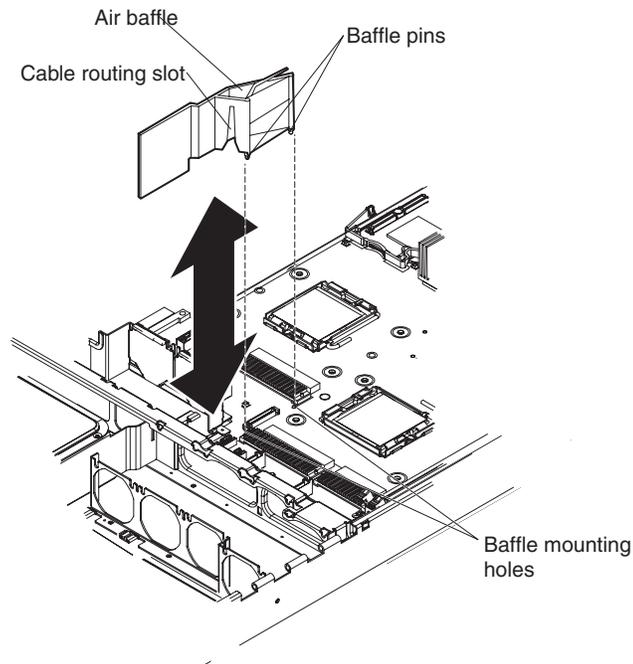
5. Reinstall the air baffle into the system board.
