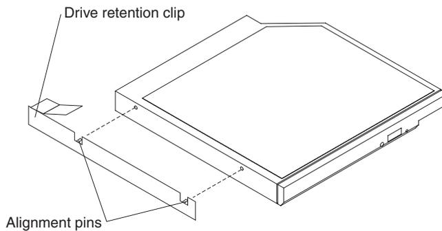
3. Slide the drive-retention clip to attach it to the side of the drive.
