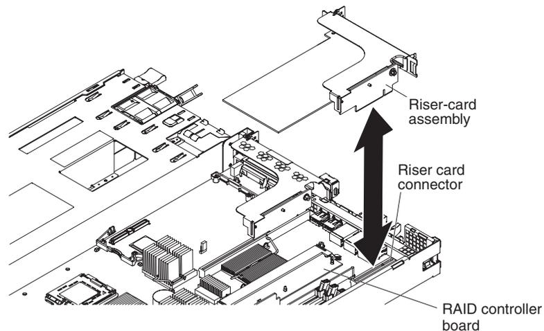
7. If an adapter was present in slot 1, reinstall it now (see “Installing an adapter” on page 103).
