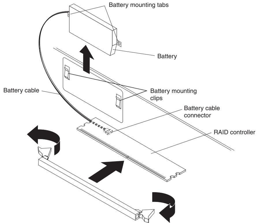
4. Do not disconnect the cable from the RAID controller battery (some models only) to the RAID controller board.
