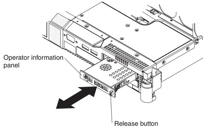
10. Press the release button on the front of the operator information panel and slide the assembly out of the server.
