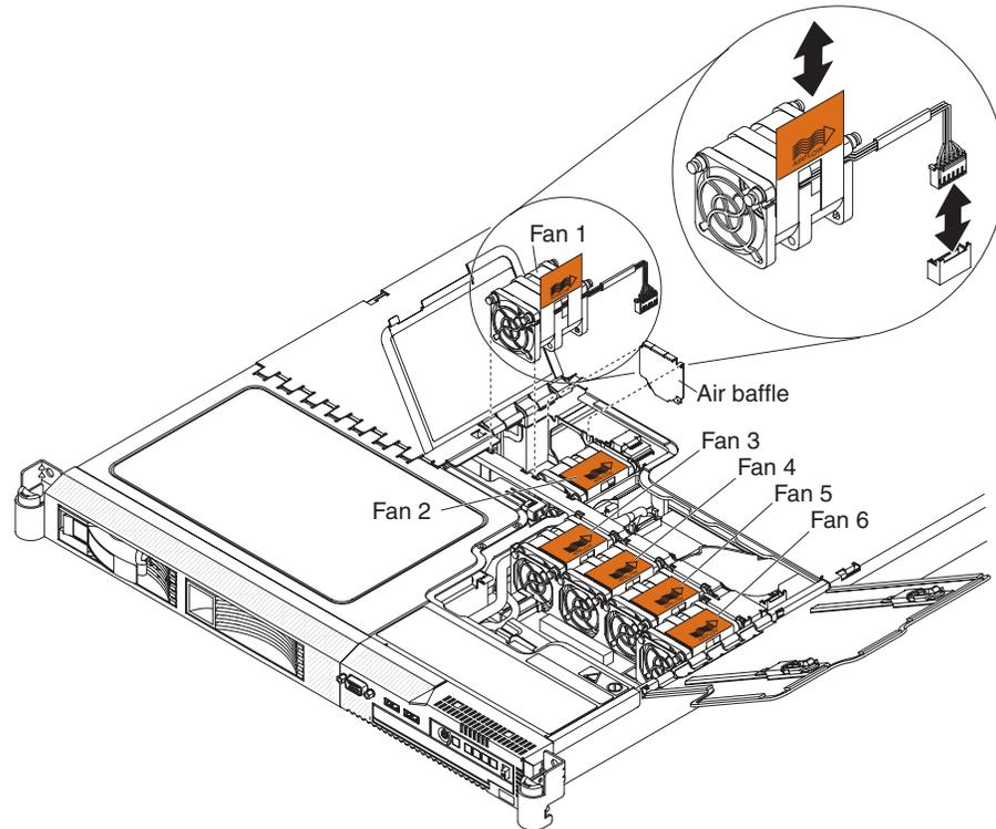
**Attention:** To ensure proper server operation, replace a failed fan within two minutes.
