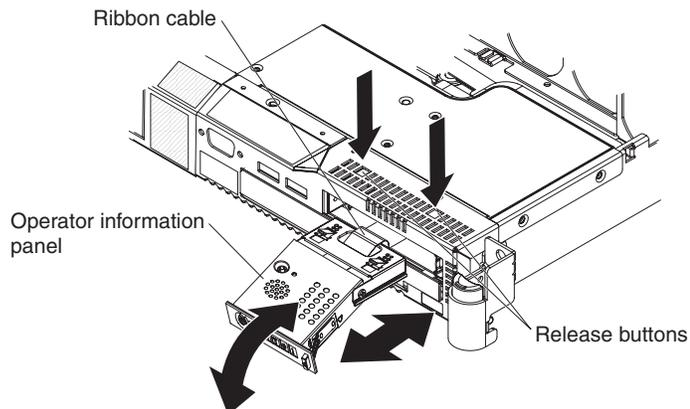
11. Press the release buttons on the top of the server and slide the operator information panel assembly rails out of the server as far as it will go.
