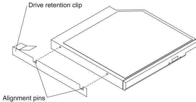
5. Slide the drive-retention clip to remove it from the drive.
