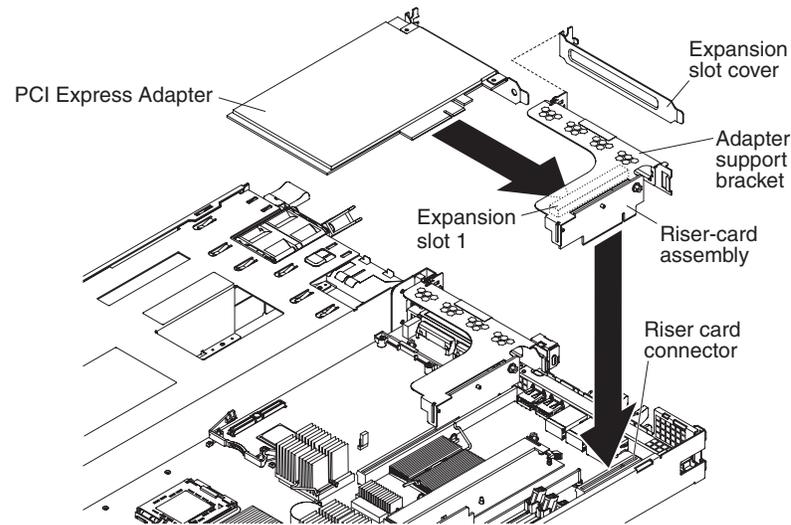
1. Remove the adapter from the static-protective package and set any jumpers or switches on the adapter as directed by the adapter manufacturer.
