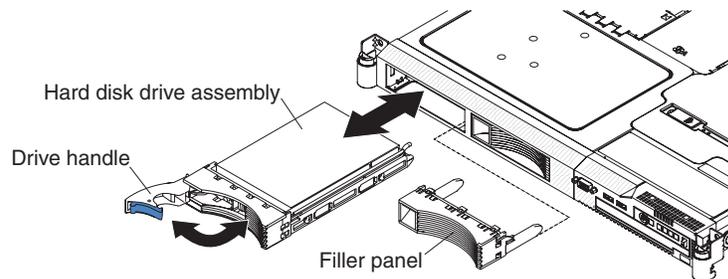
**Attention:** To avoid damage to the hard disk drive connectors, make sure that the server cover is in place and fully closed whenever you install or remove a hard disk drive.
