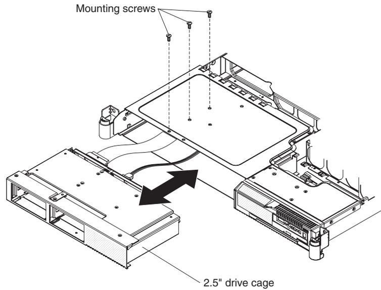
4. Remove the three drive cage mounting screws; then, slide the drive cage assembly forward out of the server.
