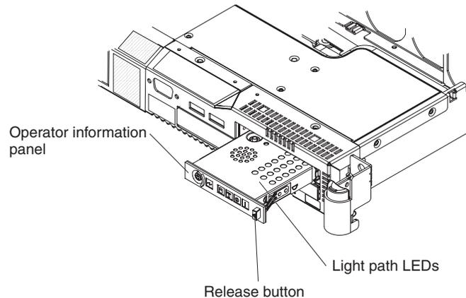
The following illustration shows the LEDs and controls on the light path diagnostics panel.
