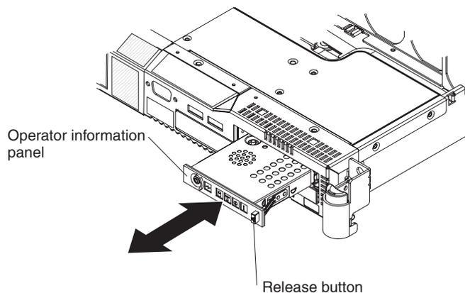
3. Slide the operator information panel into the server until it latches in place with a click.
