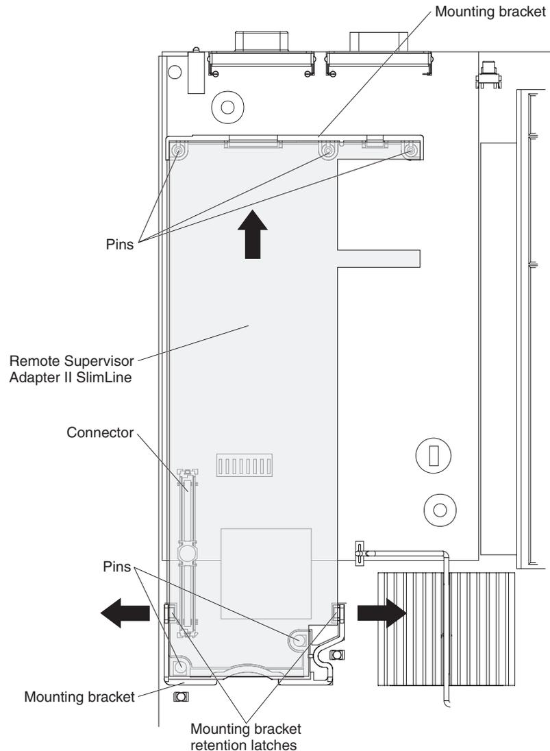
4. Spread the card retainers as you lift the Remote Supervisor Adapter II SlimLine card to disconnect it from the system board, then lift it out of the server.
