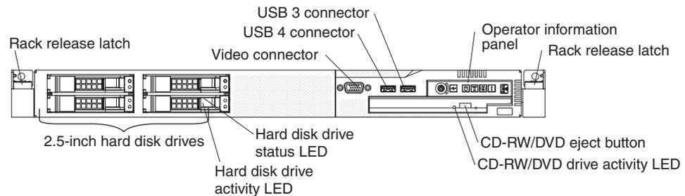
The following illustration shows the controls, LEDs, and connectors on the front of the server. This configuration supports up to two 3.5-inch hot-swappable hard disk drives or two 3.5-inch simple-swap SATA hard disk drives.
