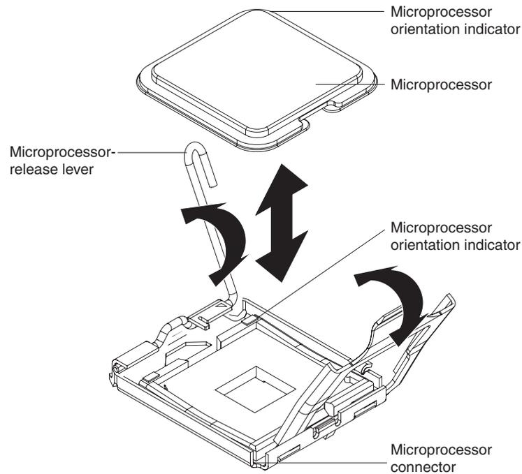
4. Open the microprocessor release lever to the fully-open position.
