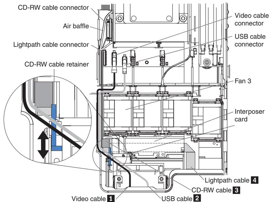
2. From the front of the server, thread the lightpath ribbon cable through the panel housing in the server; then, carefully route and connect the ribbon cable to the lightpath cable connector on the system board.
