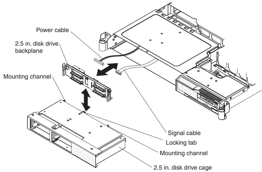
8. Press the locking tab and lift the backplane out of the server.
