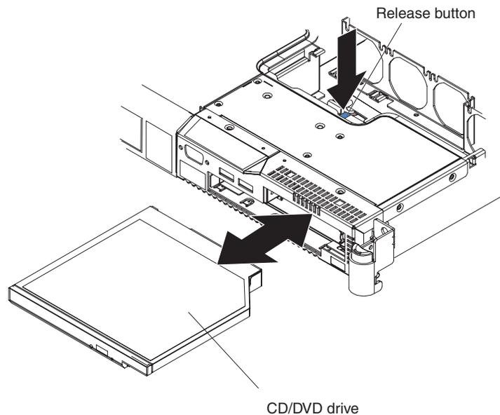
4. Press and hold the release button as you push the drive from the rear to slide it out of the bay.
