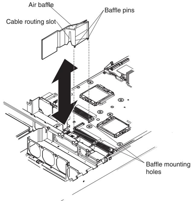
8. Remove the air baffle.
