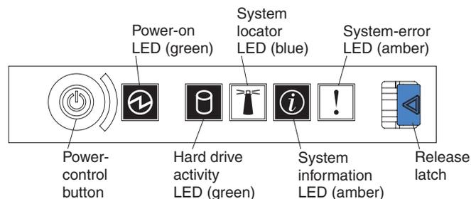
The following controls and LEDs are on the operator information panel:
