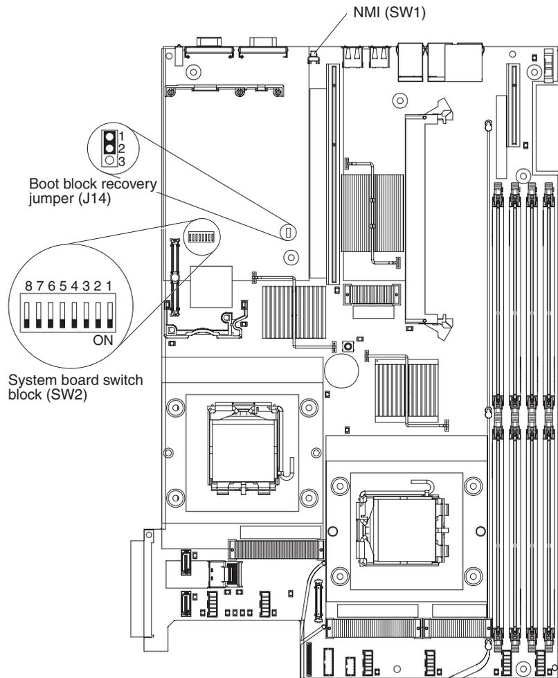
4. Move the jumper from pins 1 and 2 to pins 2 and 3 to enable the BIOS recovery mode.
