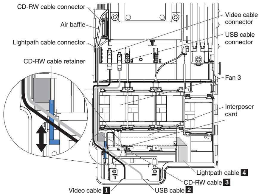
5. Slide the CD-RW cable retainer away from the interposer card.
