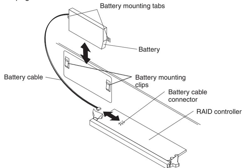
2. Insert the RAID controller battery in the server chassis.
