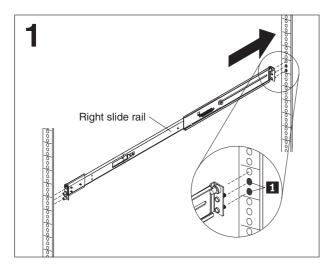
Insert the right slide rail into the rear rack mounting flange, with the rail pins 1 protruding through the flange.
