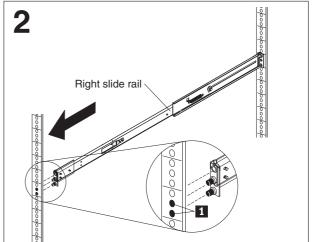
Extend the right slide rail and insert it into the front rack mounting flange, with the rail pins **1** protruding through the flange. Insert the left slide rail in the same way.
