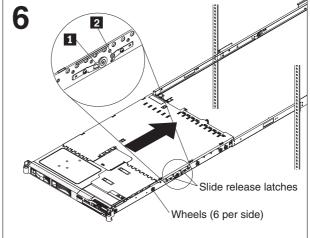
Attach the other slide rail and the cable-management-arm support bracket to the right rear mounting flange, using a single screw 1. The screw should be only finger tight.
