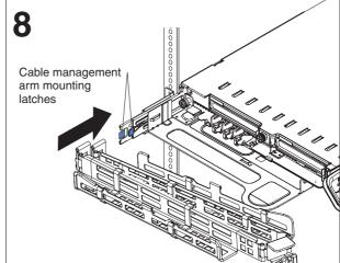
Align the cable-management-arm mounting plate with the rear of the server so that the four locking tabs on the mounting plate are aligned with the four tabs on the server. Slide the mounting plate to the left to engage the tabs; then, tighten the thumbscrew to secure the mounting plate to the server.
