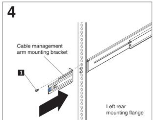
Attach the slide rail and the cable-management-arm mounting bracket to the left rear mounting flange with a single screw 1. The screw should be only finger tight.
