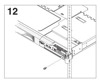
Before you transport the rack cabinet to another location with the server installed, you must secure the server to the rack with M6 screws at the front right and front left of the rack cabinet.
