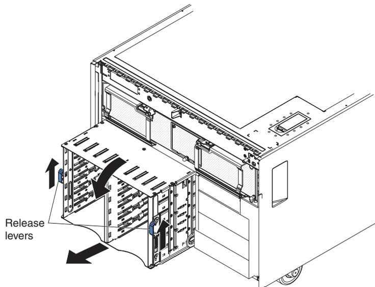
5. Lift the release levers on each side of the SAS cage and pull it out of the server until it stops.
