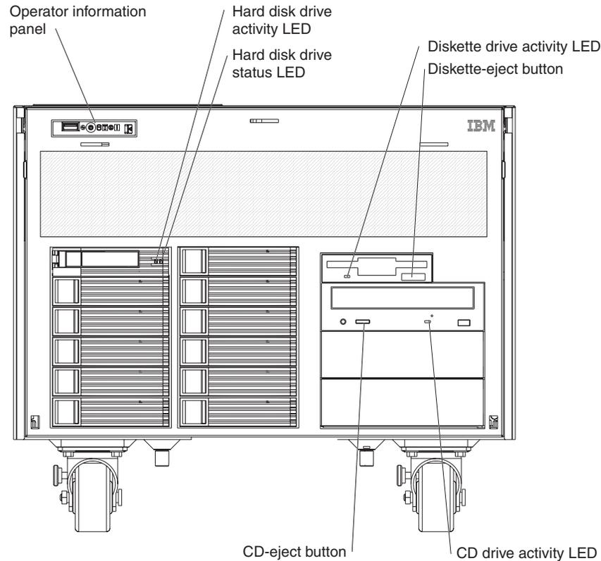
**Operator information panel:** This panel contains controls and LEDs. The following illustration shows the controls and LEDs on the operator information panel.
