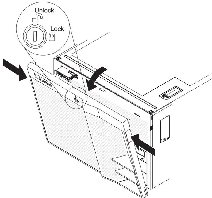
3. (Tower model only) Unlock the front cover and grasp the top corners of the front cover and pull it away from the server.
