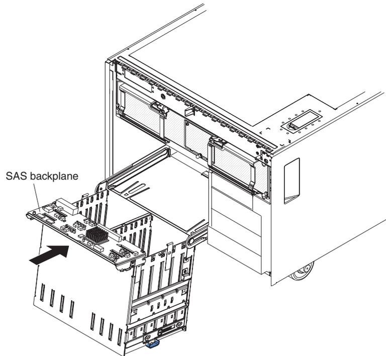
2. Slide the backplane into the card guides on the rear of the SAS hard disk drive cage and press the backplane into place.
