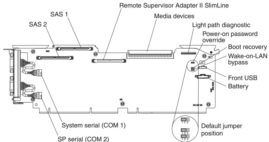
While the server is turned off, move the power-on password jumper from pins 1 and 2 to pins 2 and 3. You can then start the Configuration/Setup Utility program and reset the power-on password. After you reset the password, turn off the server again and move the jumper back to pins 1 and 2.
