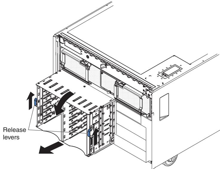
5. Lift the release levers on each side of the SAS hard disk drive cage and pull it out of the server until it stops.
