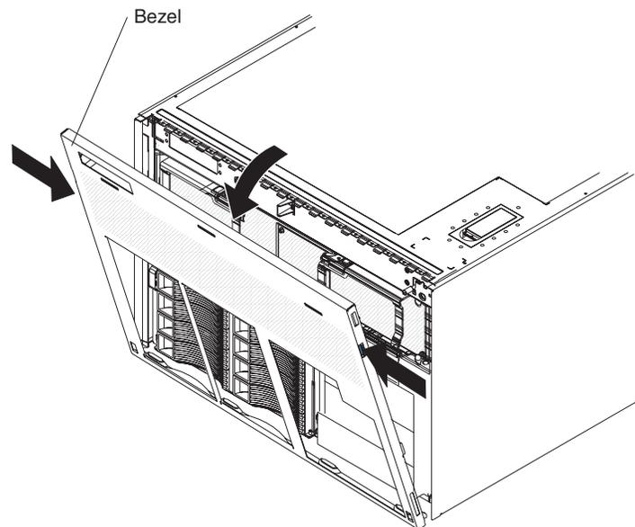
6. Press on the bezel retention tabs on both sides of the bezel, and pull the top of the bezel slightly away from the server.
