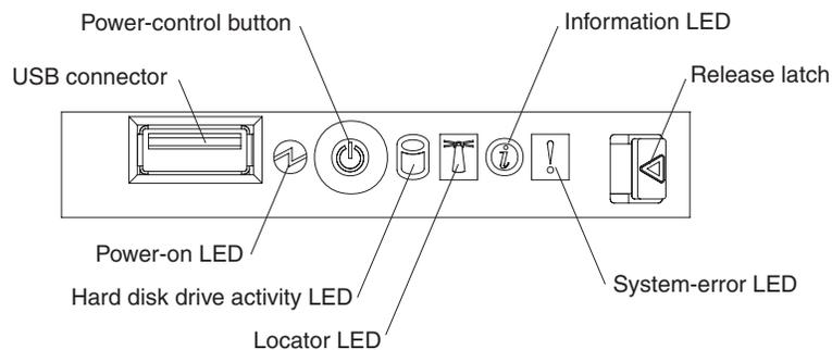
2. To view the light path diagnostics panel, press the release latch on the front of the operator information panel to the left; then, slide it forward. This reveals the light path diagnostics panel. Lit LEDs on this panel indicate the type of error that has occurred.
