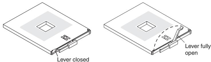
**Attention:** To avoid bending the pins on the microprocessor, do not use excessive force when pressing it into the socket.
