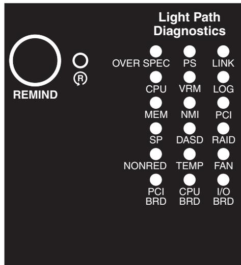
Look at the system service label on the top of the server, which gives an overview of internal components that correspond to the LEDs on the light path diagnostics panel. This information and the information in “Light path diagnostic LEDs” on page 64 can often provide enough information to correct the error.
