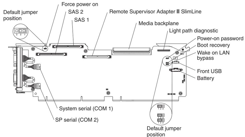
The following table describes the function of each three-pin jumper block.
