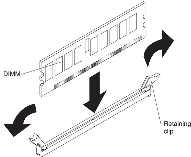
4. Insert the DIMM into the connector by aligning the edges of the DIMM with the slots at the ends of the DIMM connector. Firmly press the DIMM straight down into the connector by applying pressure on both ends of the DIMM simultaneously. The retaining clips snap into the locked position when the DIMM is seated in the connector. If there is a gap between the DIMM and the retaining clips, the DIMM has not been correctly inserted; open the retaining clips, remove the DIMM, and then reinsert it.
