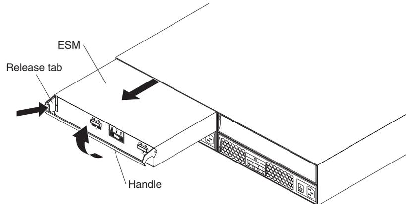
5. Using the handle, gently slide the ESM out of the EXP3000.
