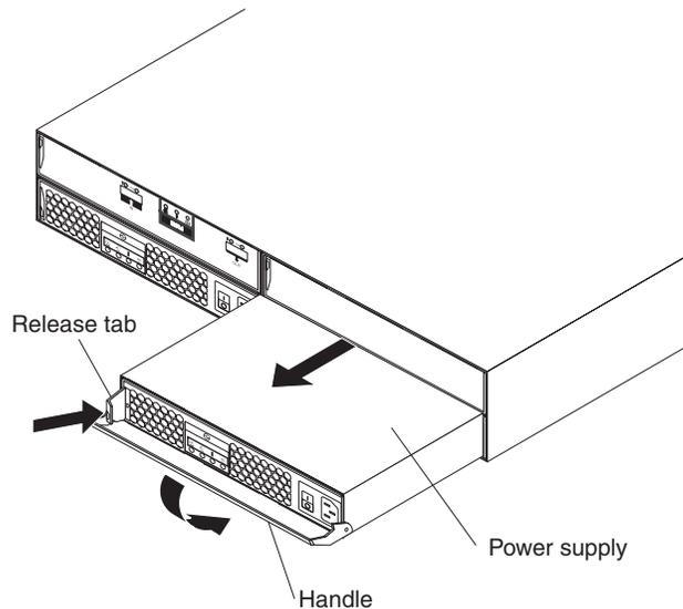
6. Using the handle, gently slide the power supply out of the EXP3000.
