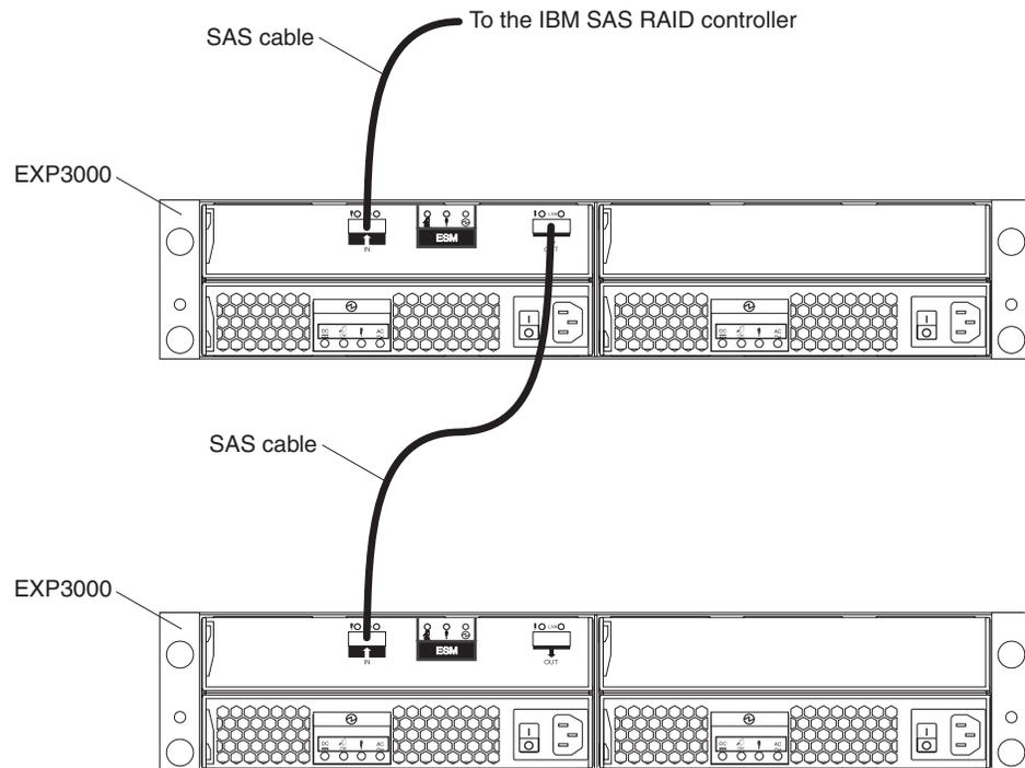
2. If your RAID controller supports connecting multiple EXP3000s, connect a second EXP3000 to the first EXP3000:
