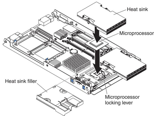
To install an additional microprocessor, complete the following steps:
