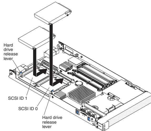
**Note:** Do not install a SCSI hard disk drive in SCSI connector 1 (SCSI ID 1) if you intend to also install an optional standard-form-factor expansion card. The standard-form-factor expansion card occupies the same area as the second hard disk drive.
