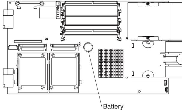
6. To remove the battery, use your finger to press down on one side of the battery; then, slide the battery out from its socket. The spring mechanism will push the battery out toward you as you slide it from the socket.
