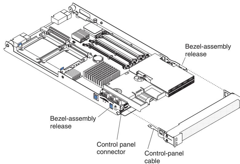
To remove the blade server bezel assembly, complete the following steps:
