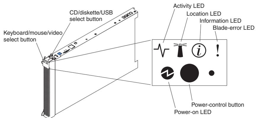
**Keyboard/mouse/video (KVM) select button:** Press this button to associate the shared BladeCenter unit keyboard port, mouse port, and video port with the blade server. The LED on this button flashes while the request is being processed then is lit when the ownership of the keyboard, mouse, and video has been transferred to the blade server. It can take approximately 20 seconds to switch the keyboard, video, and mouse control to the blade server.
