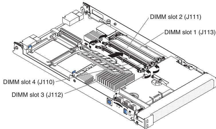
6. Locate the DIMM connectors on the system board (see the above illustration). Determine the connectors into which you will install the DIMMs.
