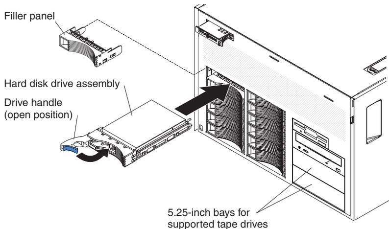
The server supports up to two 5.25-inch, half-high, SCSI tape drives in the 5.25-inch bays. A SCSI adapter is required to support the tape drives.
