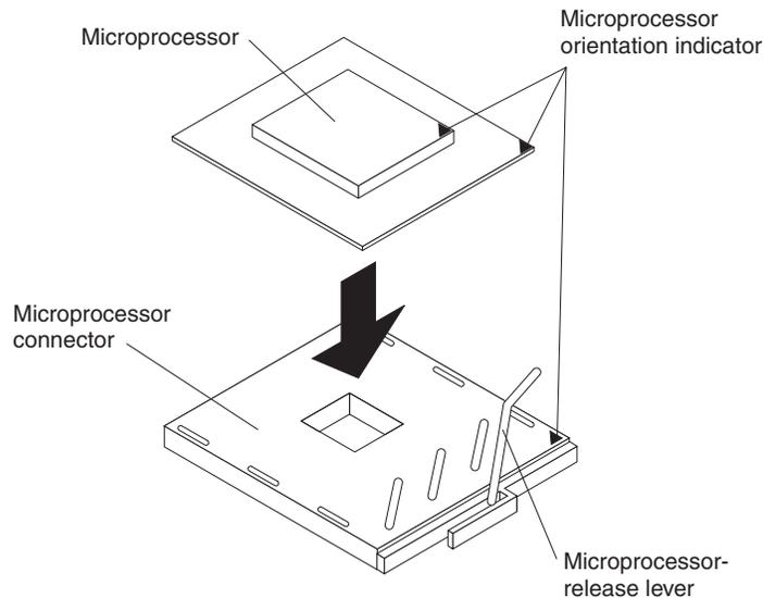
15. Close the microprocessor-release lever to secure the microprocessor.
