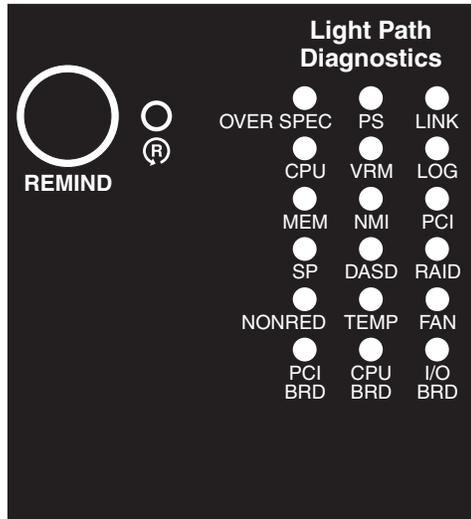
Look at the system service label on the top of the server, which gives an overview of internal components that correspond to the LEDs on the light path diagnostics panel. This information and the information in “Light path diagnostics panel” can often provide enough information to correct the error.
