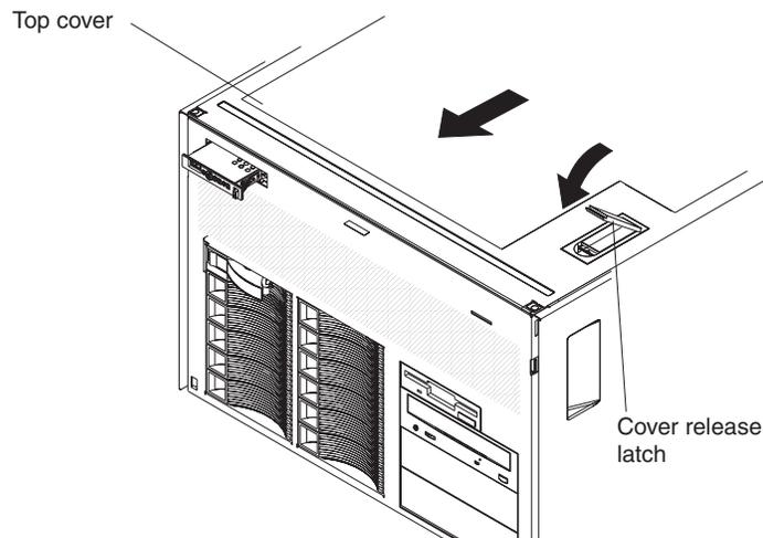
2. Move the cover-release latch to the open (up) position.
