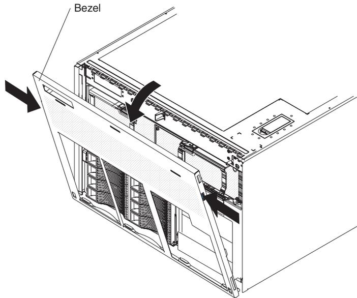
1. Press on the two release latches at the top edge of the bezel, and pull the top of the bezel slightly away from the server.
