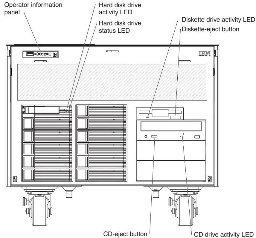
**Operator information panel:** The following illustration shows the controls and LEDs on the operator information panel.
