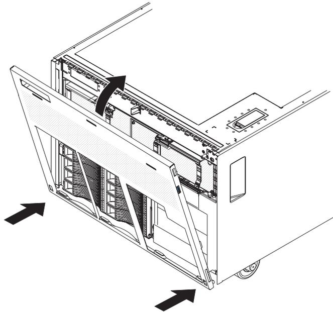
1. Insert the two tabs on the bottom of the bezel into the matching holes on the server chassis.
