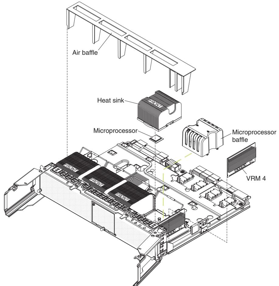
9. Remove the microprocessor baffle from a microprocessor socket and store it for future use. If you remove a microprocessor you must install a microprocessor baffle to prevent the server from overheating.
