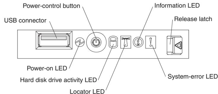
The following controls, connectors, and LEDs are on the operator information panel:
