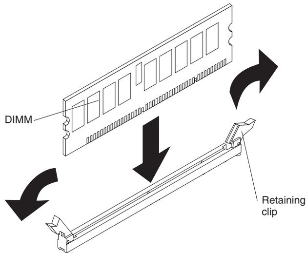
9. Insert the DIMM into the connector by aligning the edges of the DIMM with the slots at the ends of the DIMM connector. Firmly press the DIMM straight down into the connector by applying pressure on both ends of the DIMM simultaneously. The retaining clips snap into the locked position when the DIMM is seated in the connector. If there is a gap between the DIMM and the retaining clips, the DIMM has not been correctly inserted; open the retaining clips, remove the DIMM, and then reinsert it.
