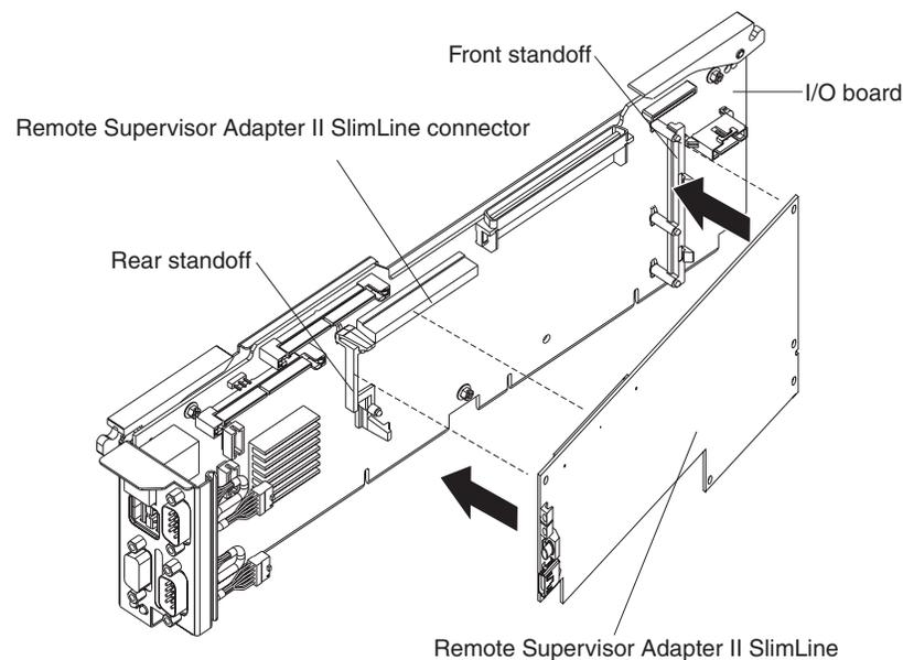
Complete the following steps to install a Remote Supervisor Adapter II SlimLine:
