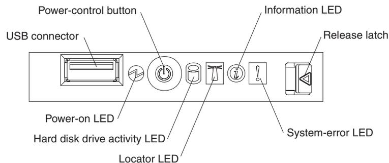
2. Unlock the front cover (tower model only) and remove the server cover to look inside the server for lit LEDs. Certain components inside the server have LEDs that will be lit to indicate the location of a problem. For example, a VRM error will light the LED next to the failing VRM on the microprocessor tray.
