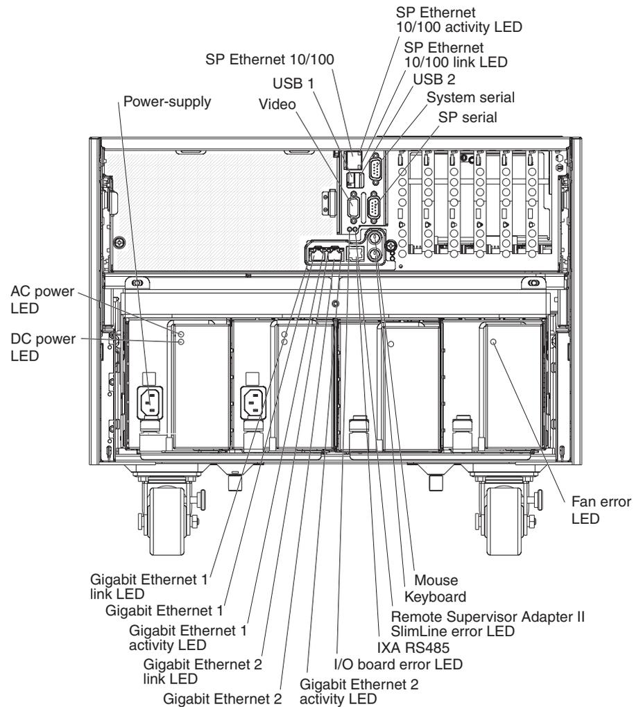
**Power-supply connector:** Connect the power cord to this connector.
