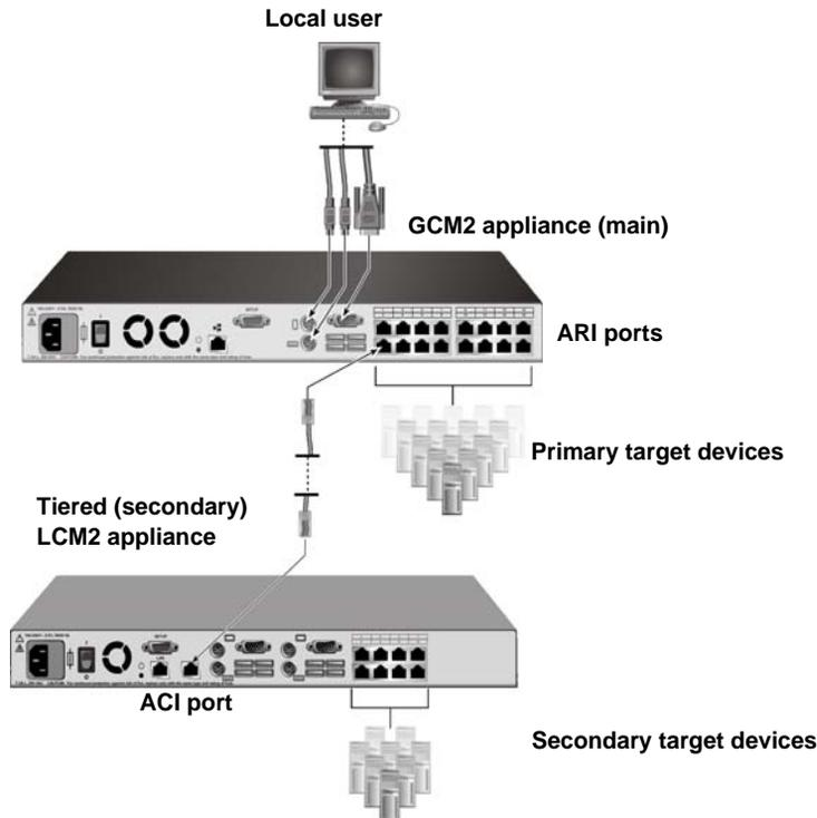
**Figure 2.4: Appliance configuration with a tiered appliance**
