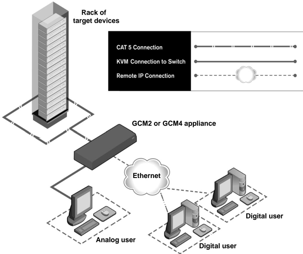
Figure 1.3: Example appliance configuration
