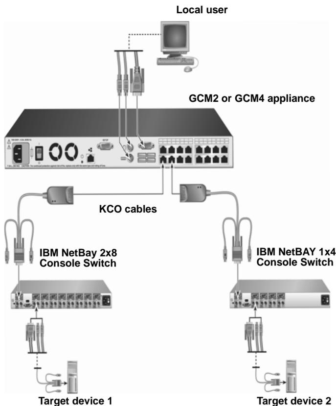
**Figure 2.5: Appliance configuration with an earlier-model appliance**
