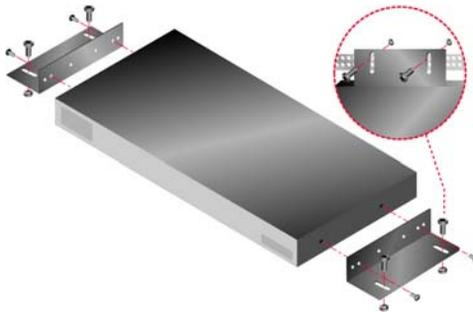
Figure 2.2: Appliance vertical installation
