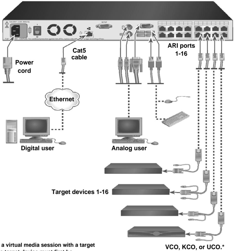
Figure 2.1: Basic appliance configuration
