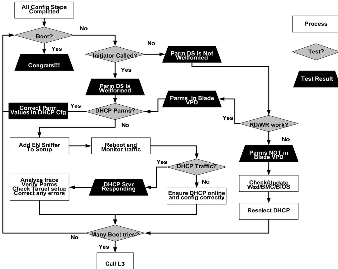
Figure 27: Error Tree for In Band iSCSI Deployment
