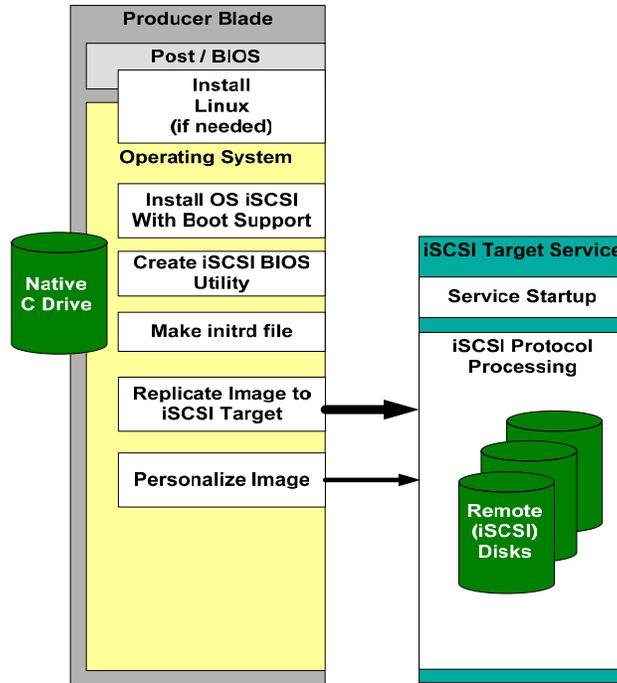
Figure 7: Disk Image Creation and Deployment
