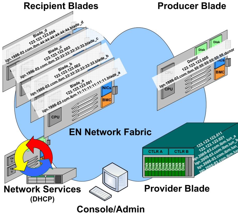
Figure 11: iSCSI Example Solution Enumerated
