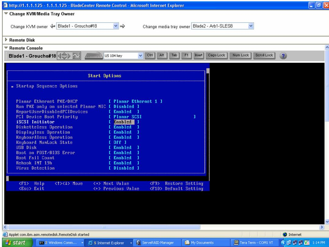
Figure 24: F1/BIOS Panel for Enabling iSCSI boot
