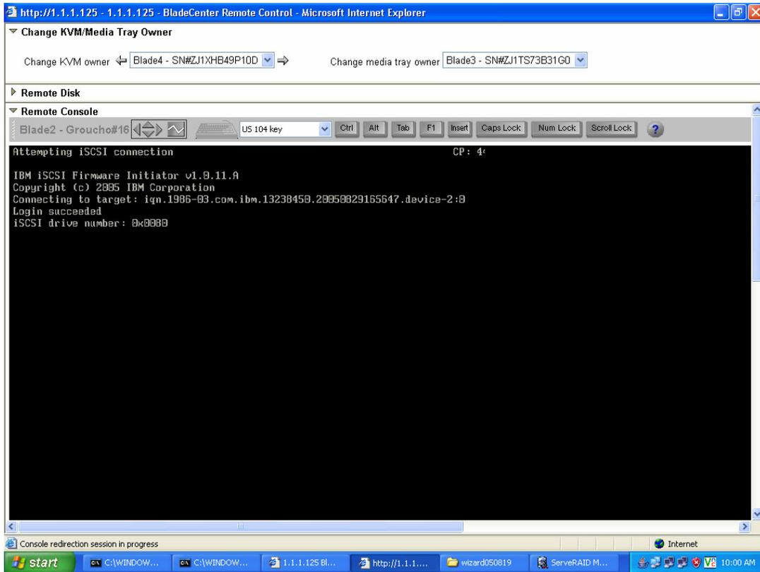
**Figure 25: BIOS Panel of a Successful iSCSI Login to an iSCSI Target**
