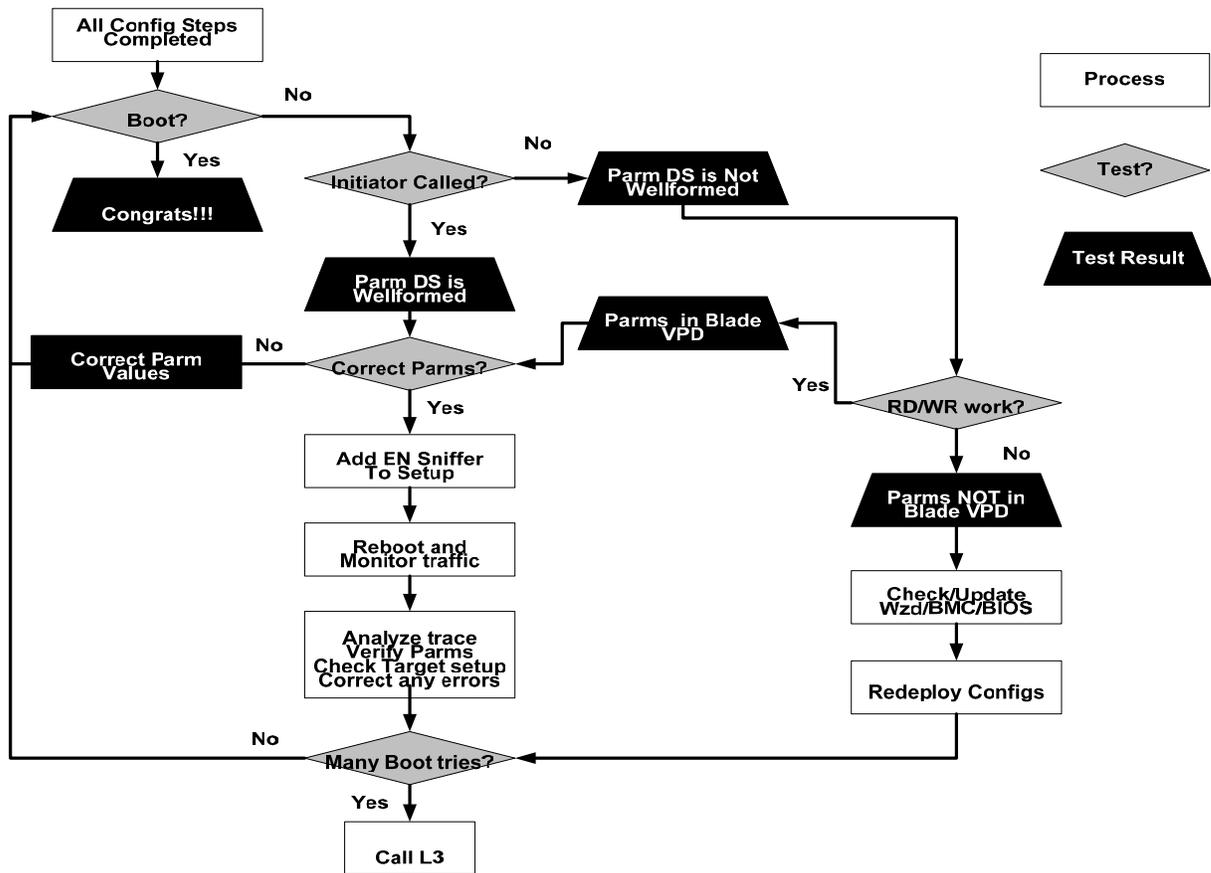
Figure 28: Error Tree for iSCSI Out of Band Deployment
