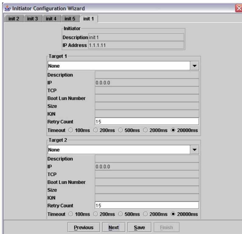
Figure 23: iSCSI Initiator to iSCSI Target Mapping Panel
