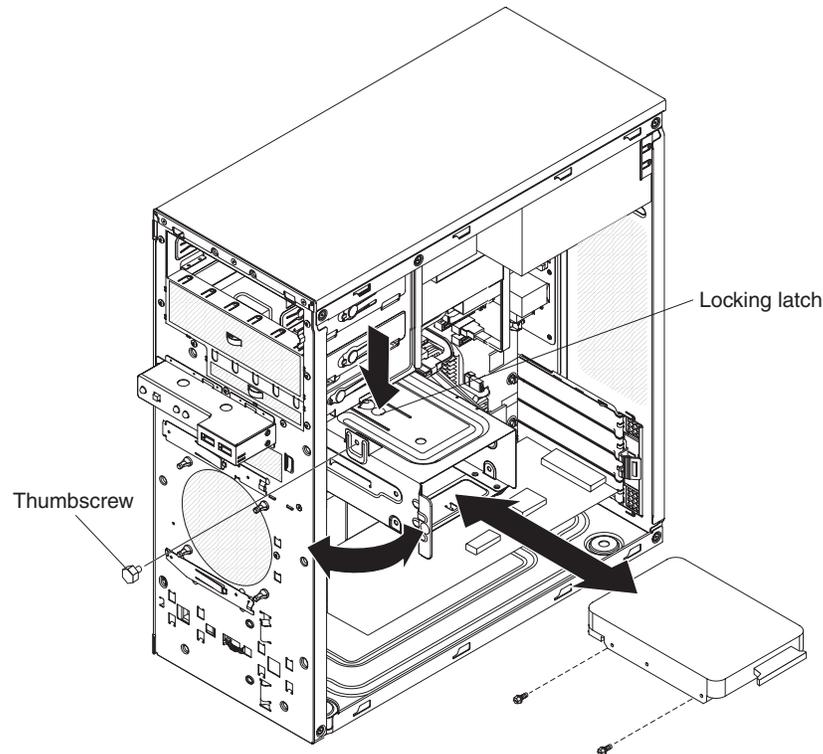
6. Touch the static-protective package that contains the drive to any unpainted metal surface on the server; then, remove the drive from the package and place it on a static-protective surface.
