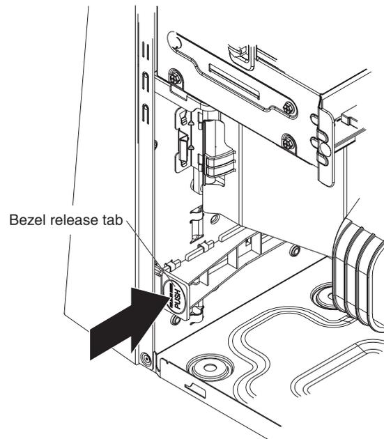
5. Press down slightly on the bezel release tab and pull the bottom of the bezel away from the chassis; then, lift the bezel to disengage the top tabs.
