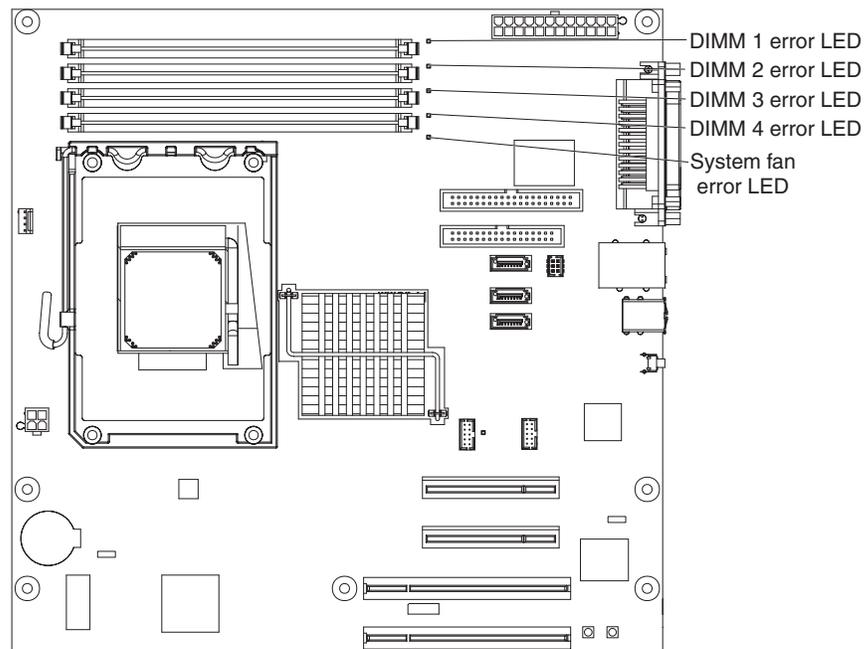
Each error LED is lit to indicate a problem with a specific component. After a problem is corrected, its LED will not be lit the next time the server is restarted; if the problem remains, the LED will be lit again. See the *Problem Determination and Service Guide* on the IBM System x Documentation CD for additional information.
