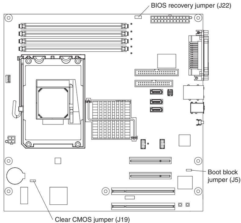
4. Move the boot block recovery jumper to pins 2 and 3.
