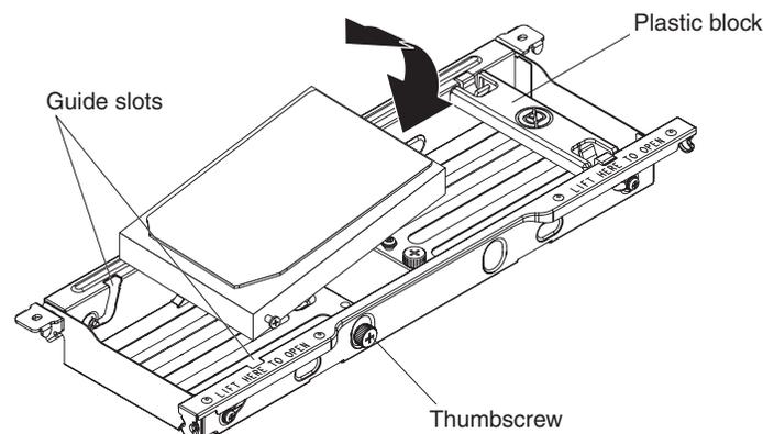
Figure 35. Removing a drive from bay 5
