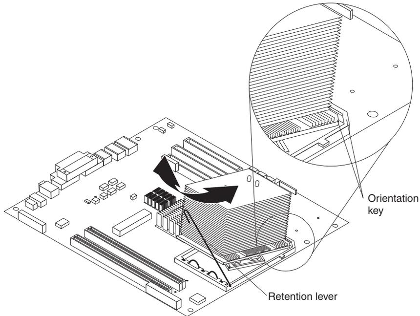
Figure 50. Installing the heat sink
