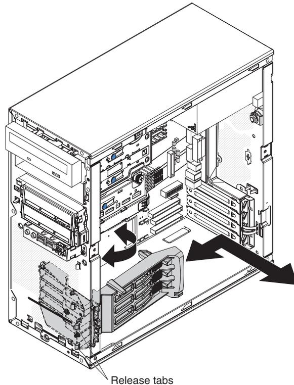
Figure 13. Removing the front adapter-retention bracket
