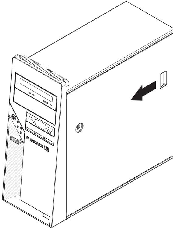
Figure 10. Installing the side cover
