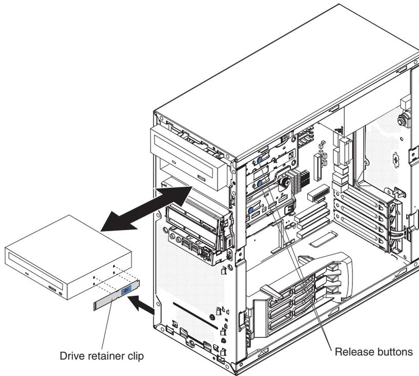
Figure 31. Removing a drive from bay 1 or 2
