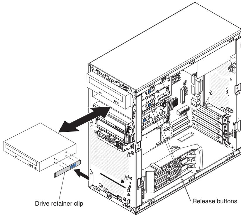
Figure 32. Installing a drive in bay 1 or 2
