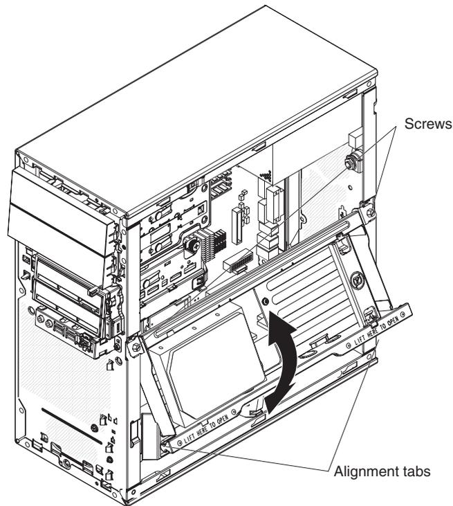
Figure 29. Installing the internal drive-bay bracket
