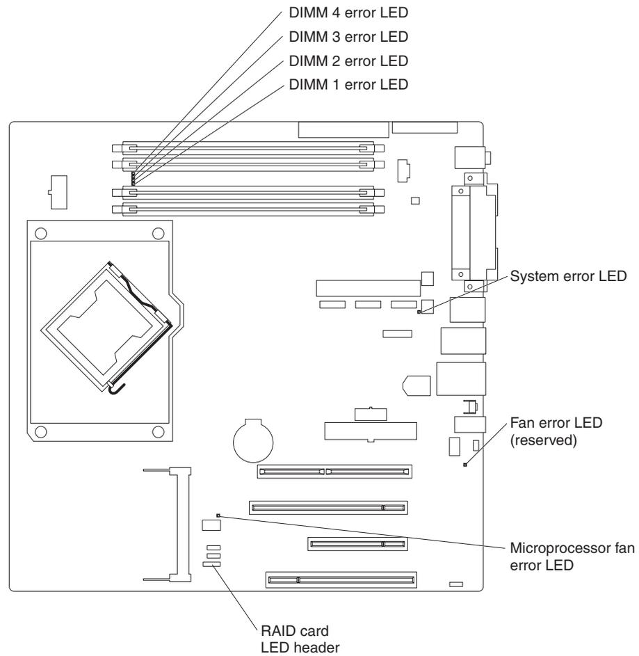
Figure 5. System-board LEDs
