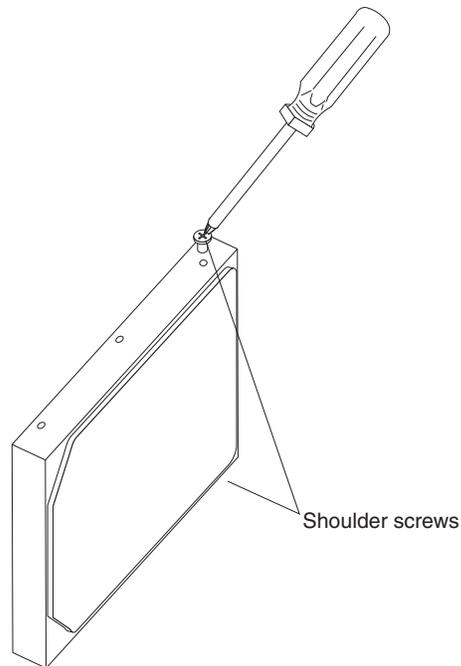
Figure 37. Hard disk drive shoulder screws
