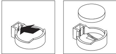
Figure 26. Removing the battery
