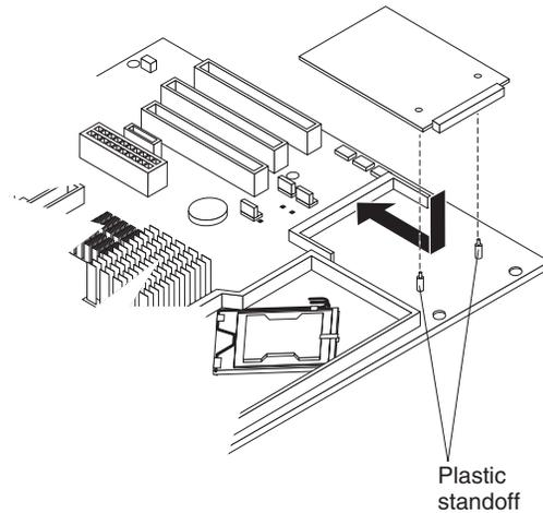
Figure 40. Installing the mini-SAS adapter
