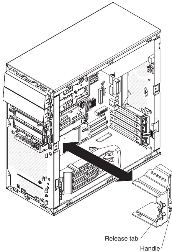
Figure 18. Installing the air baffle
