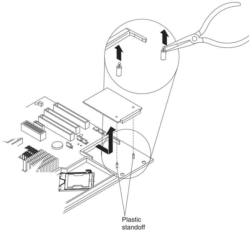
Figure 39. Removing the mini-SAS adapter
