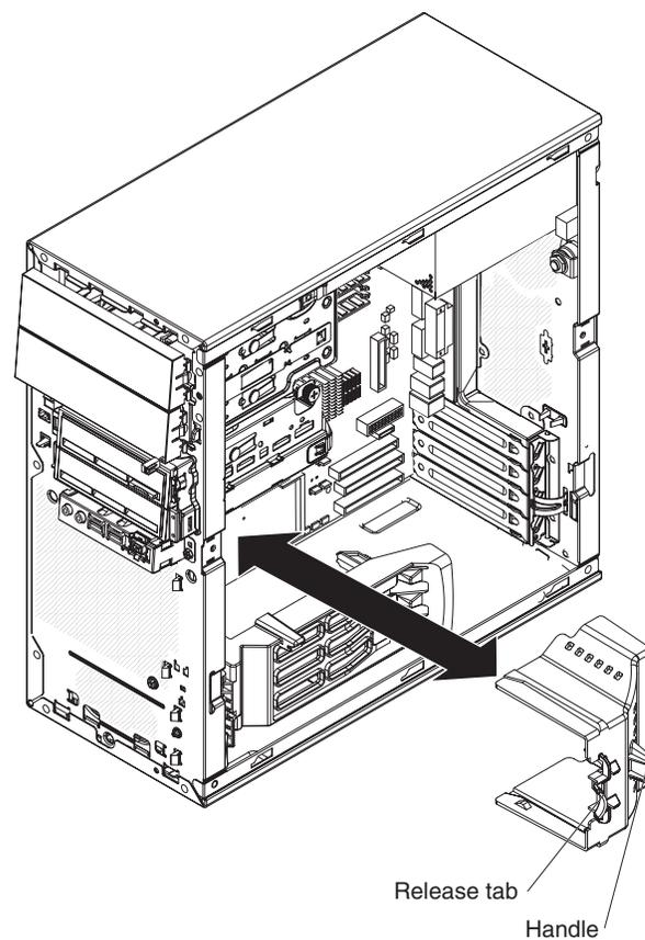
Figure 15. Removing the air baffle
