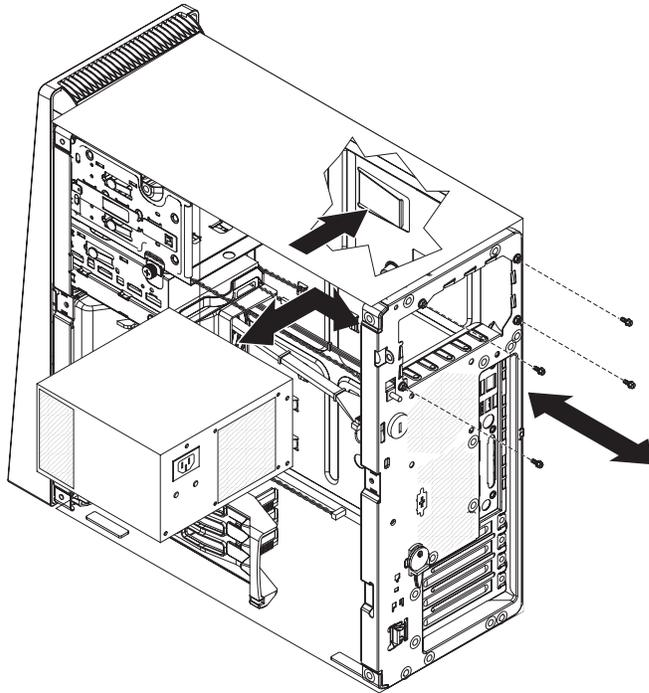
Figure 51. Removing the power supply
