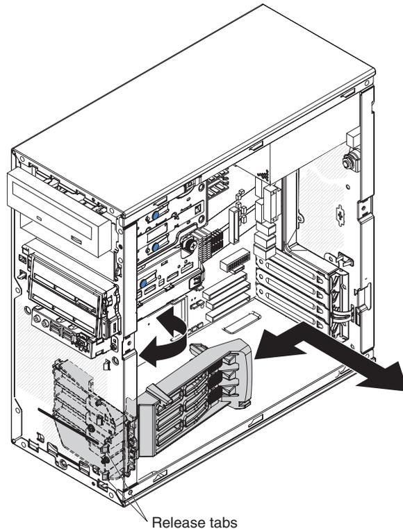
Figure 14. Installing the front adapter-retention bracket
