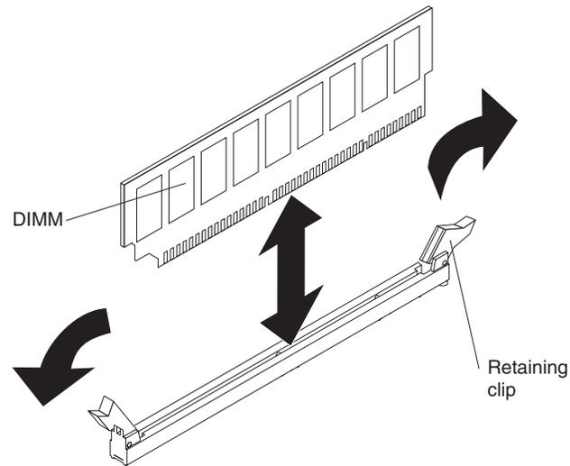
Figure 24. Installing a DIMM
