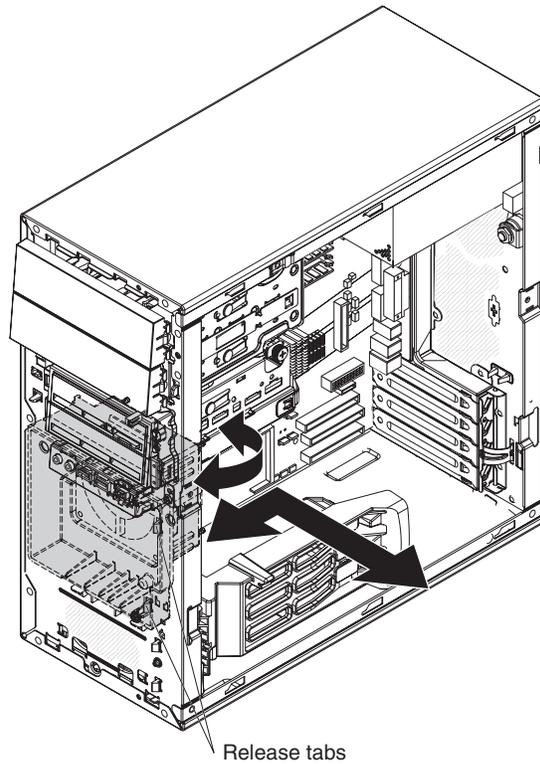
Figure 16. Removing the fan housing
