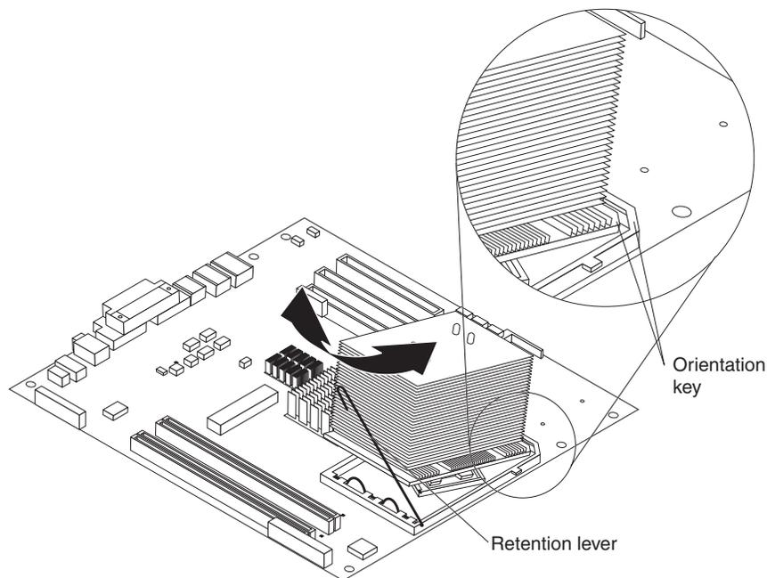
Figure 45. Removing the heat sink
