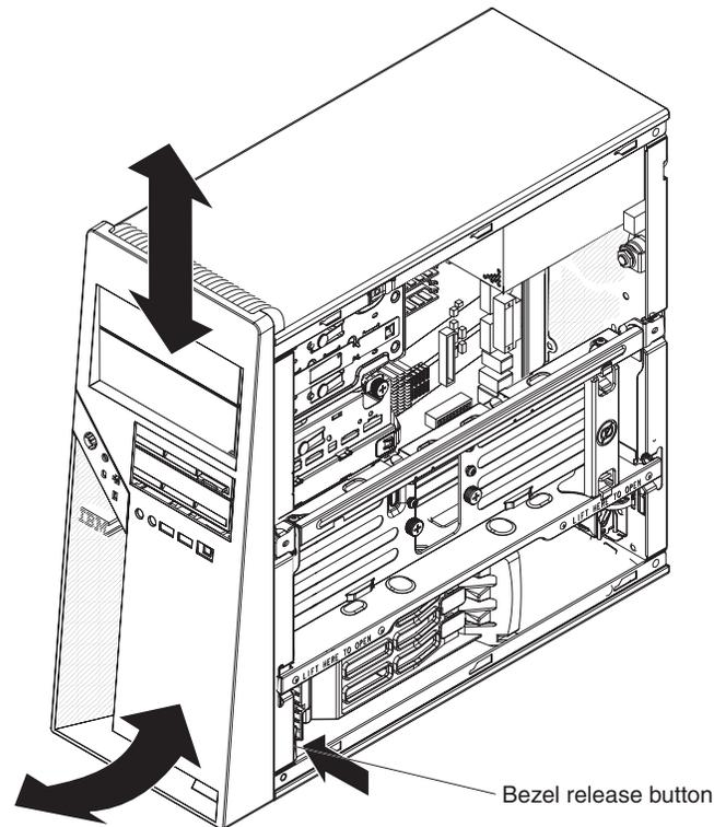
Figure 11. Removing the bezel
