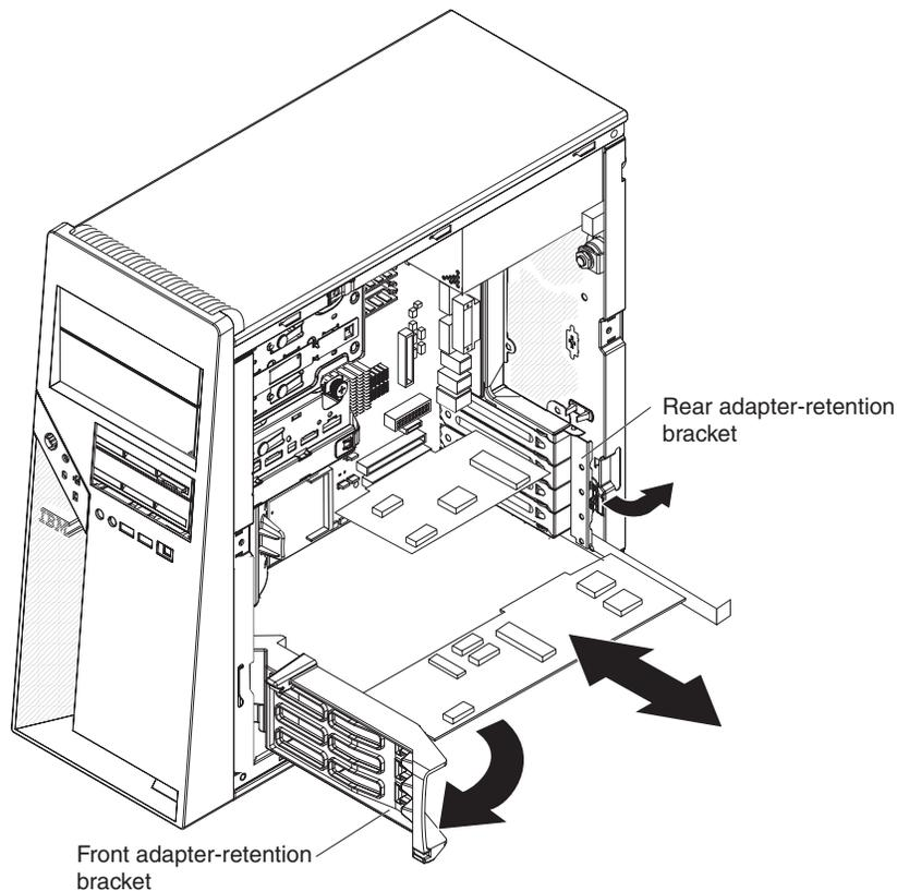
Figure 21. Installing an adapter
