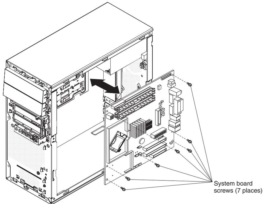
Figure 53. Removing the system board
