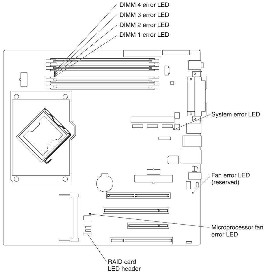
Figure 7. System-board error LED locations
