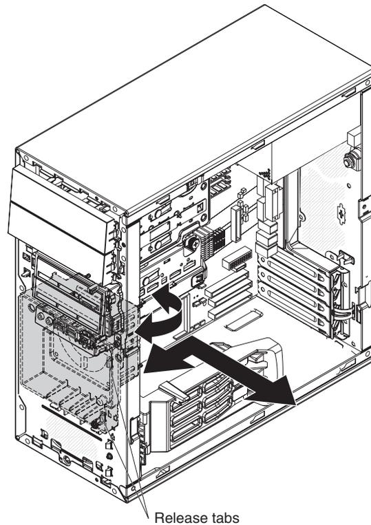
Figure 17. Installing the fan housing
