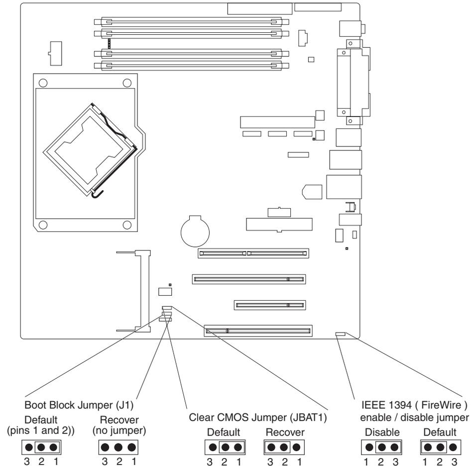
Figure 6. System-board jumpers
