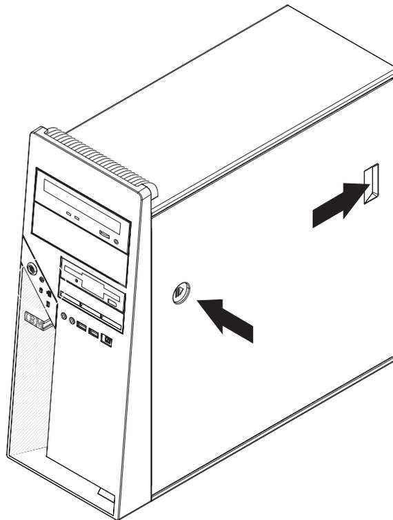
*Figure 9. Removing the side cover*
