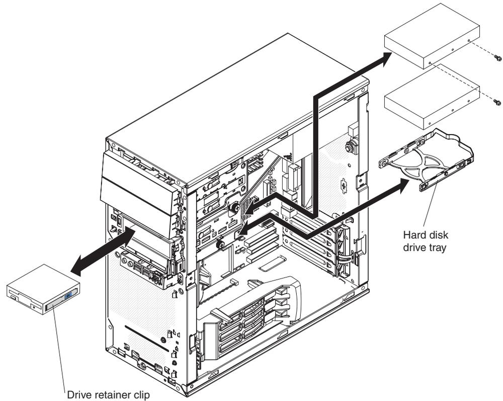
Figure 33. Removing a drive from bay 3 or 4
