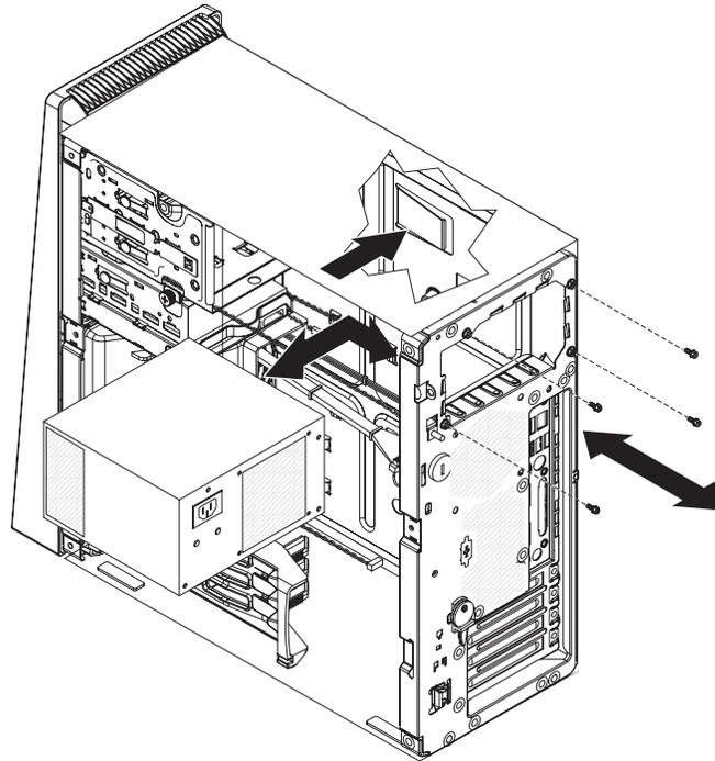
Figure 52. Installing the power supply
