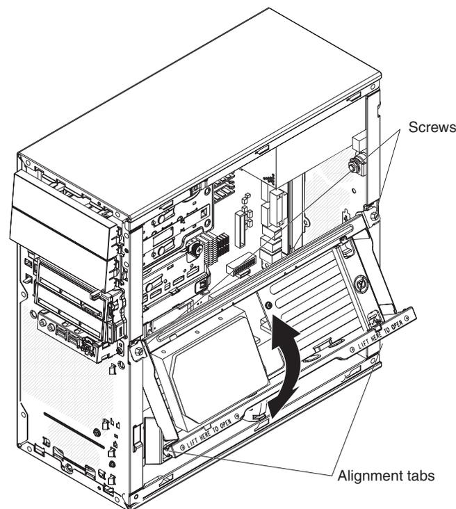
Figure 28. Removing the internal drive-bay bracket
