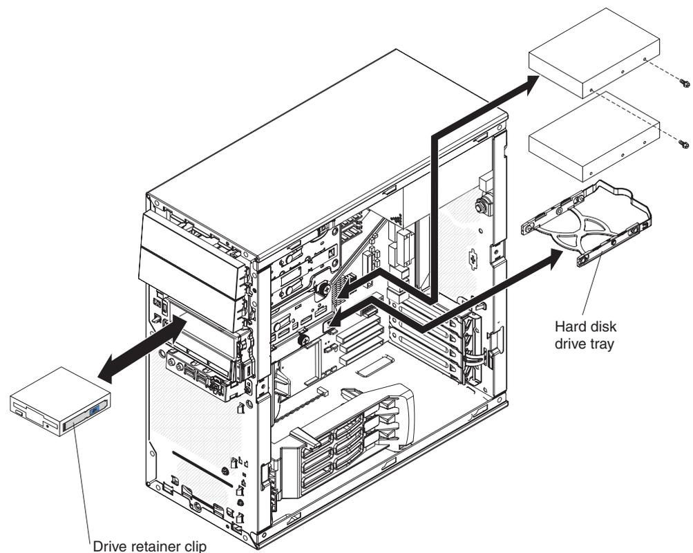
Figure 34. Installing a drive in bay 3 or 4
