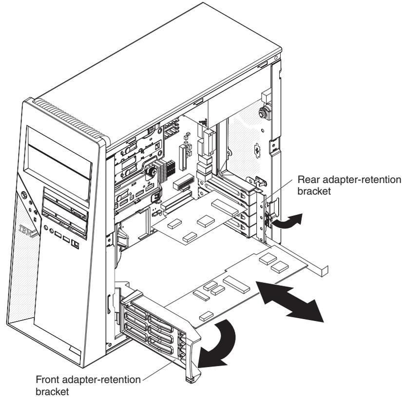
Figure 19. Removing an adapter
