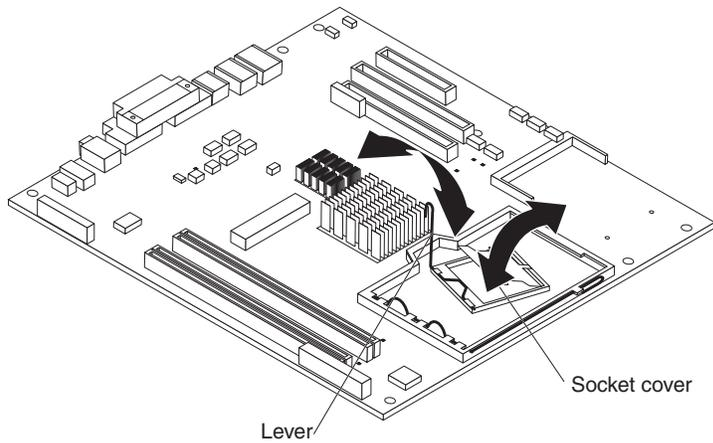
Figure 49. Closing the microprocessor socket
