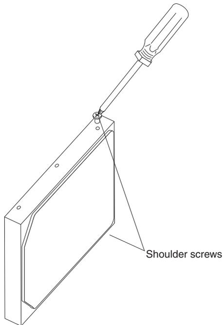
*Figure 36. Hard disk drive shoulder screws*
