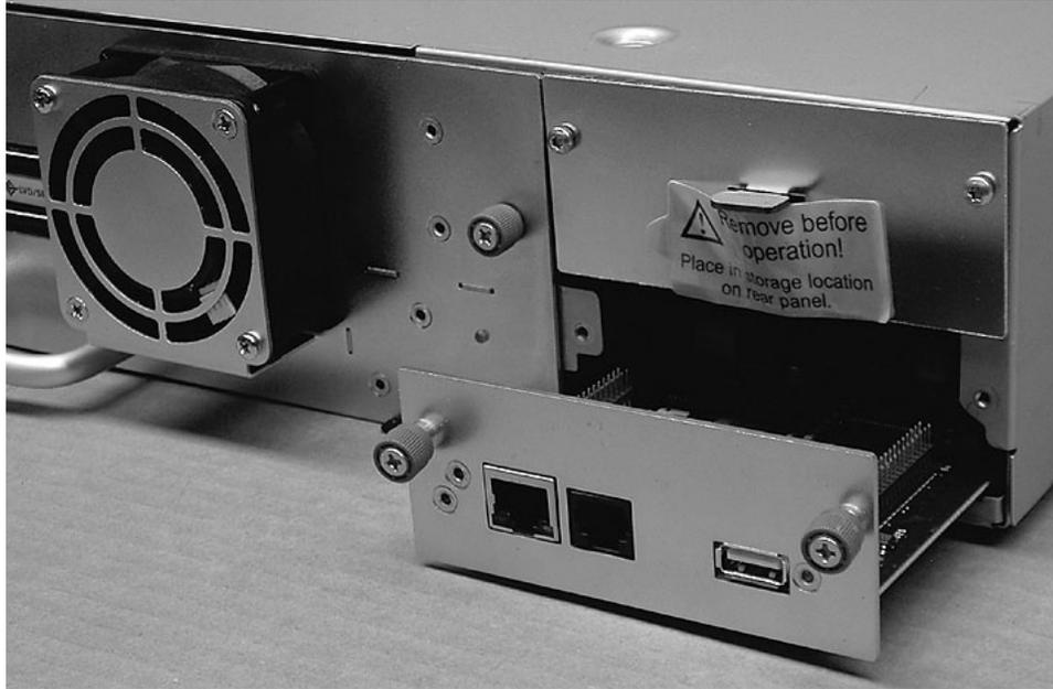
Figure 23. Remove controller card
