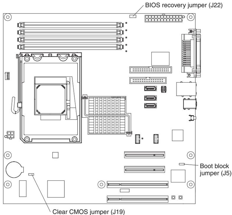
6. Move the clear CMOS recovery jumper from pins 2 and 3 to pins 1 and 2.
