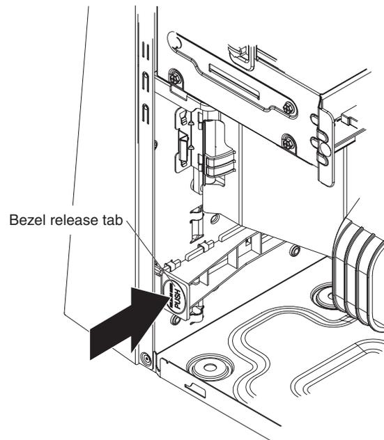
For instructions for replacing the bezel, see “Installing the bezel” on page 35.
