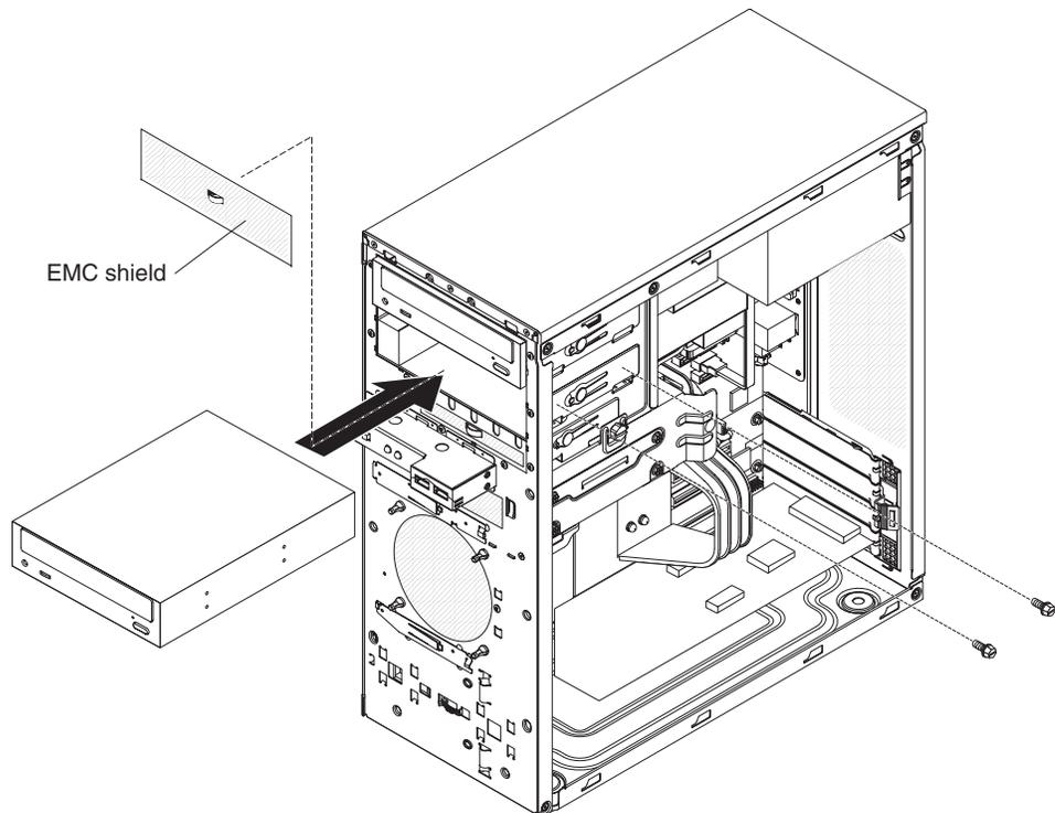
8. Secure the tape drive to the chassis with the supplied screws.
