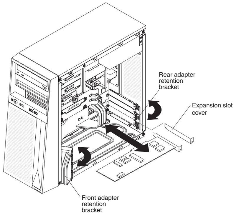
8. Reinstall the screw that you removed from the expansion slot earlier to secure the adapter to the chassis.
