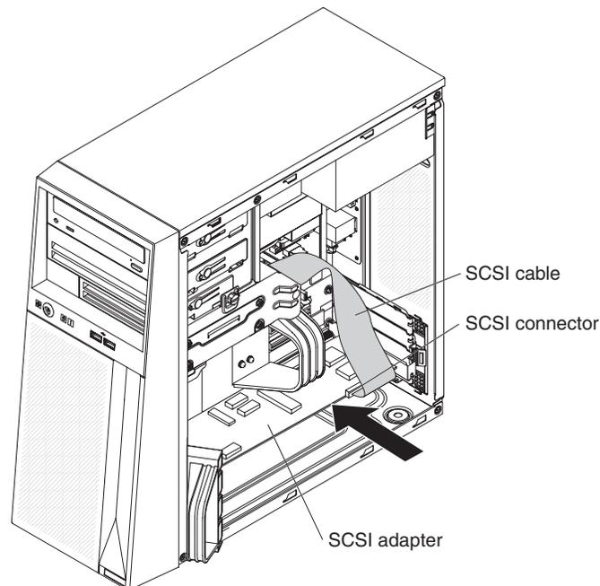
3. Complete the installation of the SCSI adapter (see “Installing an adapter” on page 32).
