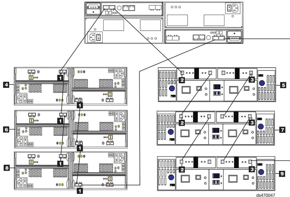
Figure 70. One DS4700 Express and two or more storage expansion enclosures in a mixed environment — Recommended cabling
