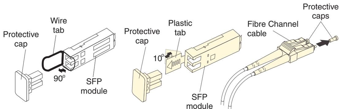
Figure 1. SFP modules and fibre channel cables
