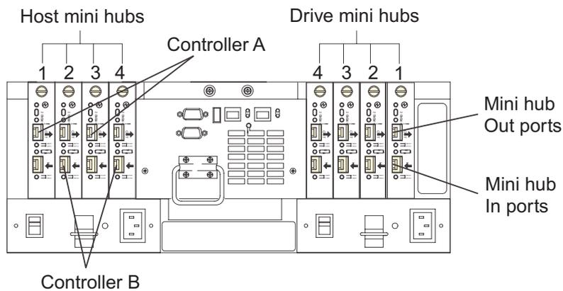
Figure 2. DS4500 Storage Subsystem ports and controllers
