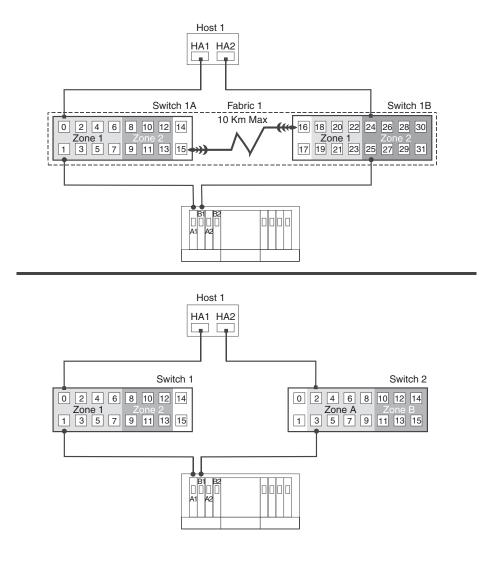
Figure 16. Switch zoning in cascaded (top) and noncascaded (bottom) Fibre Channel switches
