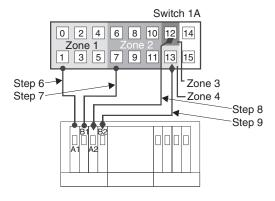
Figure 25. Storage subsystem connections to Fibre Channel switches
