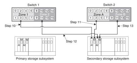
Figure 32. Secondary storage subsystem connections to Fibre Channel switches
