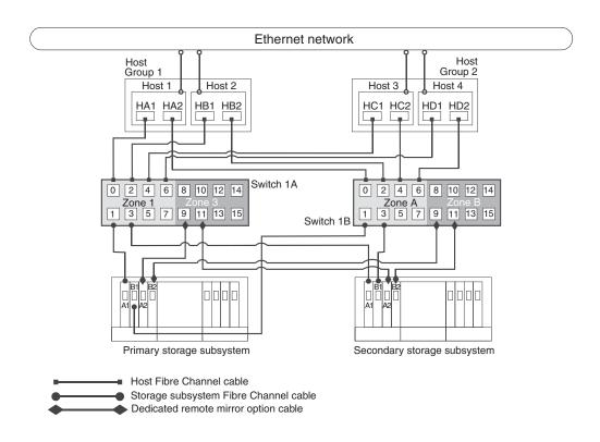
Figure 15. Intra-site configuration showing a two-switch connection
