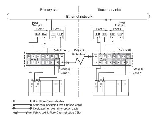
Figure 14. Dual-site, two-switch Campus configuration
