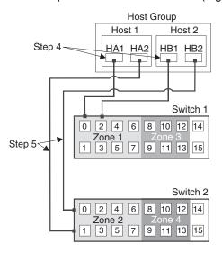
Figure 19. Host bus adapter connections to Fibre Channel switches
