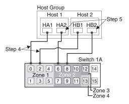
Figure 24. Host bus adapter connections to Fibre Channel switches
