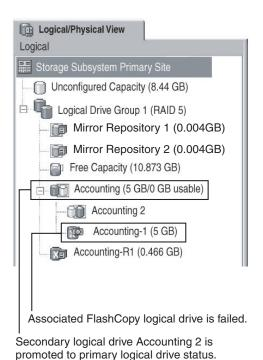
Figure 12. FlashCopy logical drive failure due to role reversal
