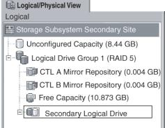
Both the primary and secondary logical drives are displayed in the Subsystem Management window for the storage subsystem.
