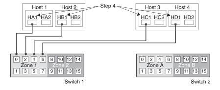
Figure 29. Primary host bus adapter (Hx1) connection to the Fibre Channel switches
