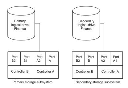
Figure 7. Controller A shown as the controller owner
