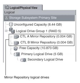
Figure 2. Mirror repository logical drives displayed in the Subsystem Management window
