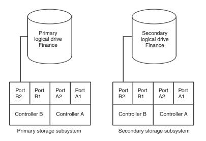
Figure 8. Controller B shown as controller owner
