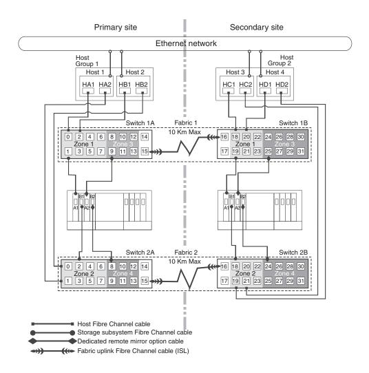
Figure 13. Dual-site, four-switch Highest Availability Campus configuration
