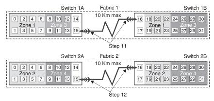
Figure 21. Connecting switches over a remote network to complete Fabric 1 and Fabric 2 environments
