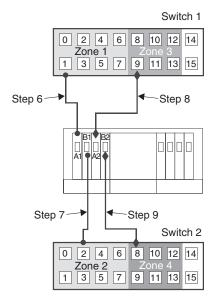
Figure 20. Storage subsystem connections to the Fibre Channel switches
