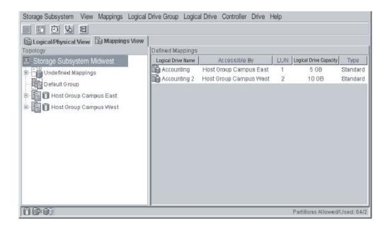
Figure 9. Mappings View of the Subsystem Management window showing storage partitioning
