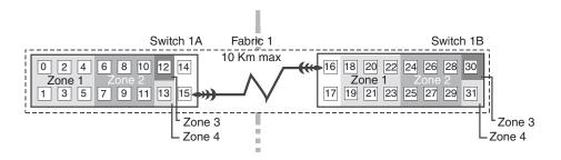
Figure 23. Switch zoning for the Campus configuration
