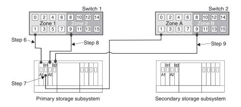
Figure 31. Primary storage subsystem connections to Fibre Channel switches
