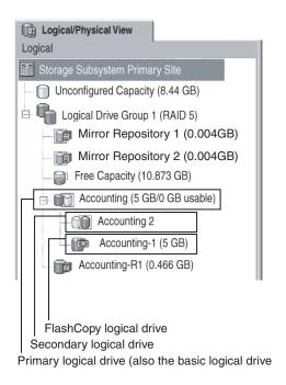
Figure 10. FlashCopy logical drive included in a mirror relationship
