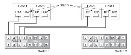
Figure 30. Secondary host bus adapter (Hx2) connection to the Fibre Channel switches
