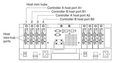
Figure 6. Controller A and Controller B host ports
