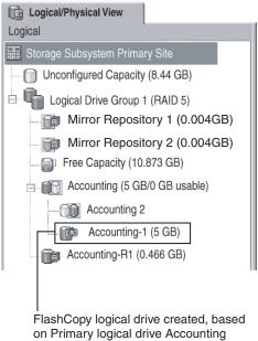
Figure 11. FlashCopy logical drive associated with primary logical drive Accounting
