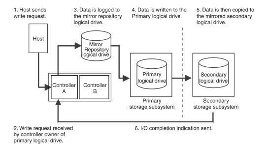
Figure 3. Data replication between primary and secondary storage subsystems
