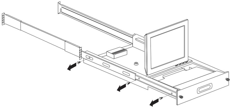
5. Remove all three screws that hold the old slide rail in place; then, attach the new slide rail using those same screws.
