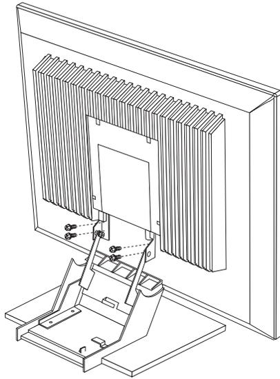
9. Remove the two screws that attach the lower cable cover to the bottom of the monitor; then, store the cable cover for possible future use.
