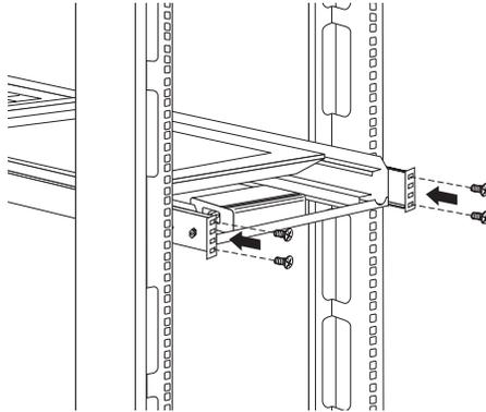
13. While one person pulls the tray halfway out of the front of the rack cabinet and supports the weight of the tray, attach the front of the tray to the rack cabinet using four of the screws from the miscellaneous hardware kit.
