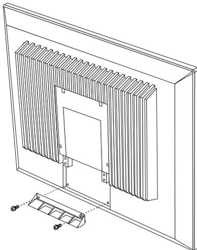
10. Connect the video and power connectors that you disconnected in step 4 on page 13 to the new monitor; then, attach the new monitor to the tray using the four screws that you removed earlier.
