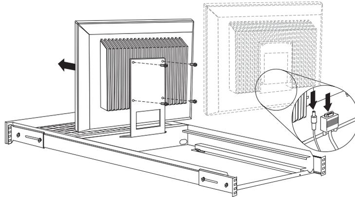
4. Disconnect the video and power connectors from the old monitor and set it aside.
