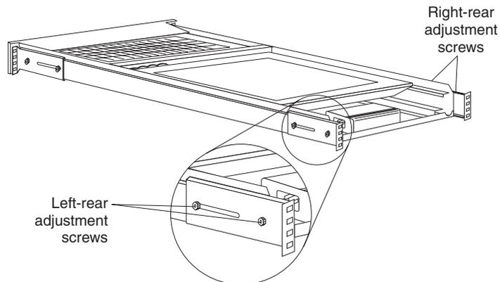
9. Tighten all four slide-rail adjustment screws.
