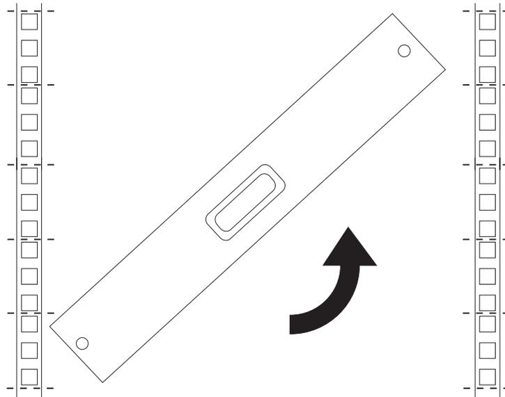
12. Attach the brackets to the rack cabinet using four screws from the miscellaneous hardware kit.
