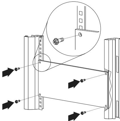
2. Attach the blank filler panel with M6 screws and cage nuts, or clip nuts depending on your rack cabinet.
