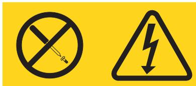
Hazardous voltage, current, and energy levels are present inside any component that has this label attached. There are no serviceable parts inside these components. If you suspect a problem with one of these parts, contact a service technician.
