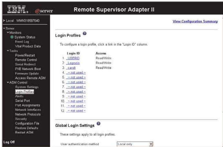
**Note:** By default, the Remote Supervisor Adapter II is configured with one login profile that enables remote access using a login user ID of USERID and a password of PASSWORD (the 0 is a zero not an O). To avoid a potential security exposure, change this default login profile during the initial setup of the Remote Supervisor Adapter II.
