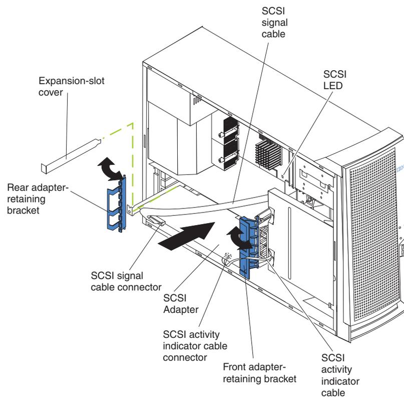
4. Complete the installation of the optional SCSI adapter.
