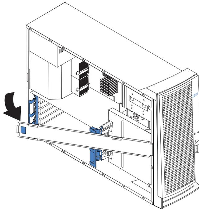
4. If your server comes with a support bracket that has a fan and a fan bracket attachment that looks like the bracket in the following illustration, complete the following steps:
