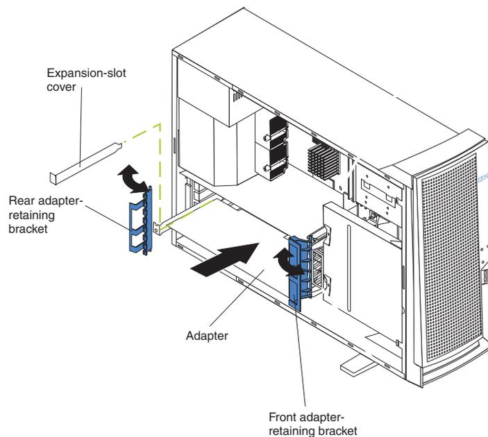
9. Connect required cables to the adapter. Route cables so that they do not block the flow of air from the fans. If you are installing an optional SCSI adapter, see "Cabling an optional SCSI adapter" on page 18 for additional information.
