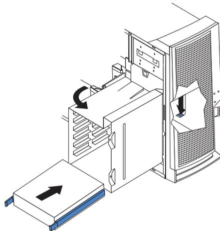
5. Attach the blue guide rails to the side of the drive using the screws that are provided.
