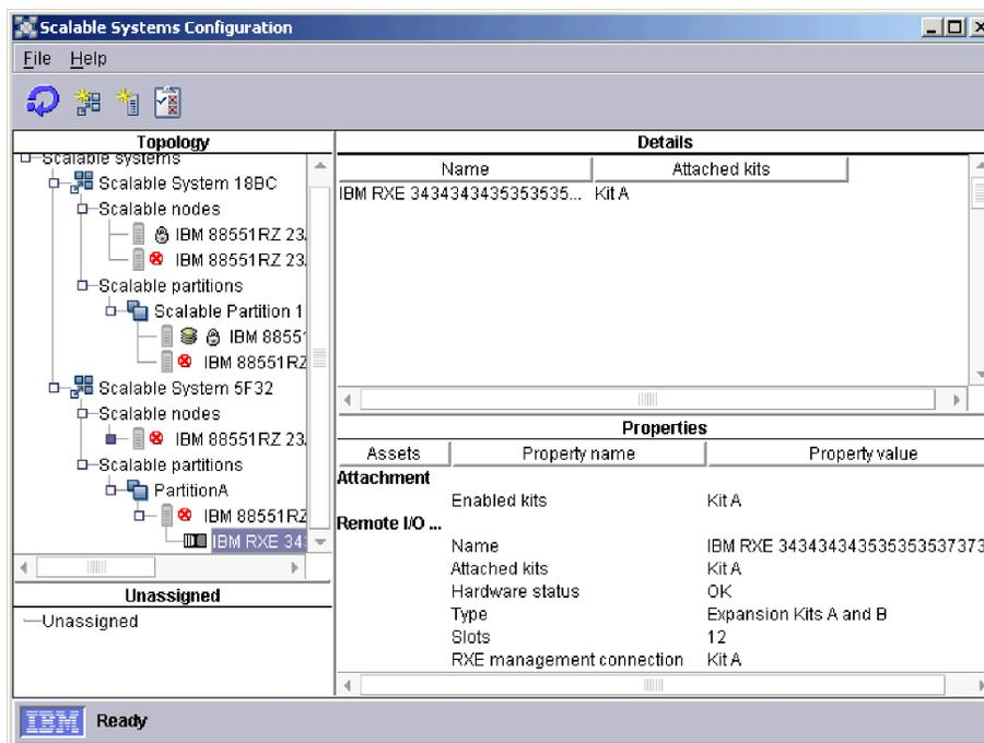
Figure 36. Displaying information about one remote I/O enclosure
