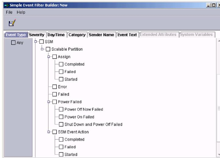
Figure 37. Scalable System Manager events in the “Simple Event Filter Builder” window
