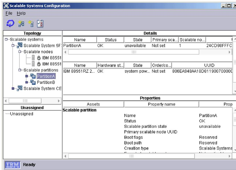
Figure 35. Displaying information about one scalable partition
