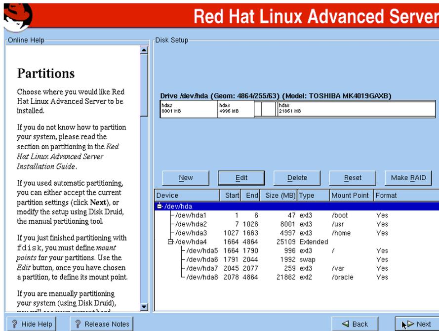
Figure 30. Disk setup with modified partitions
