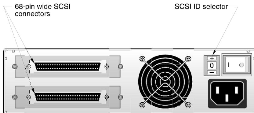
**FIGURE 11.** Back Panel of the External Tape Drive
