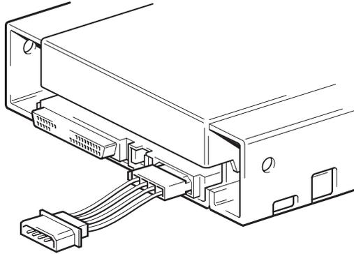
**FIGURE 10.** Power Connector on the Internal Tape Drive
