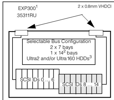
1. Housed in a 19in rack mountable drawer and ships standard with redundant 500W hot-swap power supplies, two power cords and a single 2M Ultra2 SCSI cable capable of supporting Ultra160 speeds.
