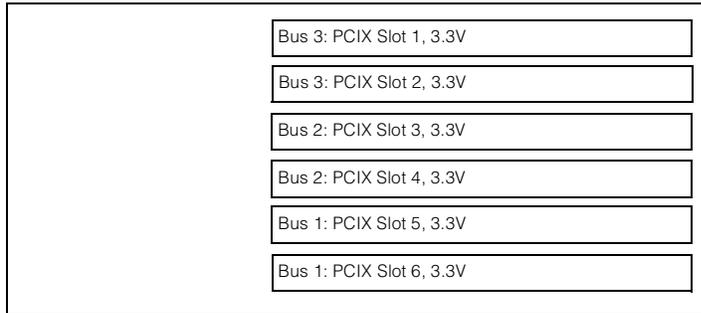
All slots are 64-bit, full-length, 133MHz Active PCI-X. Each bus supports only one 133MHz adapter. If two 133MHz adapters are installed, both will operate at 100MHz. If a lower frequency adapter is installed, the bus will operate at that frequency.
