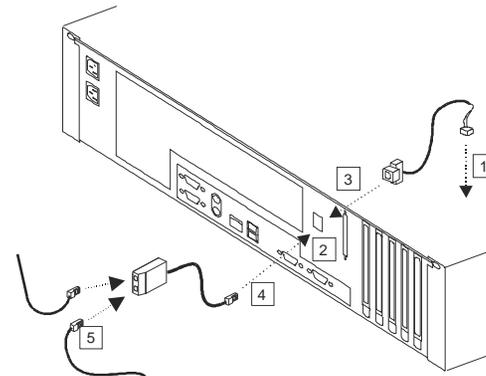
**9. Server with ASMP and no standard RS-485 ports, into which an optional ASMA is installed**
