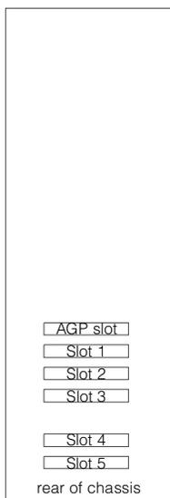
All PCI expansion slots are full-length, 32-bit, 33MHz, 5v on a single PCI bus.
