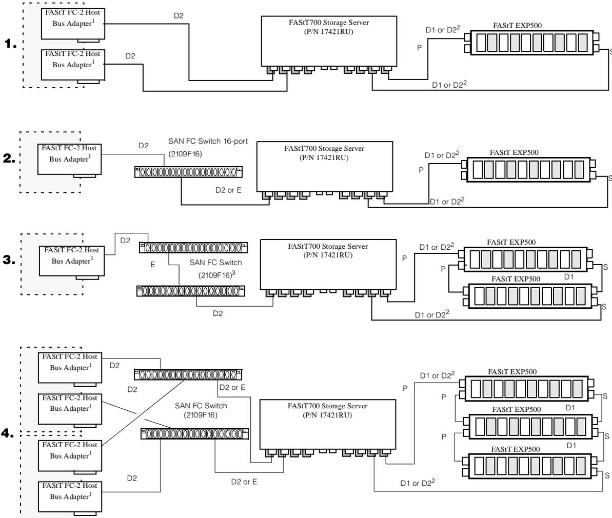
1. FASt FC-2 Host Bus Adapter (P/N 19K1246) includes an integrated short-wave SFF Module, supporting short-wave connections only.
