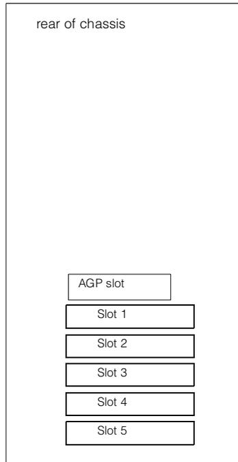
All PCI expansion slots are full-length, 32-bit, 33MHz, 5V or universal on a single PCI bus.
