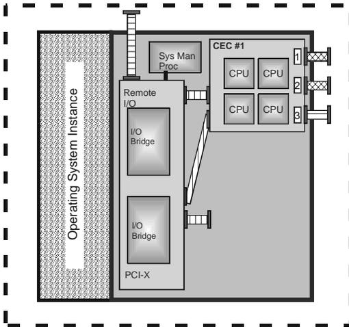
Logical diagram of SMP Expansion Module cabling (including scalability cables) for single node, eight-way x440 running one operating system
