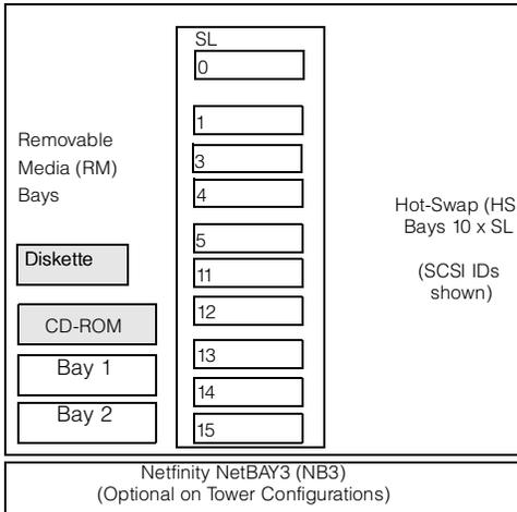
Bus A includes the top five bays supported by the standard integrated Ultra2 SCSI controller connected by a standard 16-bit LVDS cable. Bus B includes the lower five bays. For clarity, the SCSI IDs are identified
