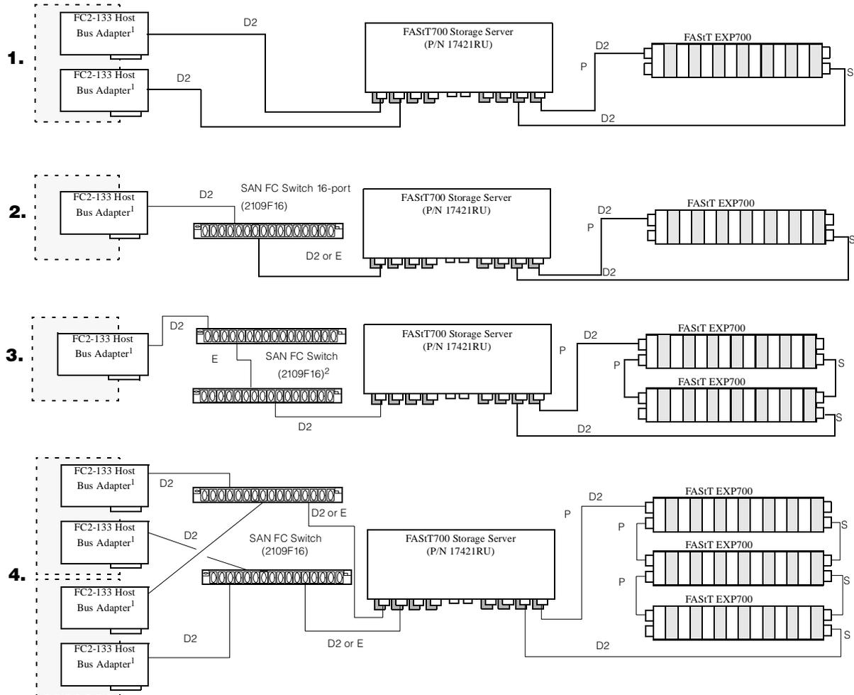
1. FC2-133 Host Bus Adapter (P/N 24P0960) includes an integrated short-wave SFF Module, supporting short-wave connections only.
