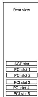
Slot 1: Bus C, 32-bit, 33MHz, 5v, half-length
