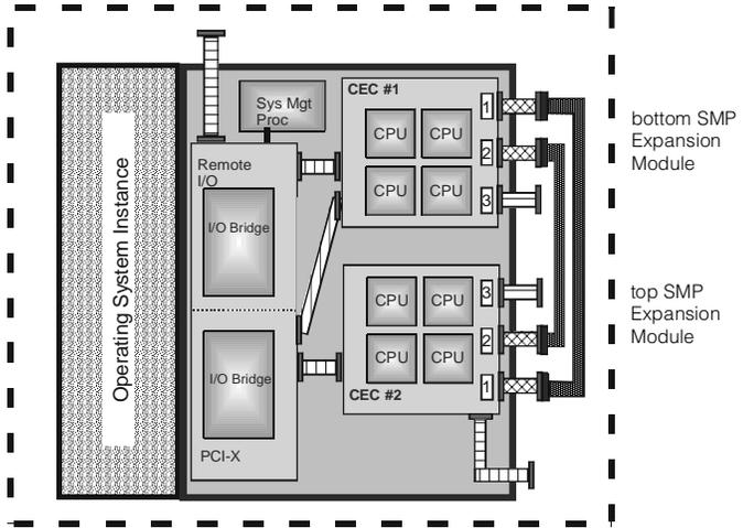
Logical Diagram of SMP Expansion Module cabling for 16-way x440 (two eight-way models) running one operating system. The top SMP Expansion Modules in each chassis are labeled CEC #2. Scalability ports are shown top to bottom one to three.
