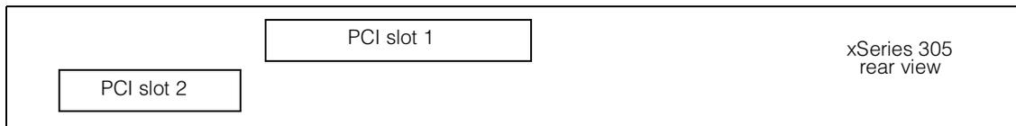
Slot 1: Bus 1, 64-bit, 66/100/133MHz PCI-X, full-size, half-length, 3.3v
