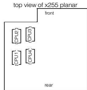
1. Three additional processors may be installed, providing a maximum of four. All processors must be identical in type, speed, and cache size. See diagram for order of installation.
