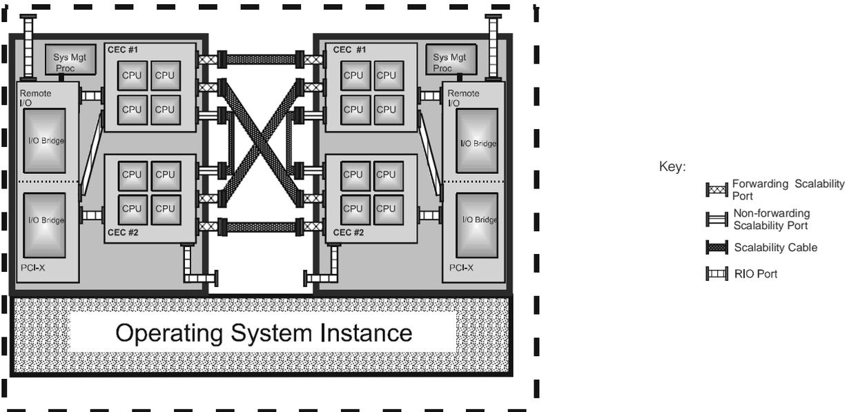
**SMP Expansion cabling configuration (rear view of system chassis')**
