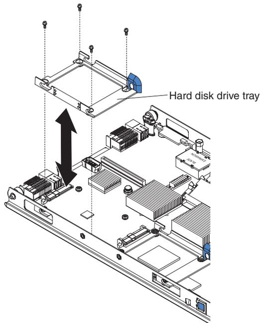
1. Place the drive tray into position on the system board and install the four screws to secure it.
