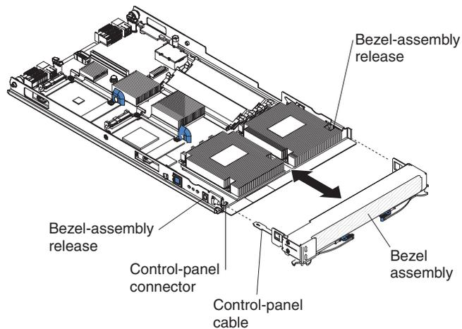
1. Connect the control-panel cable to the control-panel connector on the system board.
