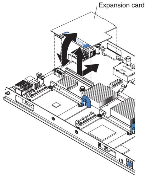
1. Touch the static-protective package that contains the expansion card to any *unpainted* metal surface on the BladeCenter unit or any *unpainted* metal surface on any other grounded rack component; then, remove the expansion card from its package.
