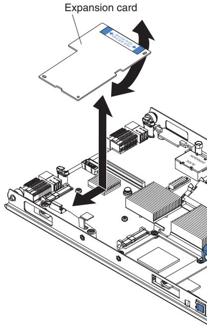
1. Touch the static-protective package that contains the expansion card to any *unpainted* metal surface on the BladeCenter unit or any *unpainted* metal surface on any other grounded rack component; then, remove the expansion card from its package.
