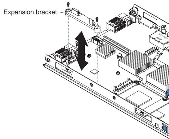
1. Place the expansion bracket in position on the system board and install the two screws that secure it to the system board.
