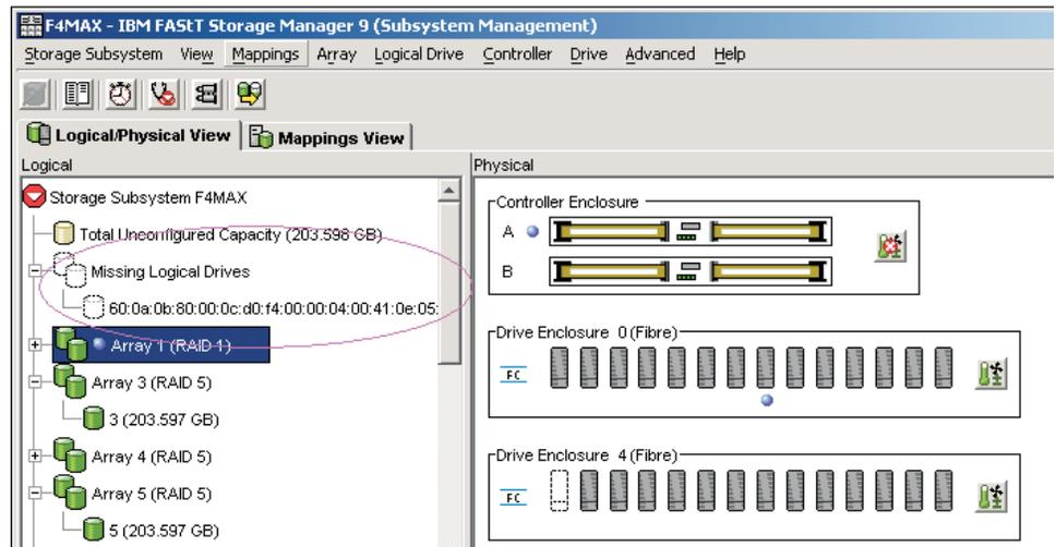
Figure 20. Subsystem Management Logical/Physical View of Missing Logical Drives
