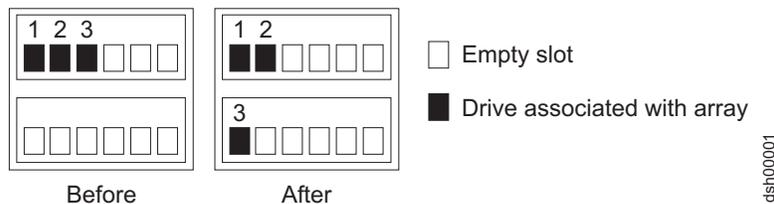
Figure 18. Manner recommended for reordering a defined array using empty slots in two storage enclosures
