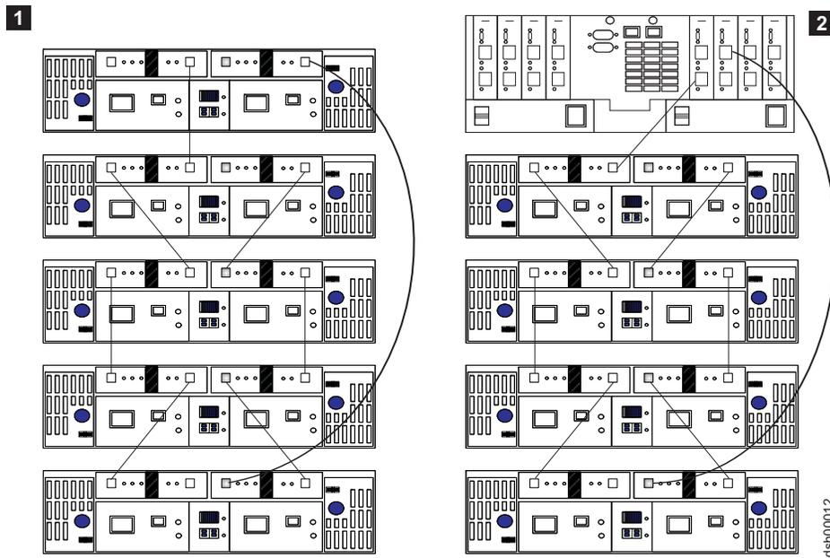
Figure 12. Unacceptable cable loop scheme for connecting DS4000 storage devices
