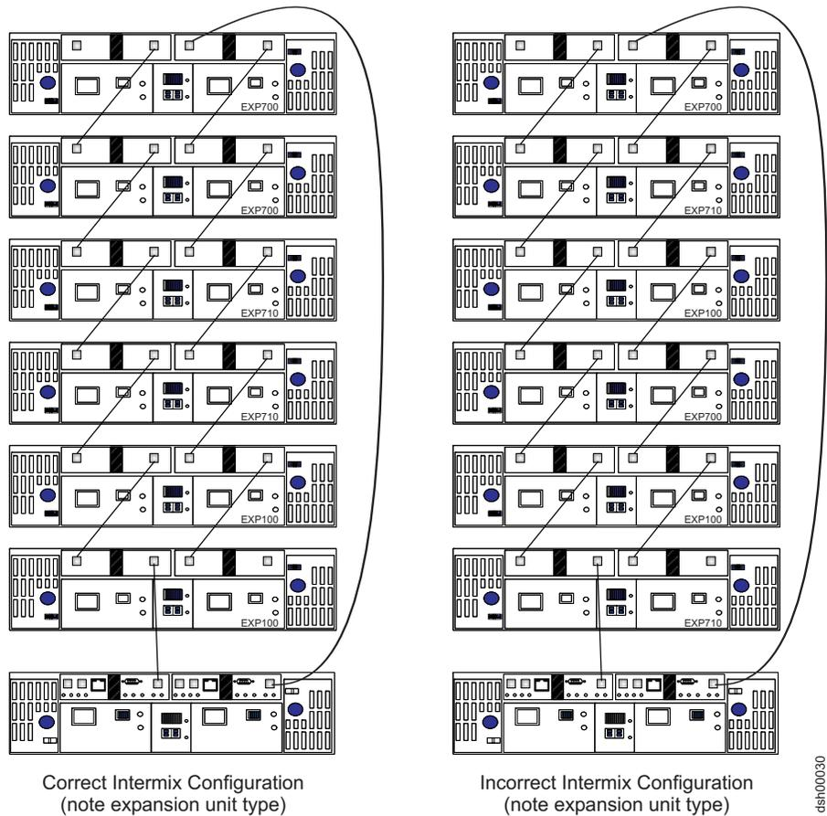
Figure 8. Correct and incorrect ways to group DS4000 storage expansion enclosures in a redundant drive loop
