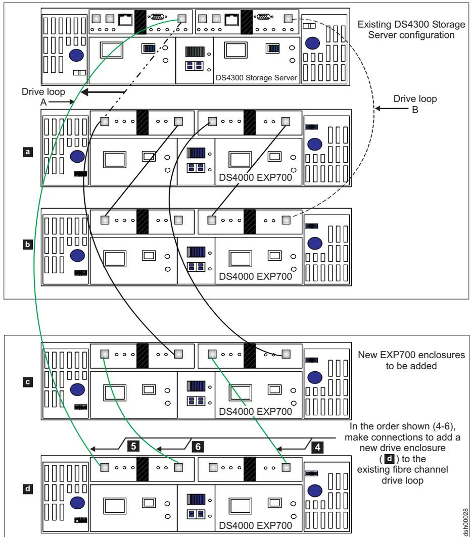
Figure 29. Cabling a second drive enclosure to the beginning of a functioning drive loop
