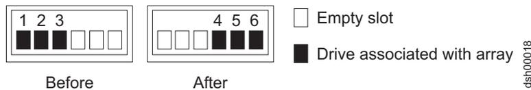
Figure 17. Manner recommended for reordering a defined array using empty slots in one storage enclosure
