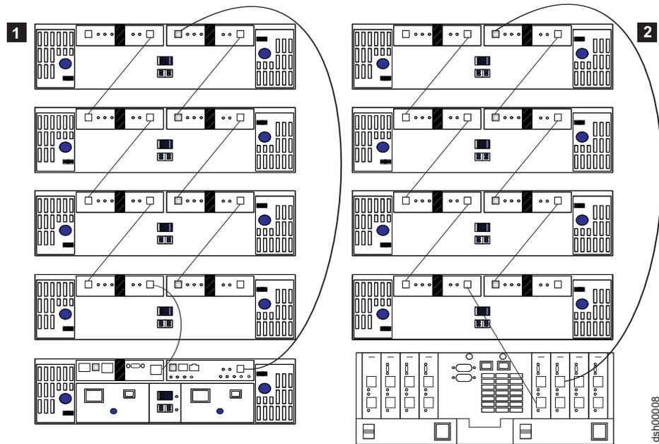
Figure 9. Recommended cable loop scheme for connecting DS4000 storage devices
