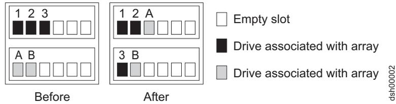
Figure 19. Reordering multiple defined arrays across previously used slots in two storage enclosures
