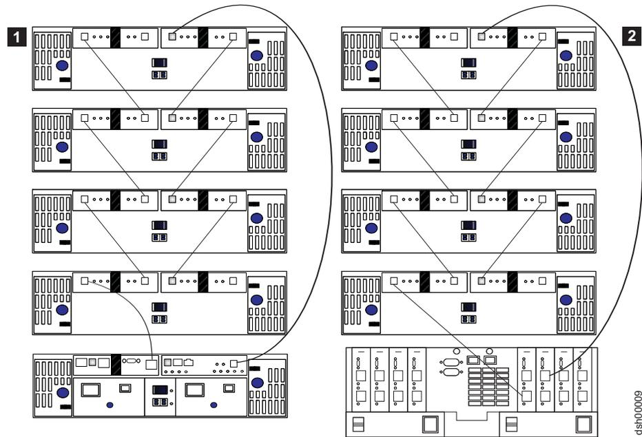
Figure 13. Unacceptable cable loop scheme for connecting DS4000 storage devices
