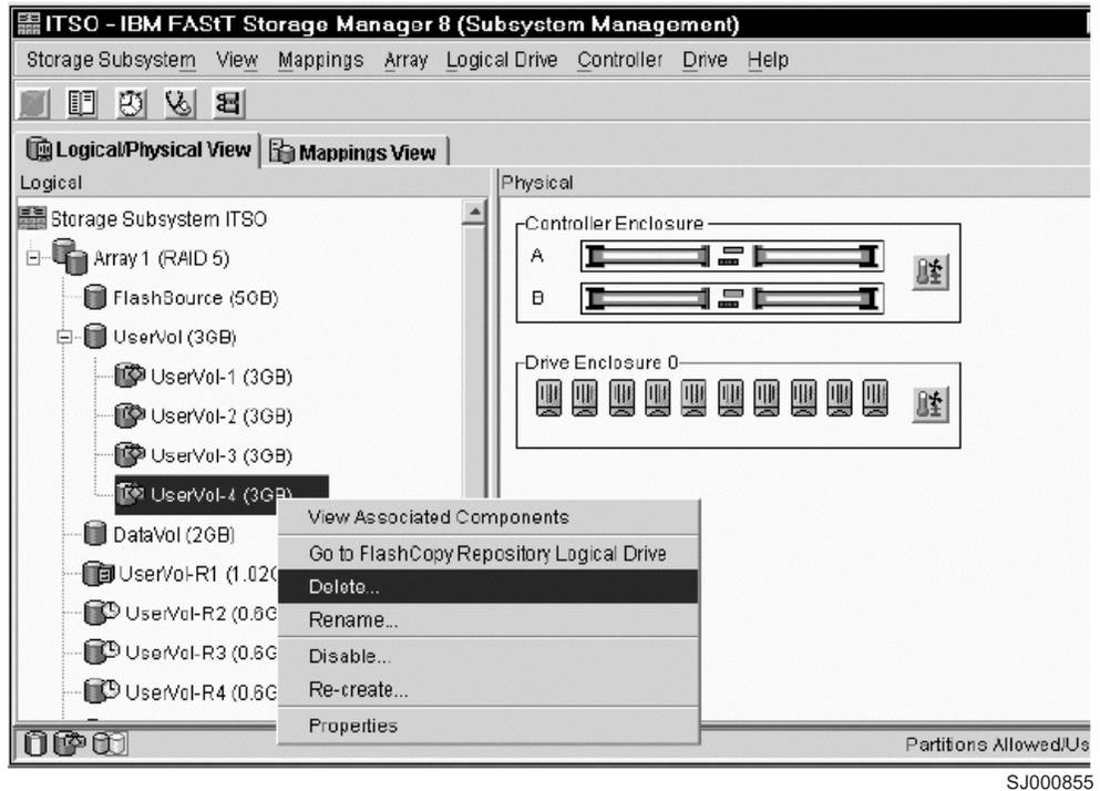
Figure 50. Deleting the FlashCopy logical drive
