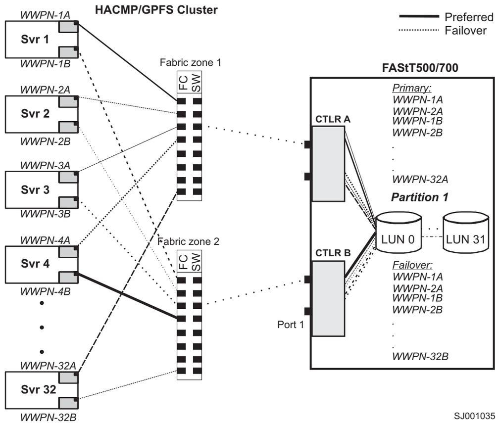
Figure 18. HACMP/GPFS Cluster Configuration example with single FASt500/700, shown with one partition per FASt
