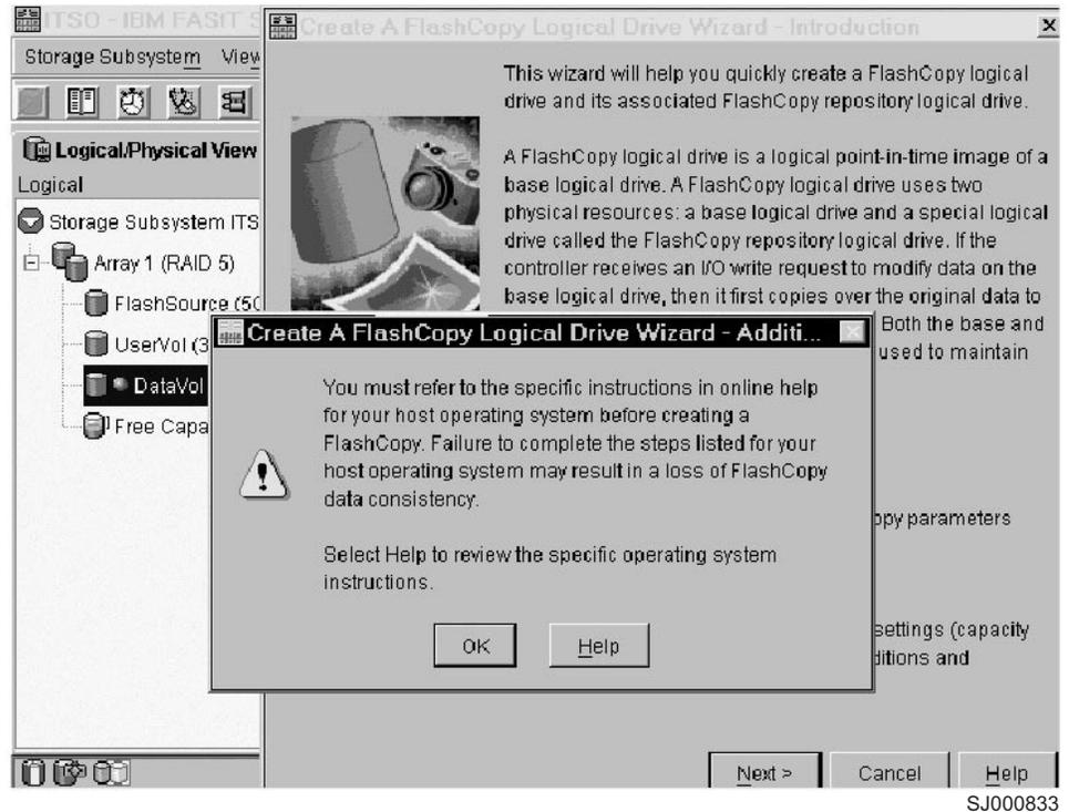
Figure 28. Create a FlashCopy Logical Drive Wizard startup
