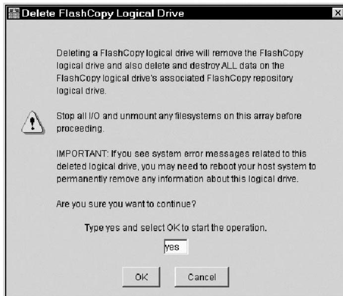
Figure 51. Delete FlashCopy Logical Drive Dialog window
