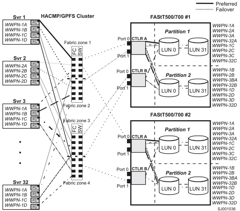
Figure 19. HACMP/GPFS Cluster Configuration example with multiple FAST500/700, shown with two partitions per FAST
