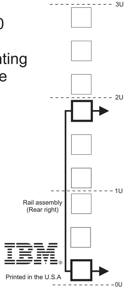
Figure 51. Rear rack mounting template
