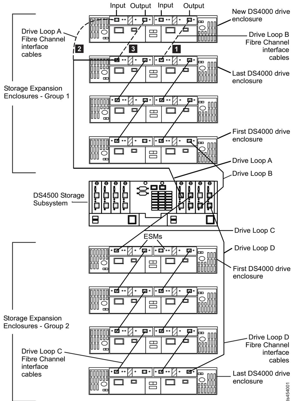
Figure 42. Cabling the EXP100 to two redundant loops
