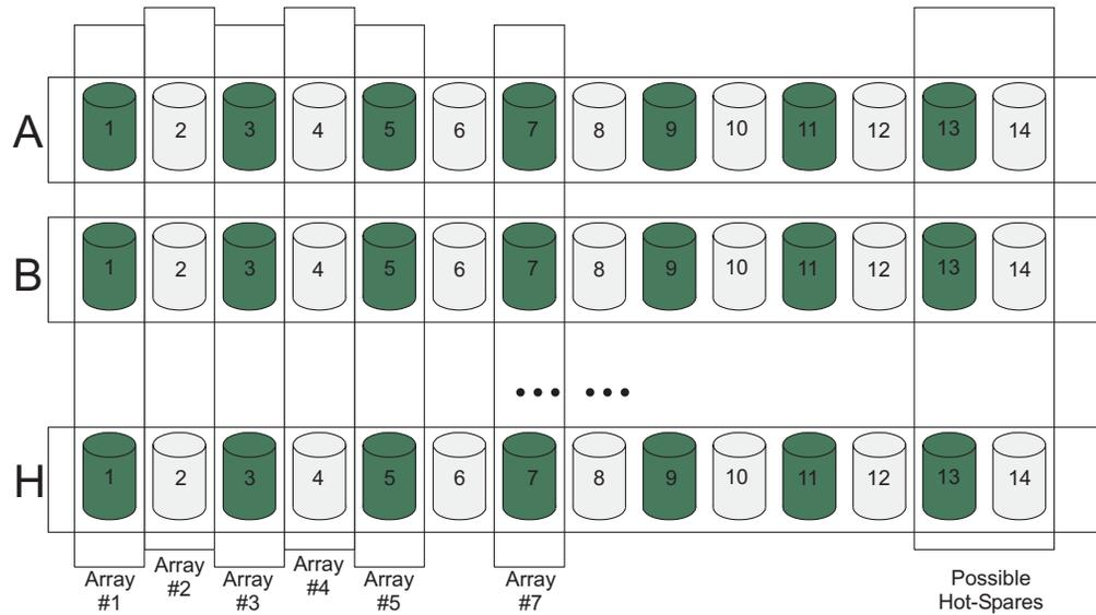
Figure 12. Orthogonally striped RAID arrays – Option 1
