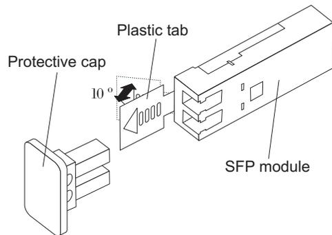
Figure 30. Unlocking the SFP module latch - plastic variety
