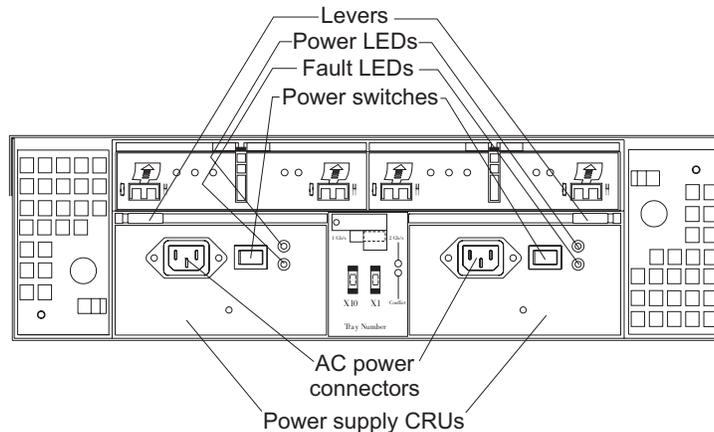
Figure 4. Power supply controls, indicators, and connectors
