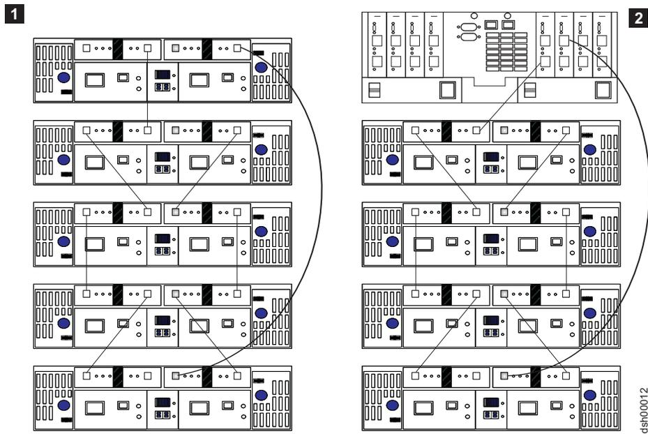
Figure 13. Alternate cable loop schemes possible but not recommended when connecting DS4000 storage devices (4 of 4)
