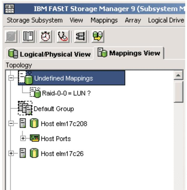
Figure 9. Undefined FlashCopy disk
