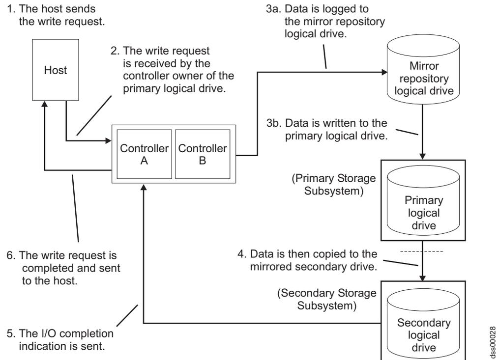
Figure 27. Data replication between primary and secondary storage subsystems: Synchronous write mode (Metro Mirroring)
