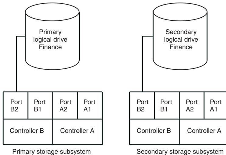
Figure 35. Controller B shown as controller owner
