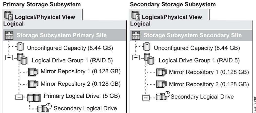
Figure 30. Mirrored logical drive pair showing Synchronization-in-Progress status
