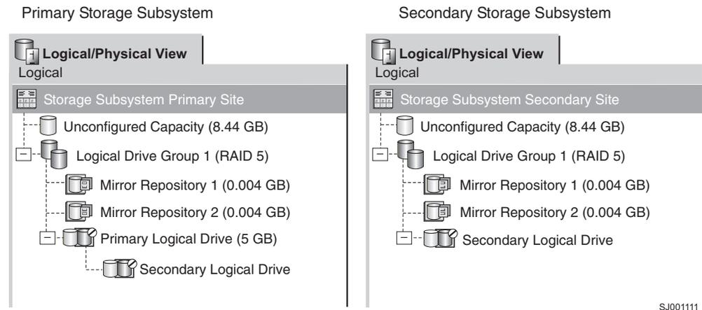
Figure 29. Mirrored logical drive pair showing Unsyncronized status
