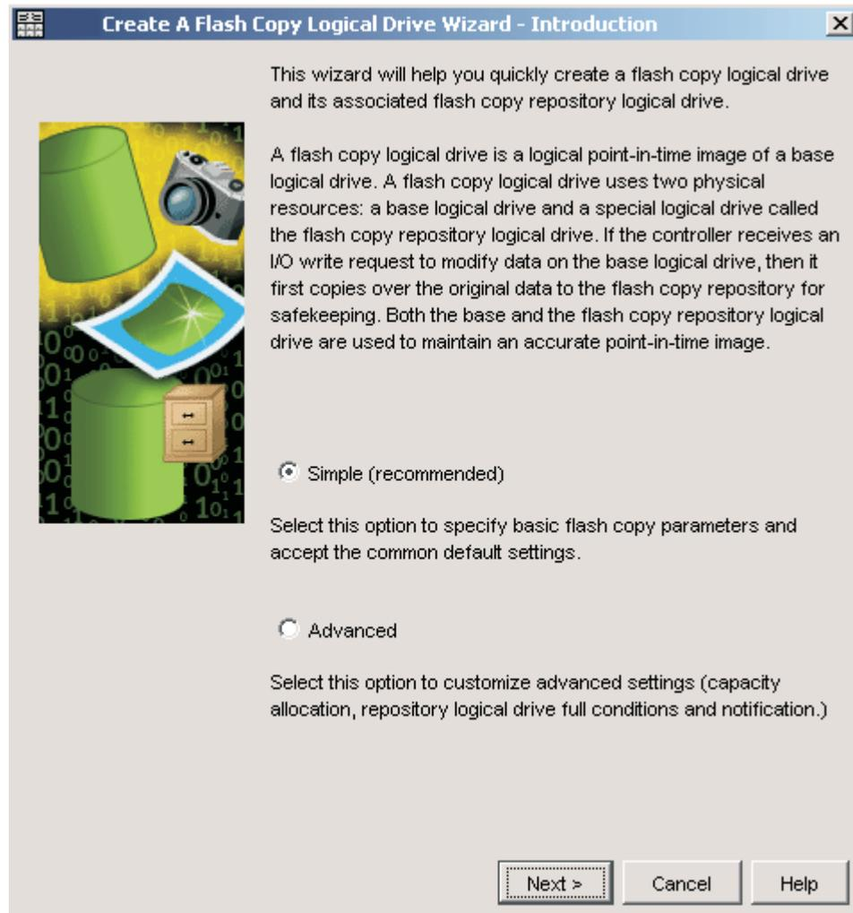
Figure 2. FlashCopy Logical Drive Wizard Introduction panel
