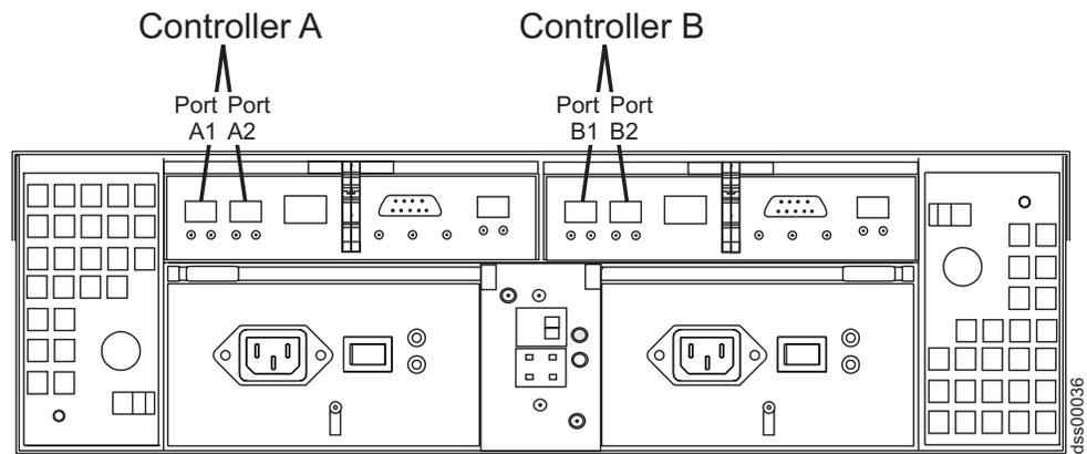
Figure 32. Controller A and Controller B host ports, machine type 1722
