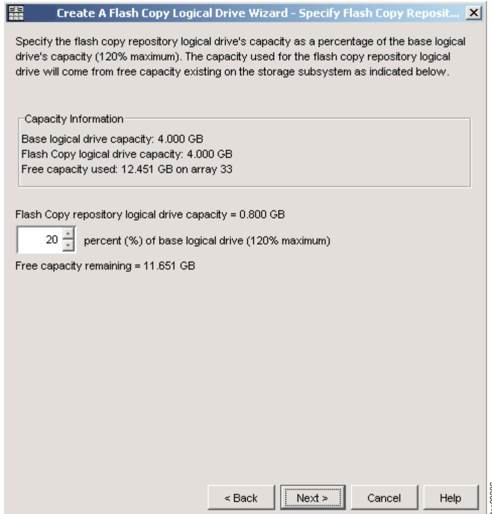
Figure 7. Specify Repository Logical Drive Capacity panel
