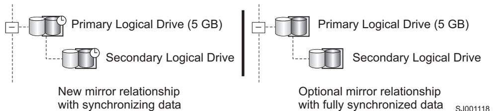
Figure 43. Synchronizing and optimal mirror relationship icons
