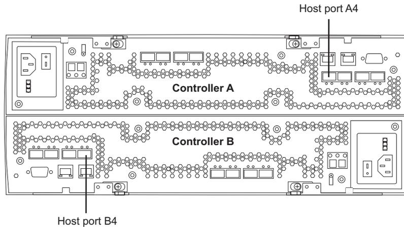
Figure 33. Controller A and Controller B host ports, machine type 1815
