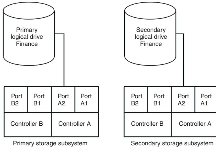
Figure 34. Controller A shown as the controller owner
