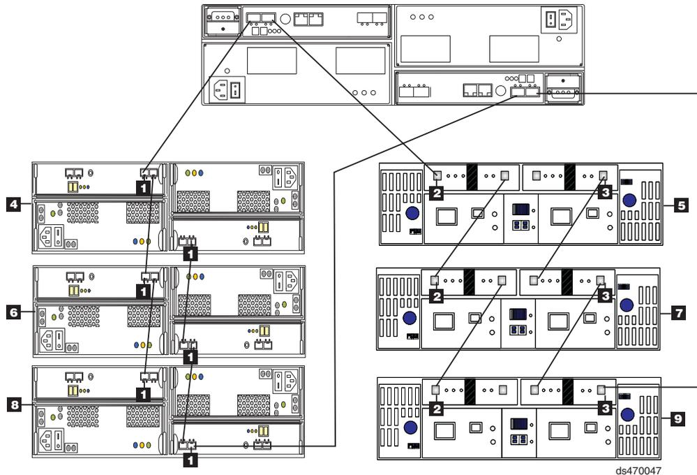
Figure 60. One DS4700 and two or more storage expansion enclosures in a mixed environment — Recommended cabling
