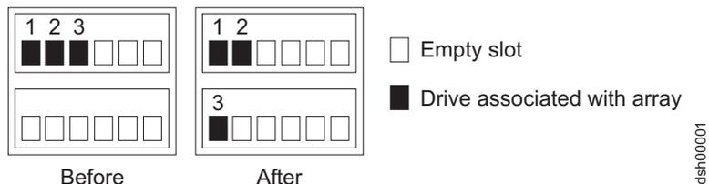
Figure 20. Manner recommended for reordering a defined array using empty slots in two storage enclosures
