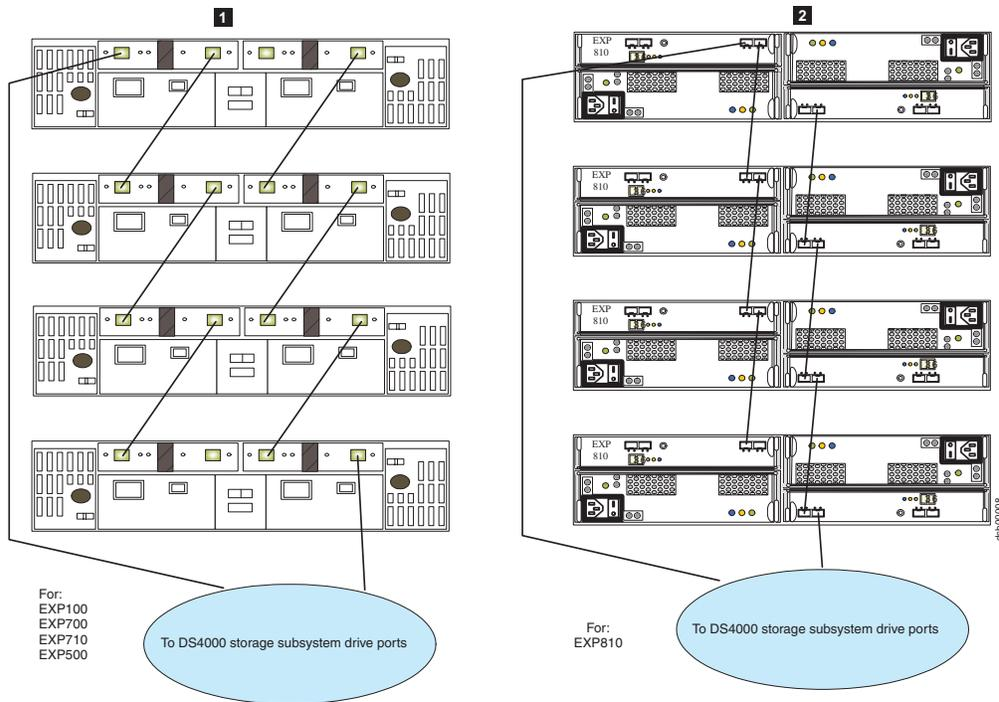
Figure 11. Recommended cable loop scheme for connecting DS4000 storage devices
