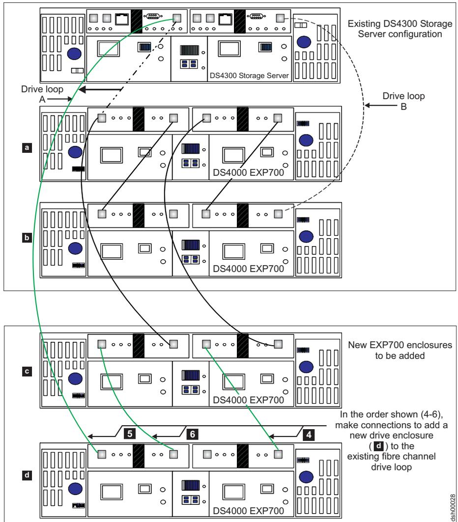
Figure 33. Cabling a second drive enclosure to the beginning of a functioning drive loop
