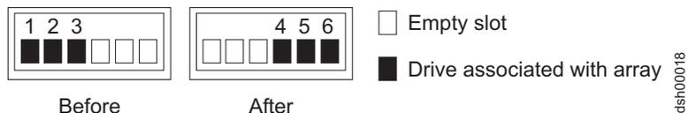
Figure 19. Manner recommended for reordering a defined array using empty slots in one storage enclosure
