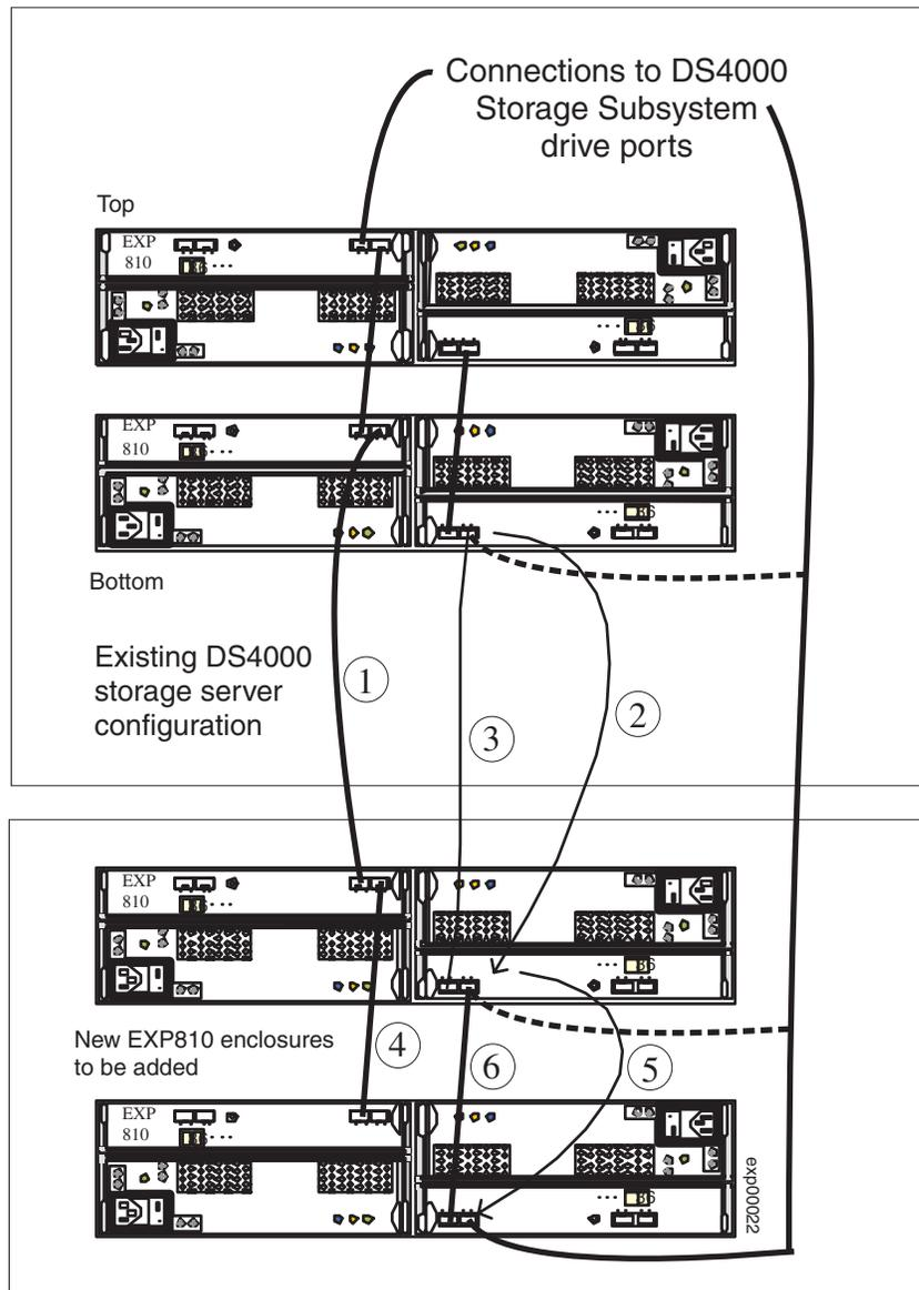
Figure 35. Cabling a second EXP810 drive enclosure to the end of a functioning drive loop
