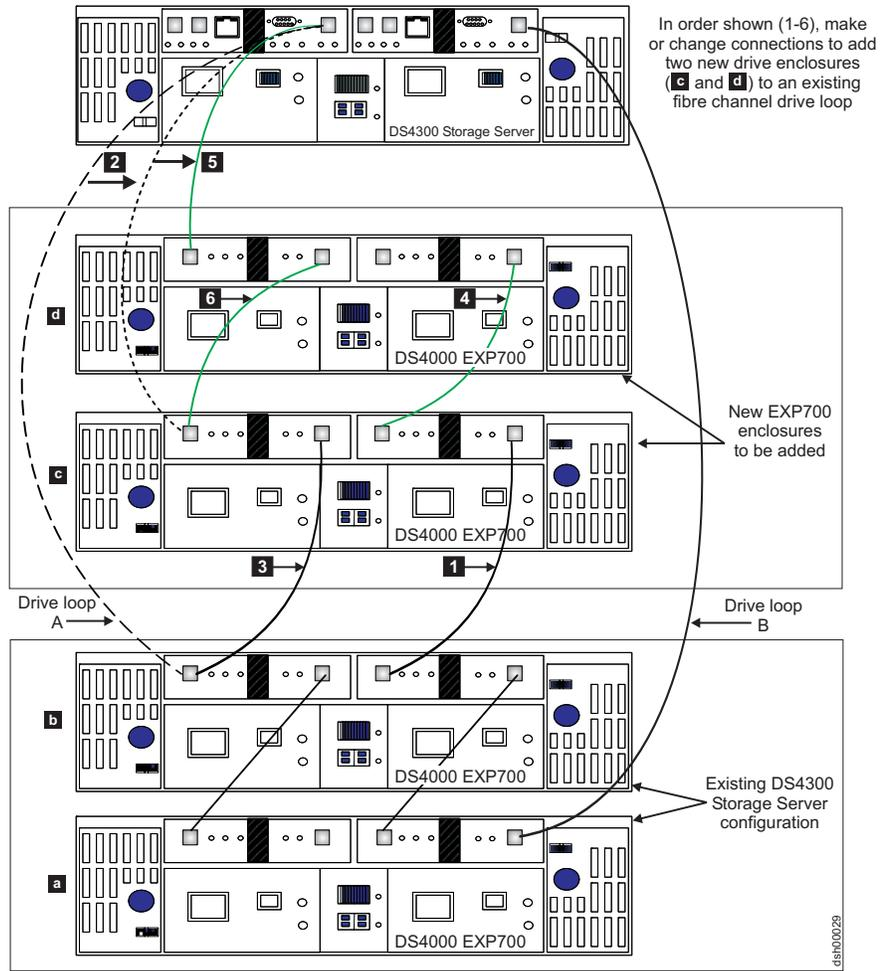
Figure 34. Recommended connection: Planned cabling of additional drive enclosures to the beginning of a functioning drive loop
