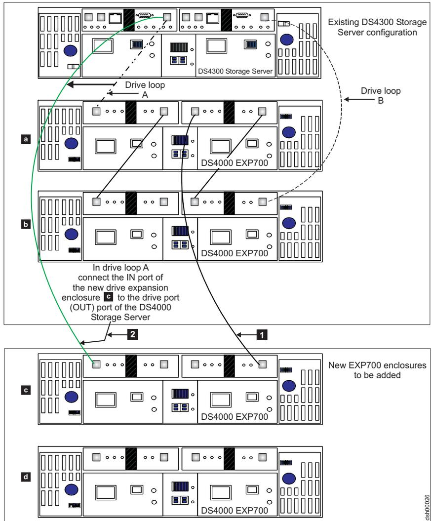
Figure 29. Cabling a single drive enclosure to the beginning of a functioning drive loop (step 2 of 3)
