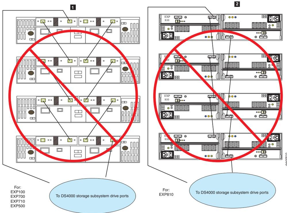
Figure 13. Not recommended alternate cable loop scheme for connecting DS4000 storage devices
