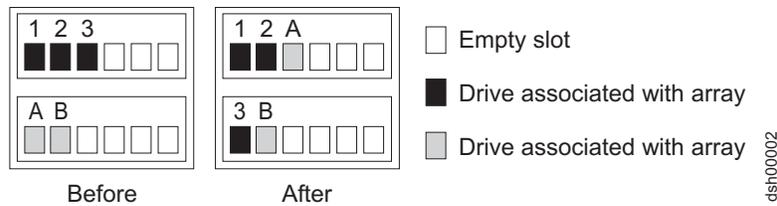
Figure 21. Reordering multiple defined arrays across previously used slots in two storage enclosures
