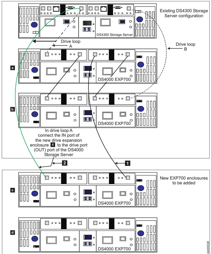
Figure 41. Cabling a single drive enclosure to the beginning of a functioning drive loop (step 2 of 3)
