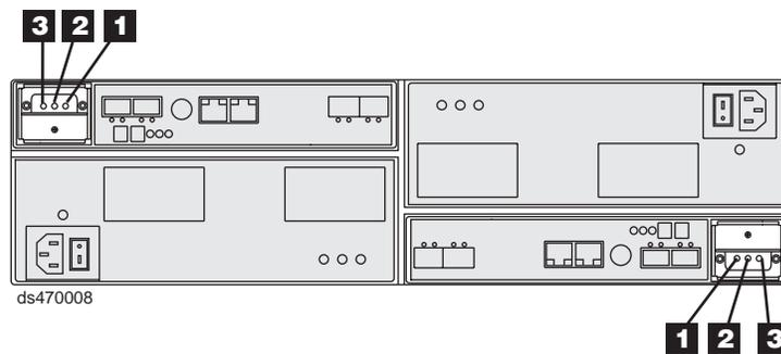
Figure 64. Battery unit LEDs
