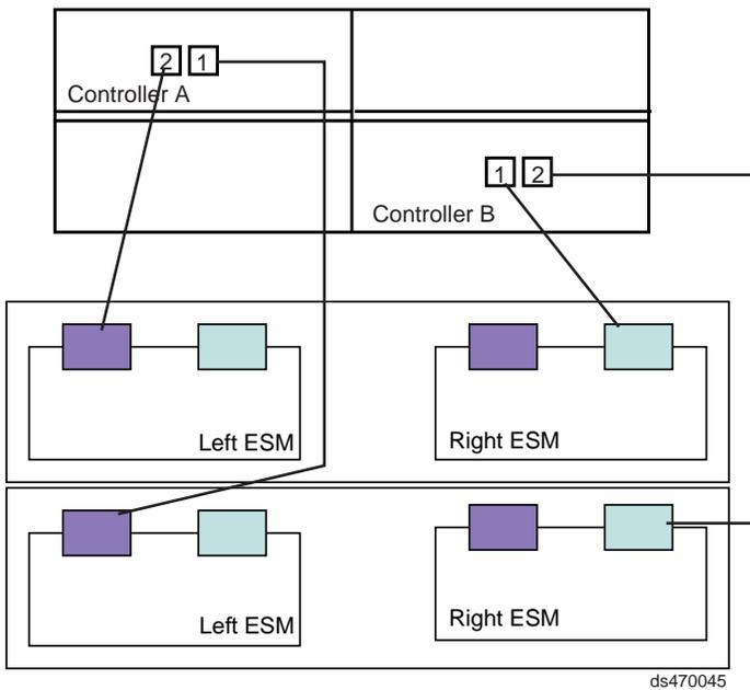
Figure 41. One DS4200 Express and two storage expansion enclosure — Recommended cabling
