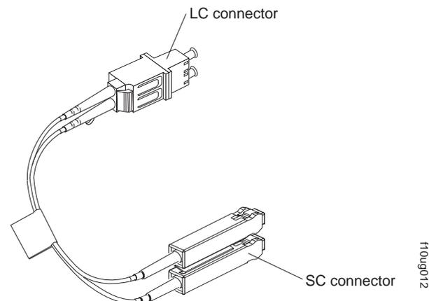
Figure 32. LC-SC fibre-channel cable adapter
