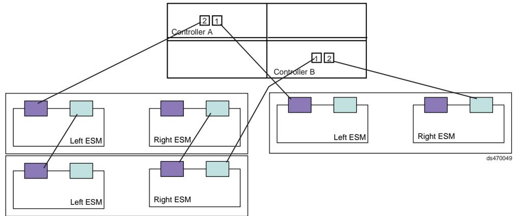
Figure 42. One DS4200 Express and three storage expansion enclosure — Recommended cabling
