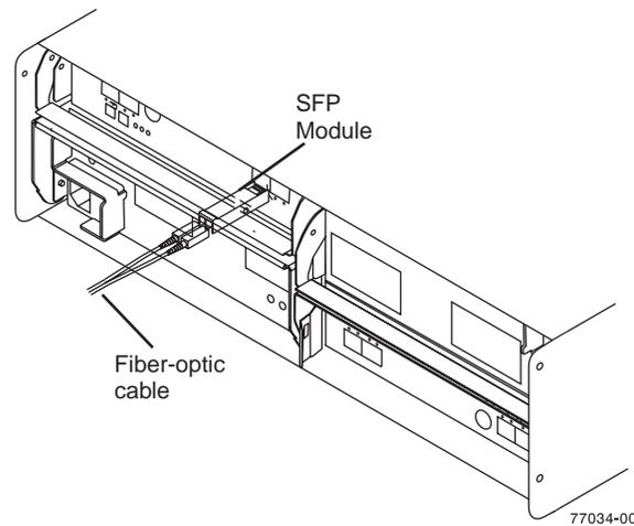
Figure 6. SFP module and fiber optic cable
