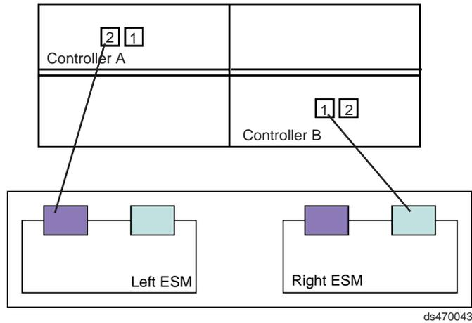
Figure 39. One DS4200 Express and one storage expansion enclosure — Recommended cabling
