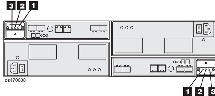
Figure 68. Battery unit LEDs
