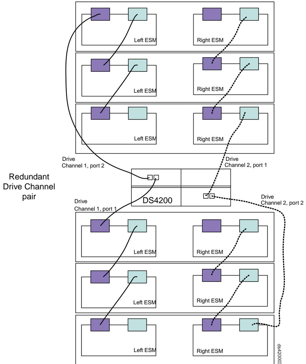
Figure 37. Example of a redundant drive channel pair
