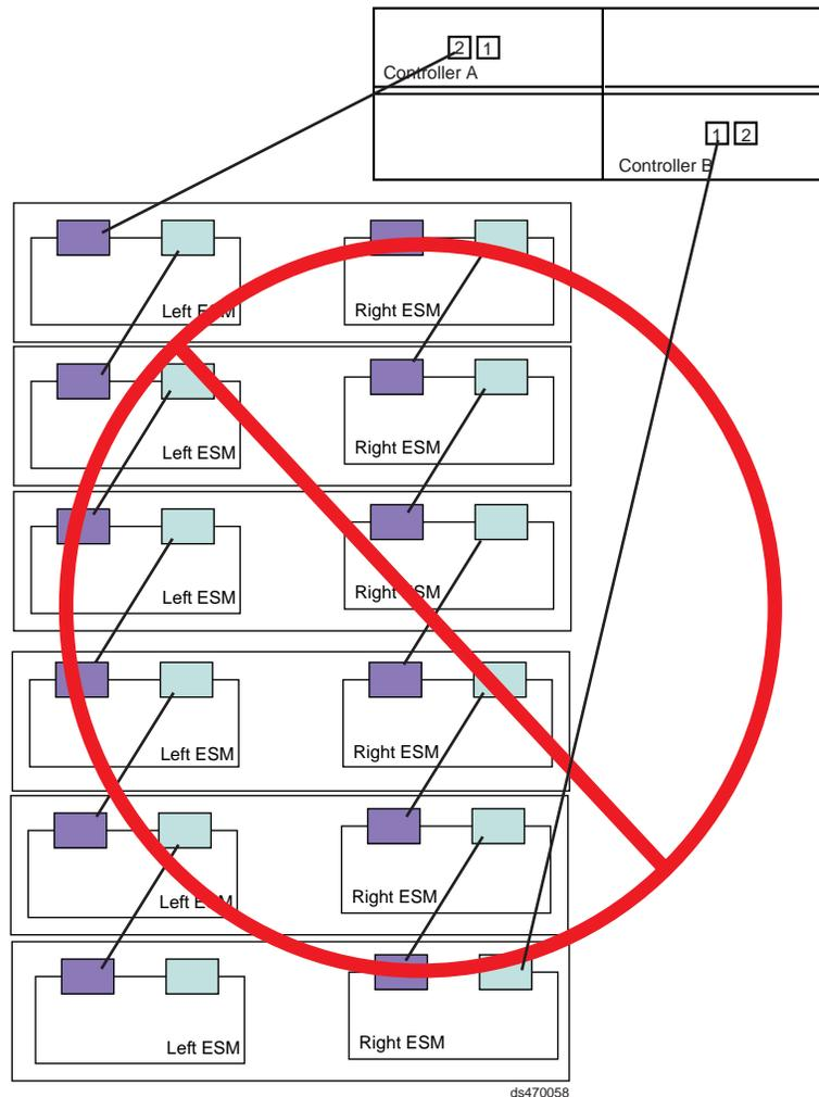
Figure 45. One DS4200 Express and up to six storage expansion enclosure — Not recommended
