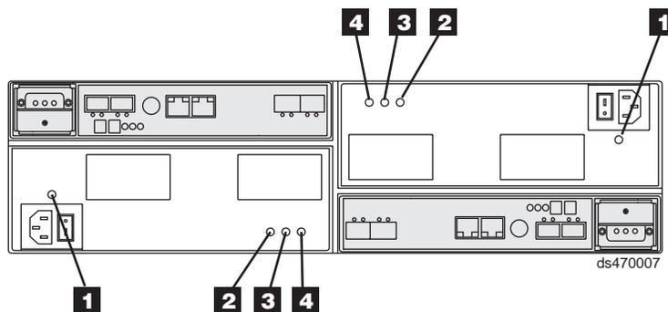
Figure 62. Power supply and fan unit LEDs
