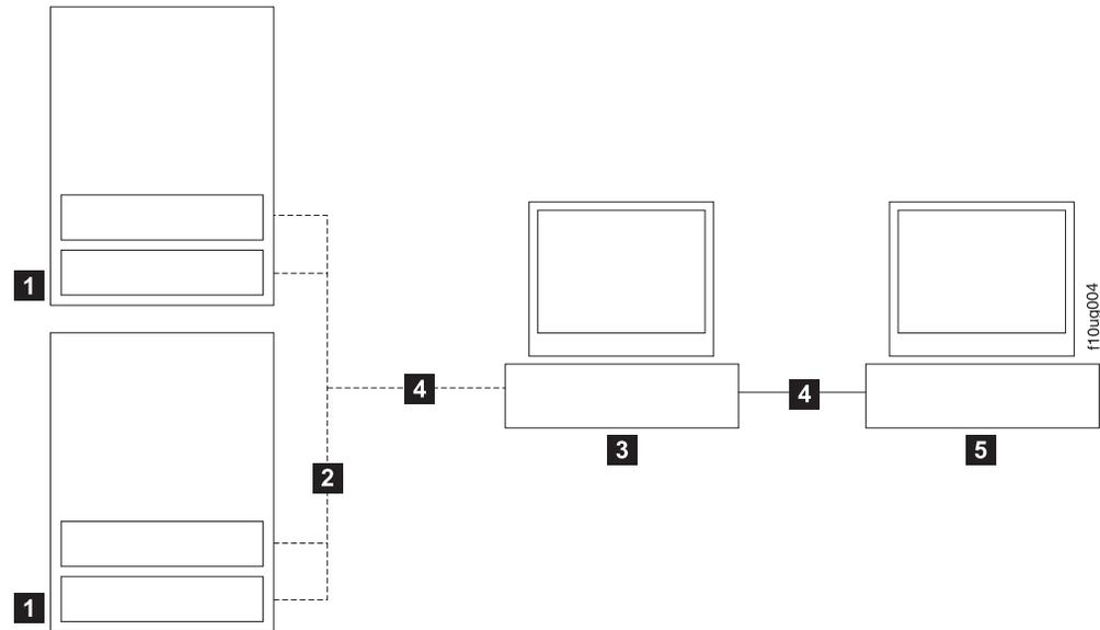
Figure 52. Host-agent (in-band) managed storage subsystems
