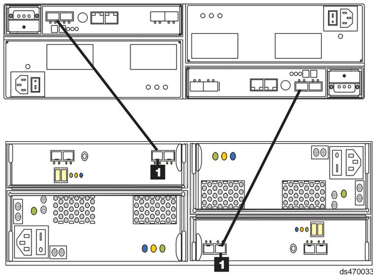
Figure 46. One DS4200 Express and one EXP420 storage expansion enclosure — Recommended cabling
