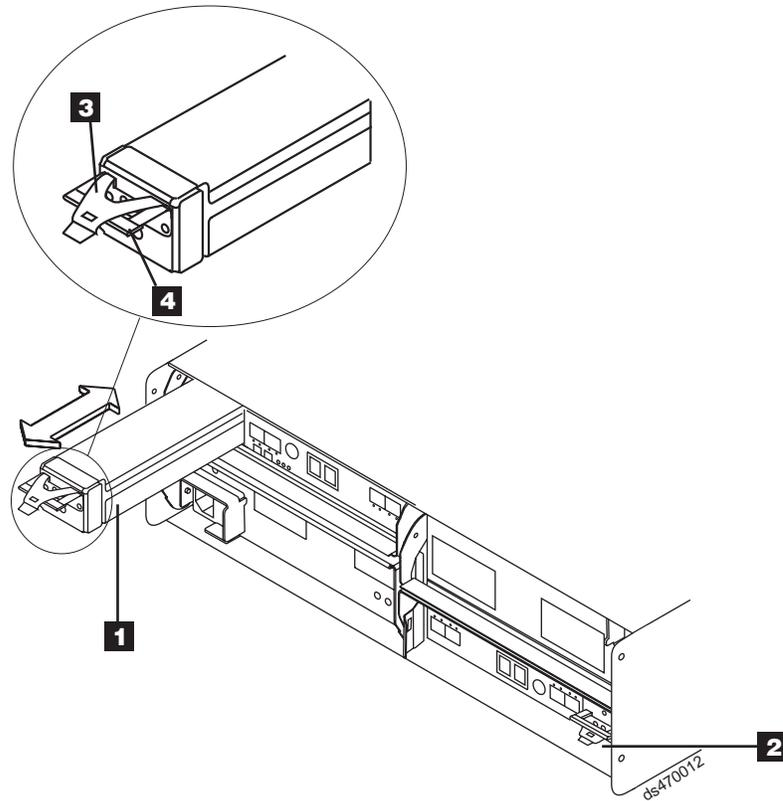
Figure 78. Removing and replacing a battery unit from the controller chassis
