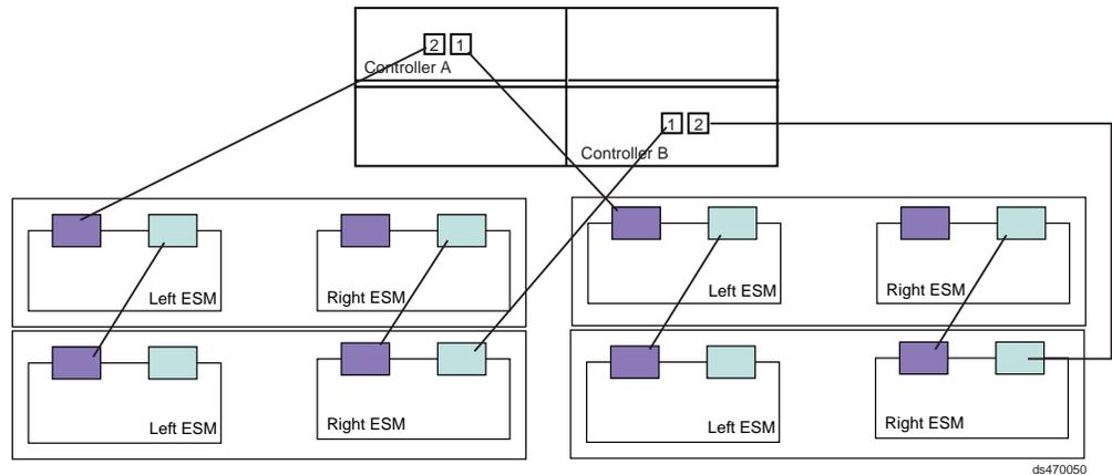
Figure 43. One DS4200 Express and four storage expansion enclosure — Recommended cabling
