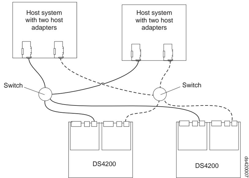
Figure 59. Example of two storage subsystems in a dual SAN environment
