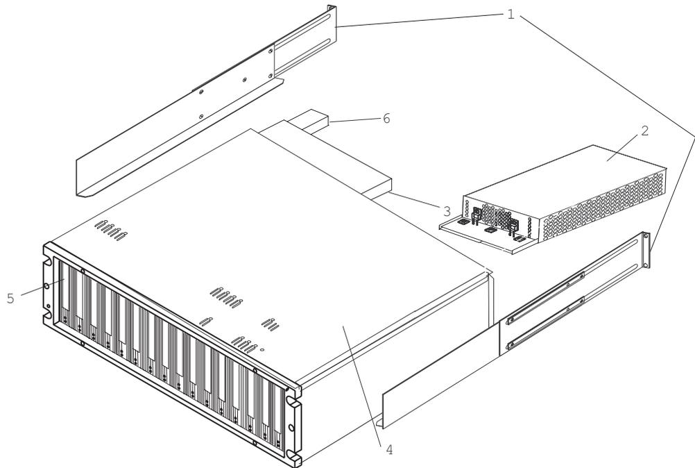
Figure 81. DS4200 Express storage subsystem parts list
