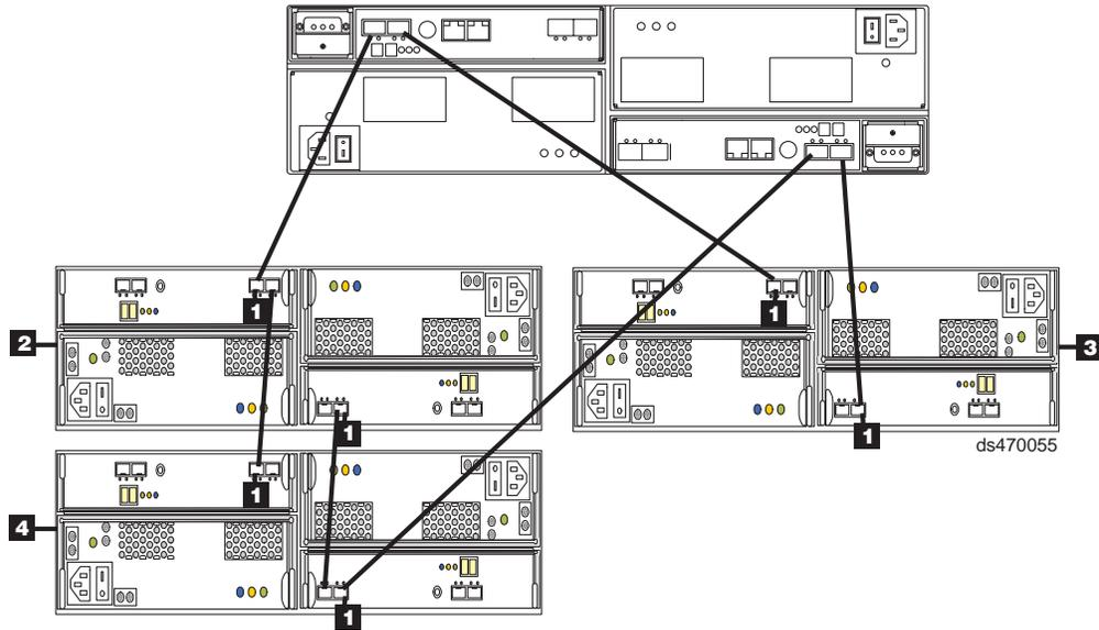
Figure 48. One DS4200 Express and three EXP420 storage expansion enclosures behind a pair of DS4200 Express drive ports
