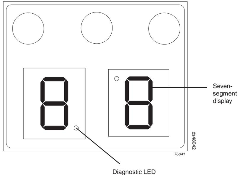
Figure 66. Numeric display LEDs
