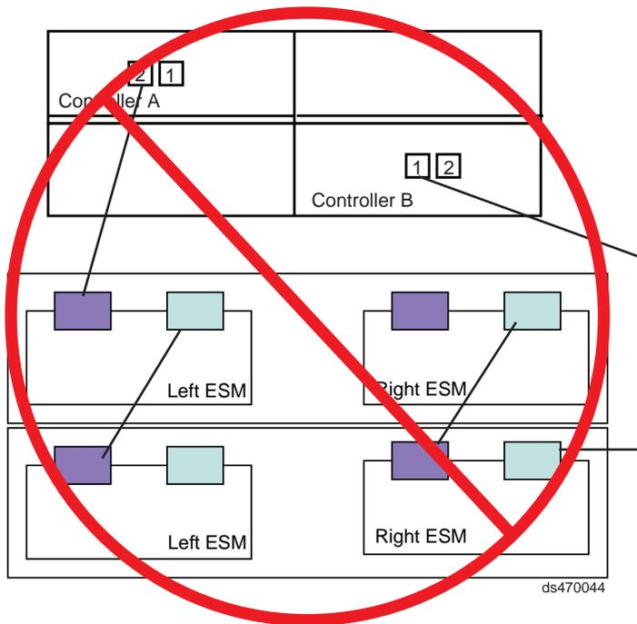
Figure 40. One DS4200 Express and two storage expansion enclosure — Not recommended cabling
