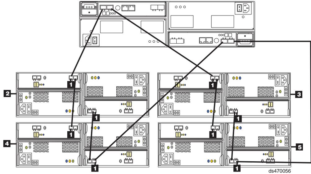
Figure 49. One DS4200 Express and four EXP420 storage expansion enclosures behind a pair of DS4200 Express drive ports
