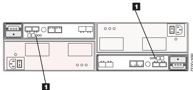
Figure 67. Cache Active LEDs
