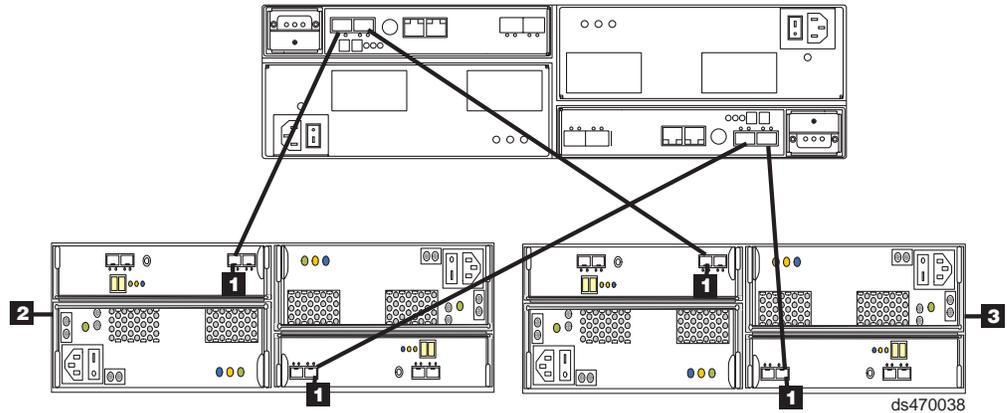
Figure 47. One DS4200 Express and two EXP420 storage expansion enclosures behind a pair of DS4200 Express drive ports
