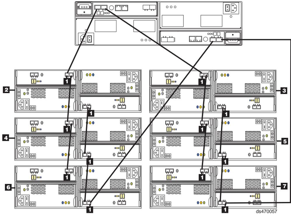
Figure 50. One DS4200 Express and a maximum of six EXP420 storage expansion enclosures behind a pair of DS4200 Express drive ports
