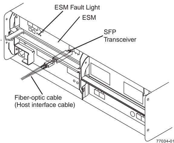
Figure 79. Replacing an SFP module
