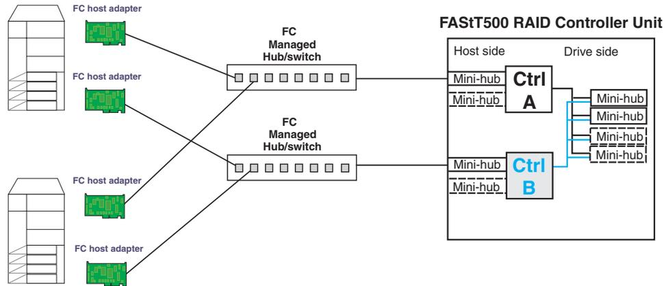
Figure 121. Type 2 configuration - With hubs
