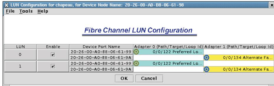
Figure 150. Fibre Channel LUN Configuration window
