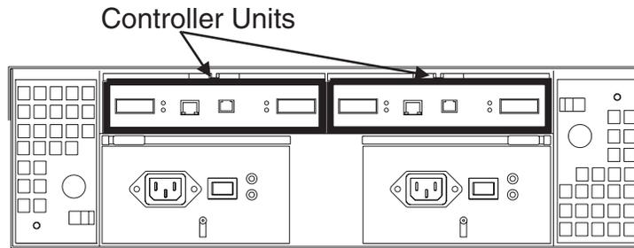
Figure 140. FAST200 fibre channel controller unit locations
