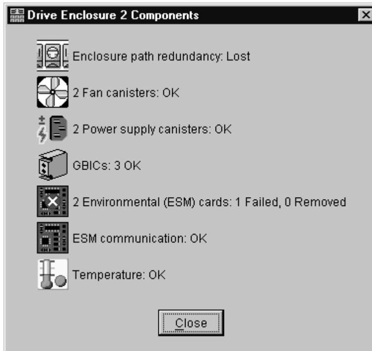
Figure 153. Drive enclosure components - ESM failure
