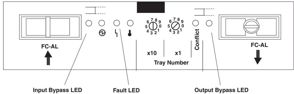
Figure 161. FAST EXP500 ESM indicator lights
