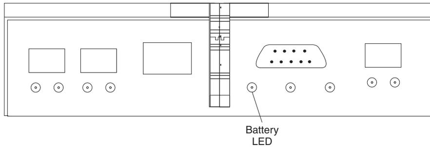
Figure 53. Type 1722 FAStT600 storage server battery LED
