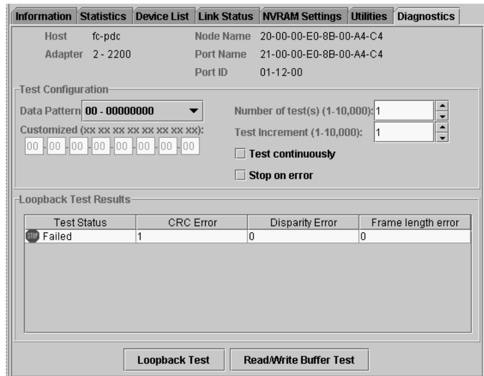
Figure 87. Test Results section of the Diagnostics panel
