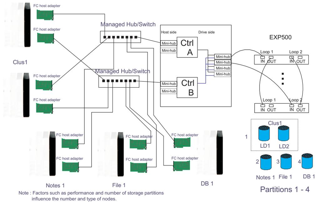
Figure 36. Type 3552 FAST500 RAID controller cluster/non-cluster share
