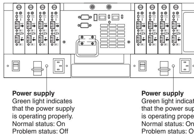
Figure 66. Type 1742 FASiT900 storage server power supply indicator light
