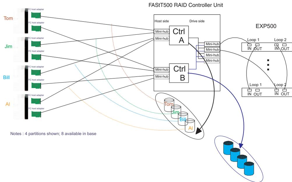
Figure 40. Type 3552 FAST500 RAID controller basic storage partitions
