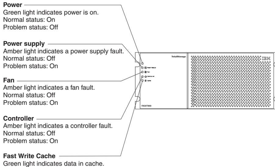
Figure 62. Type 1742 FASt900 storage server indicator lights
