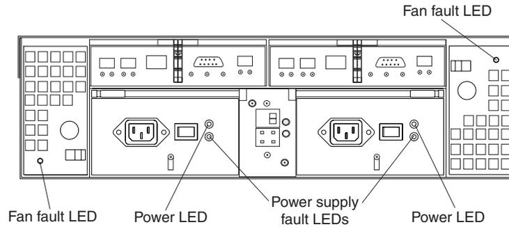
Figure 51. Type 1722 FASSt600 storage server fan and power supply LEDs
