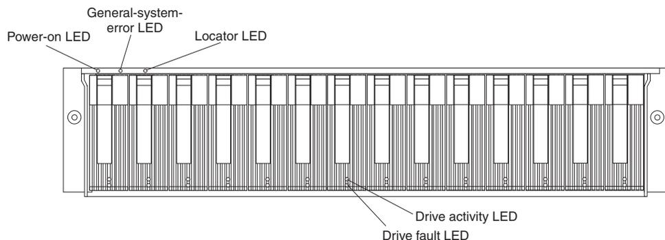
Figure 49. Type 1722 FASiT600 storage server LEDs (front)
