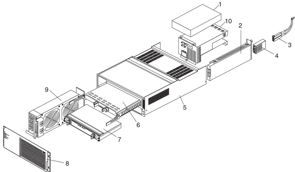
Figure 68. Type 1742 FASt900 storage server parts listing
