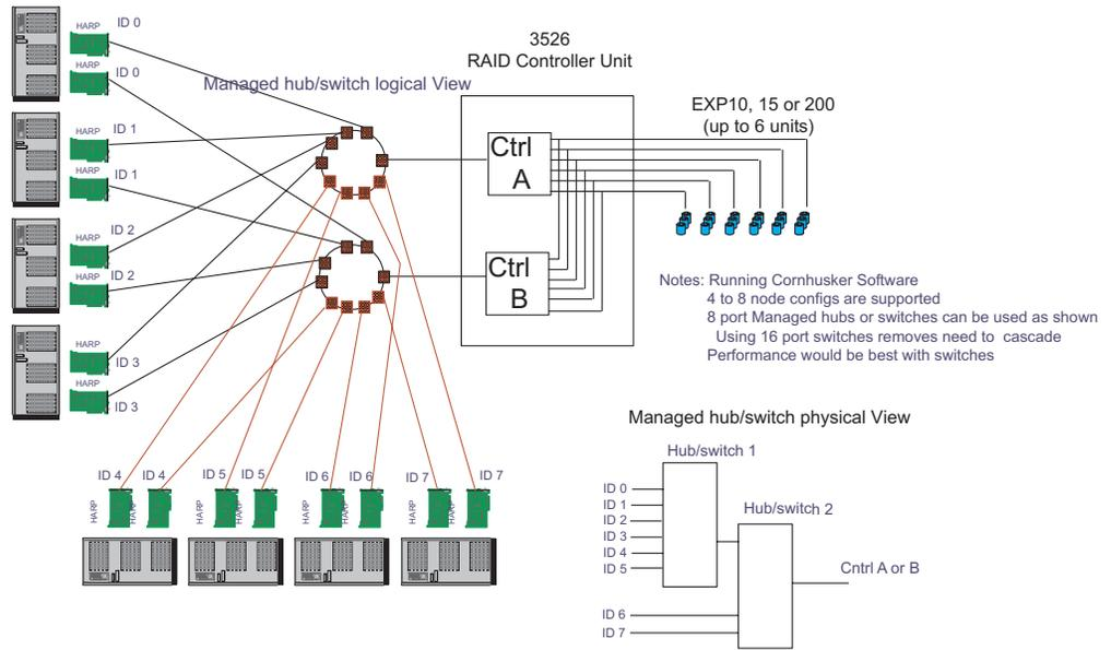
Figure 18. Type 3526 Fibre Channel RAID controller cornhusker configuration
