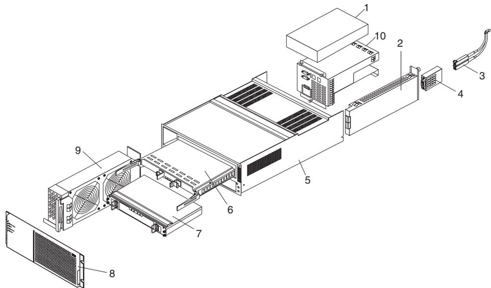
Figure 45. Type 3552 FASiT500 RAID controller parts listing
