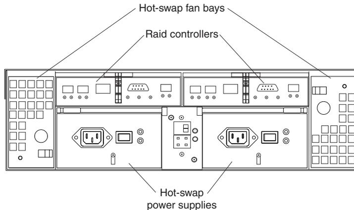
Figure 47. Type 1722 FAST600 storage server back view
