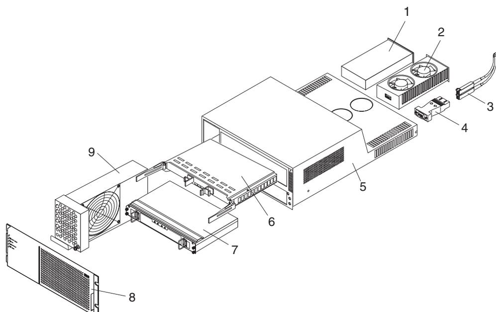
Figure 23. Type 3526 Fibre Channel RAID controller parts list
