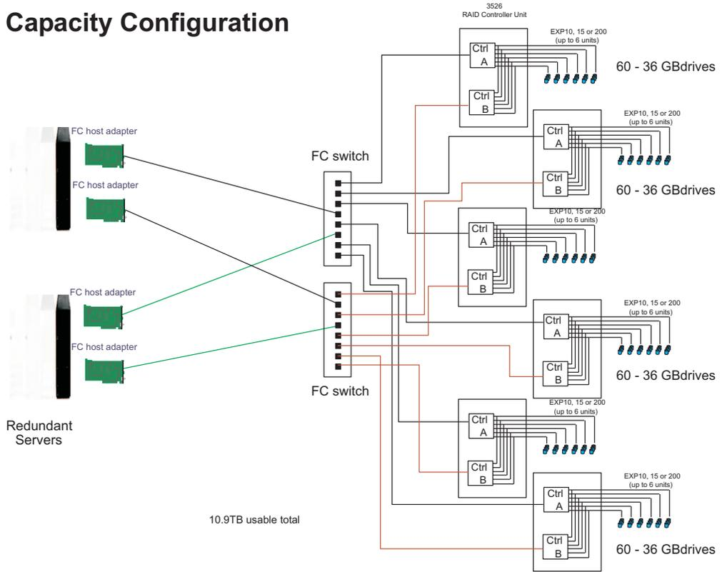
Figure 20. Type 3526 Fibre Channel RAID controller capacity configuration
