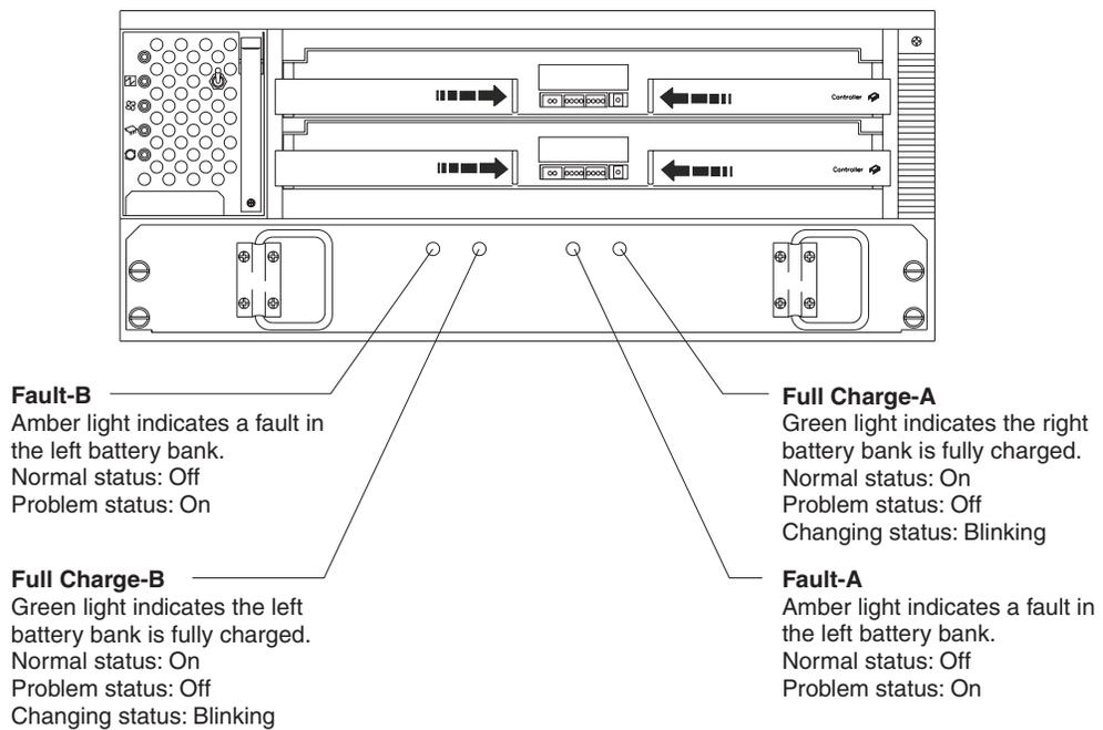
Figure 64. Type 1742 FASiT900 storage server battery indicator lights
