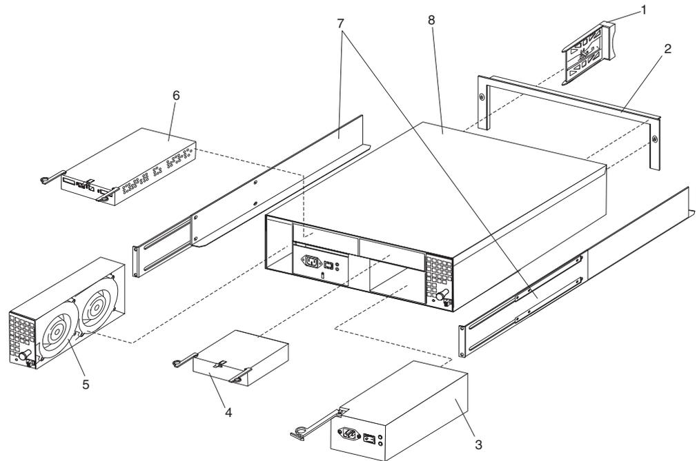
Figure 30. Parts list (FASiT200 Type 3542 and FASiT200 HA Type 3542 controller)
