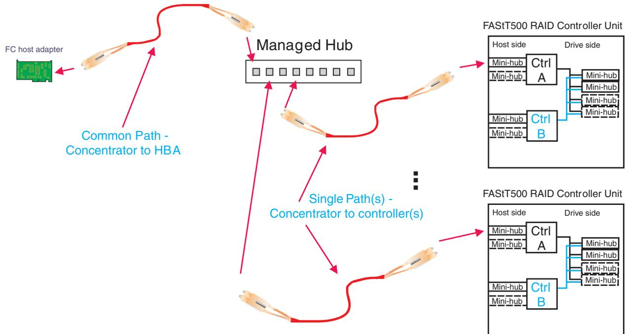
Figure 123. Type 2 configuration with multiple controller units
