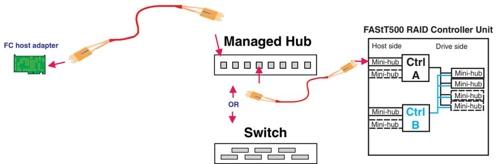
Figure 167. Typical connection path
