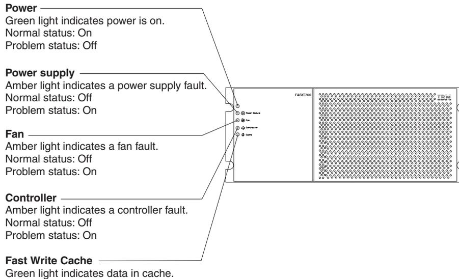
Figure 55. Type 1742 FAStT700 storage server indicator lights
