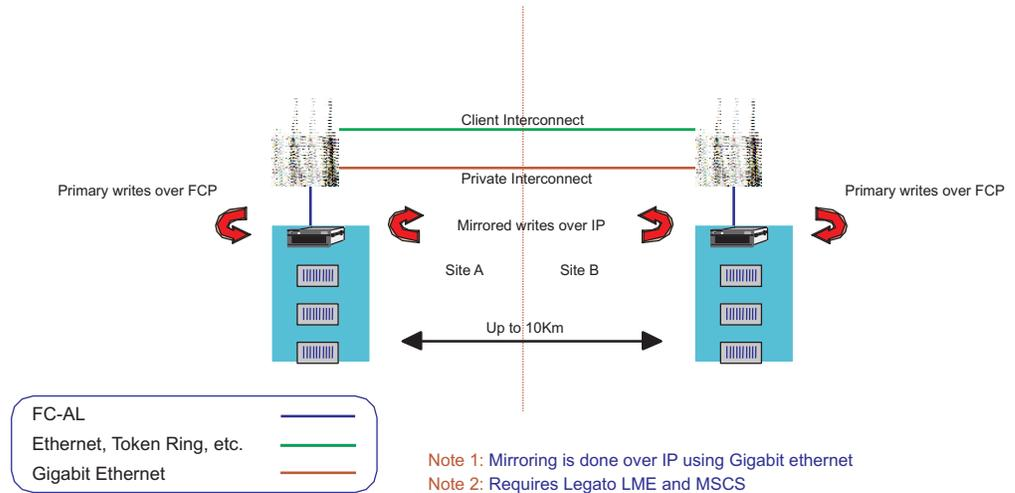
Figure 44. Type 3552 FASi500 RAID controller Legato HA/replication for MS
