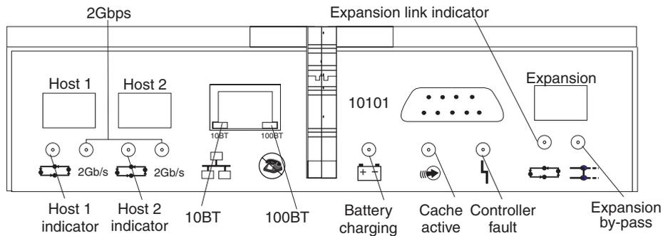
Figure 50. Type 1722 FAStT600 RAID controller LEDs
