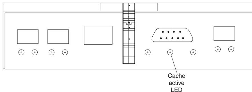
Figure 52. Type 1722 FASiT600 storage server cache active LED
