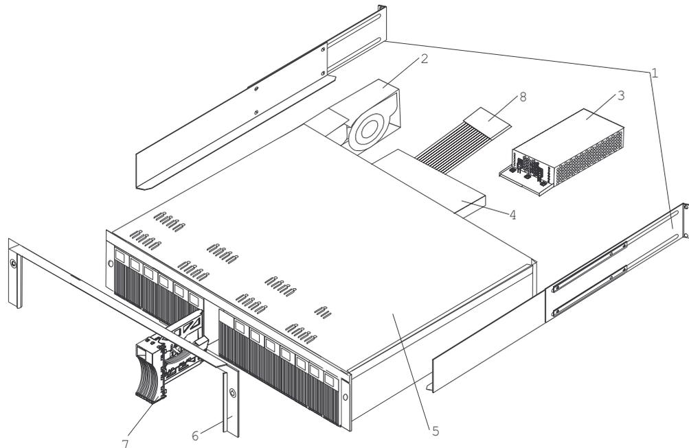
Figure 54. Type 1722 FAST600 storage server parts list
