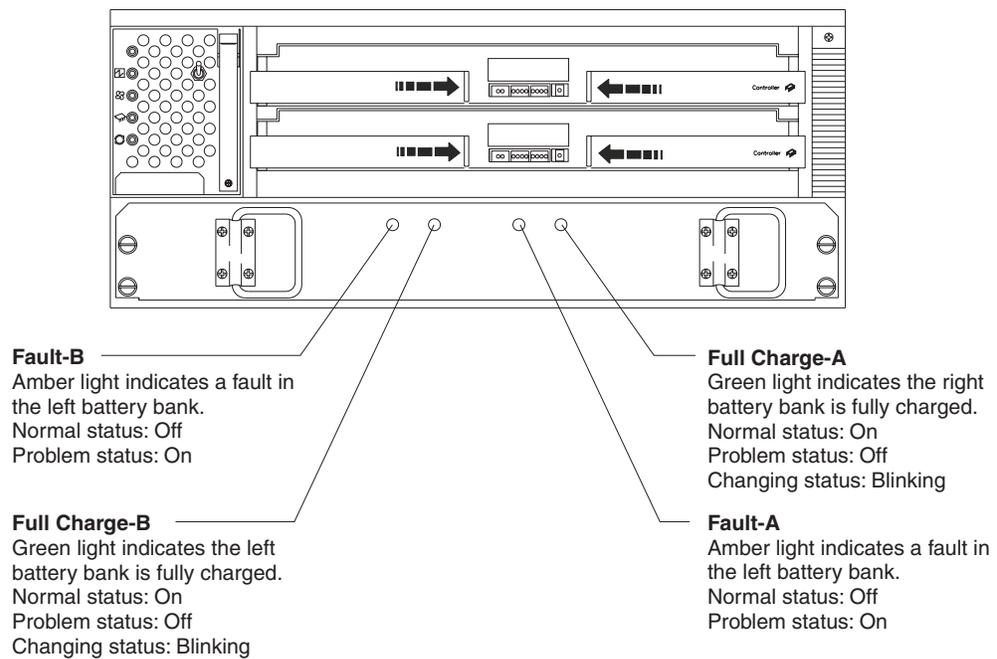
Figure 57. Type 1742 FASi700 storage server battery indicator lights
