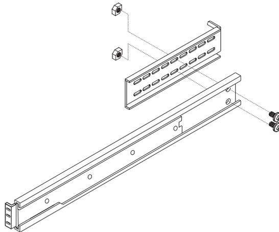
5. Install both slide-rail assemblies in the rack cabinet:
