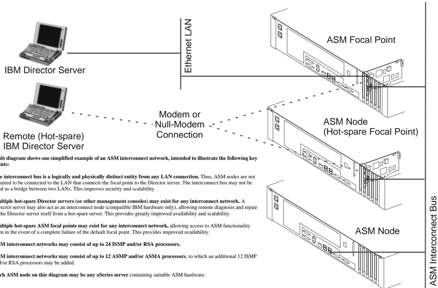
This diagram shows one simplified example of an ASM interconnect network, intended to illustrate the following key points:
