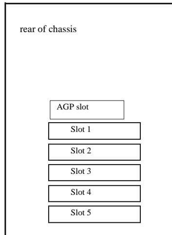
All PCI expansion slots are full-length, 32-bit, 33MHz, 5V or universal on a single PCI bus.
