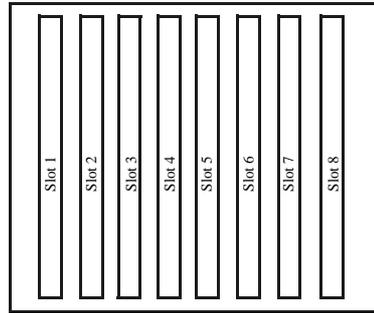
All slots are full-length, 64-bit, 66MHz, 3.3V (5V tolerant).
