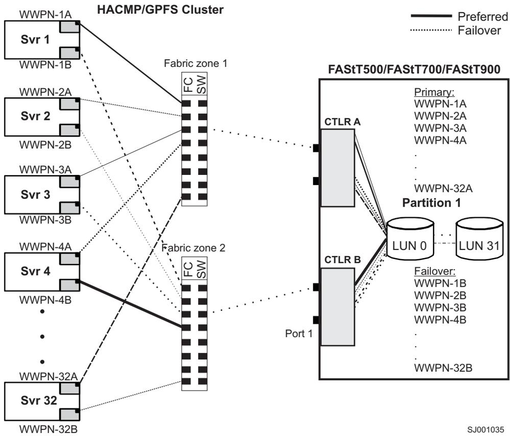
Figure 18. HACMP/GPFS cluster configuration with single FAST500/700/900, shown with one partition per FAST
