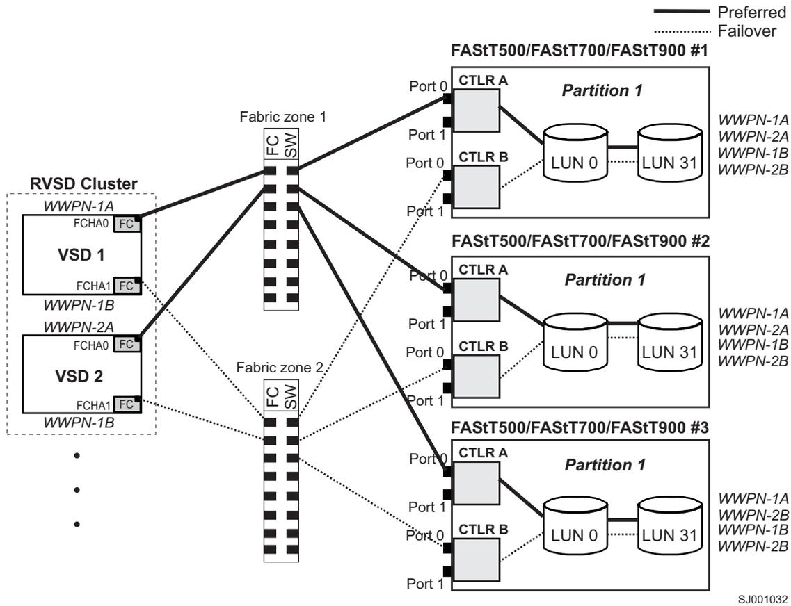
Figure 15. RVSD cluster configuration with multiple FAST500/700/900 - Storage Manager 8.3, shown with one partition per FAST
