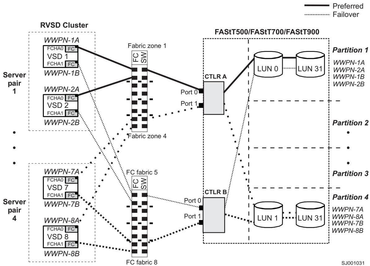
Figure 14. RVSD cluster configuration with single FASt500/700/900 - Storage Manager 8.3, shown with two partitions (four maximum) per FASt
