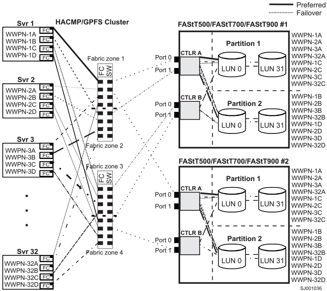
Figure 19. HACMP/GPFS cluster configuration with multiple FAST500/700/900, shown with two partitions per FAST
