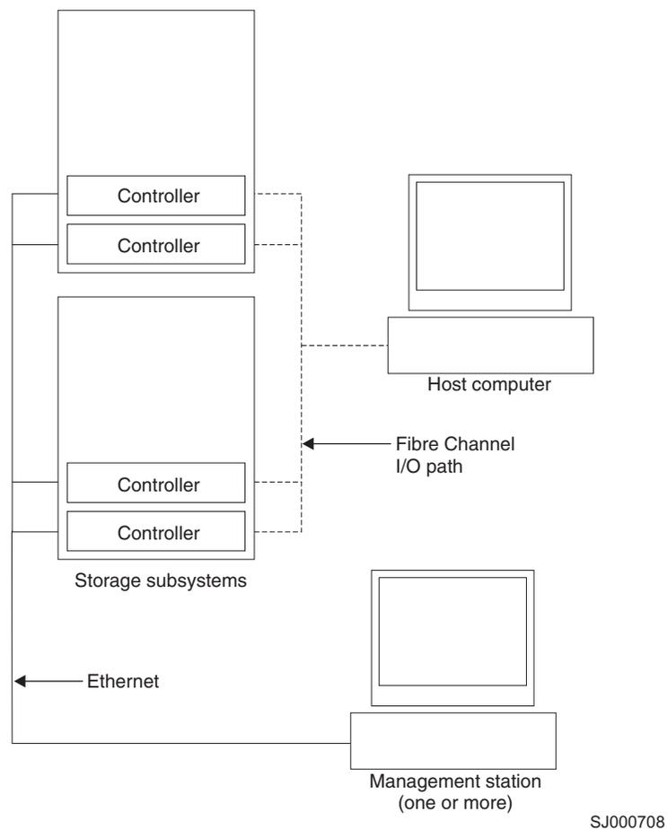
Figure 3. Direct (out-of-band) managed storage subsystems
