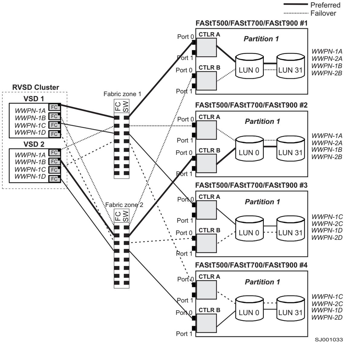
Figure 16. Typical RVSD cluster configuration with multiple FAS T500/700/900 - Storage Manager 8.3, shown with one partition per FAS T
