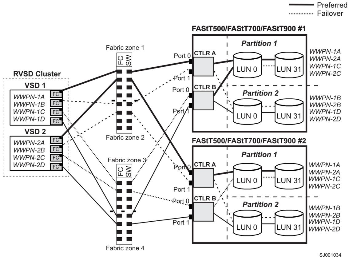
Figure 17. RVSD cluster configuration with multiple FAST500/700/900 - Storage Manager 8.3, shown with two partitions per FAST
