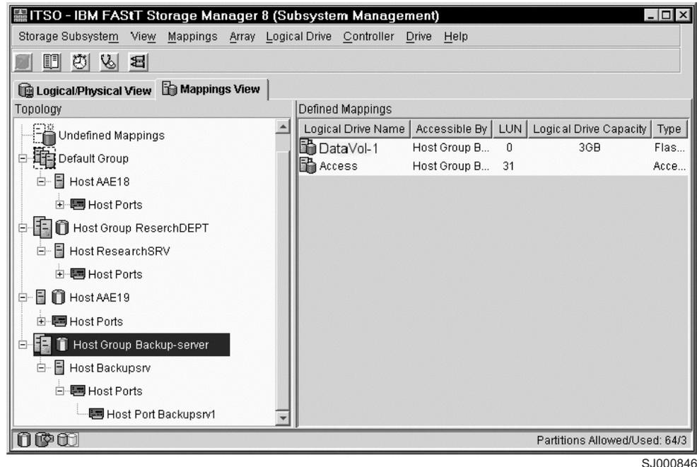
Figure 36. Mapped FlashCopy logical disk
