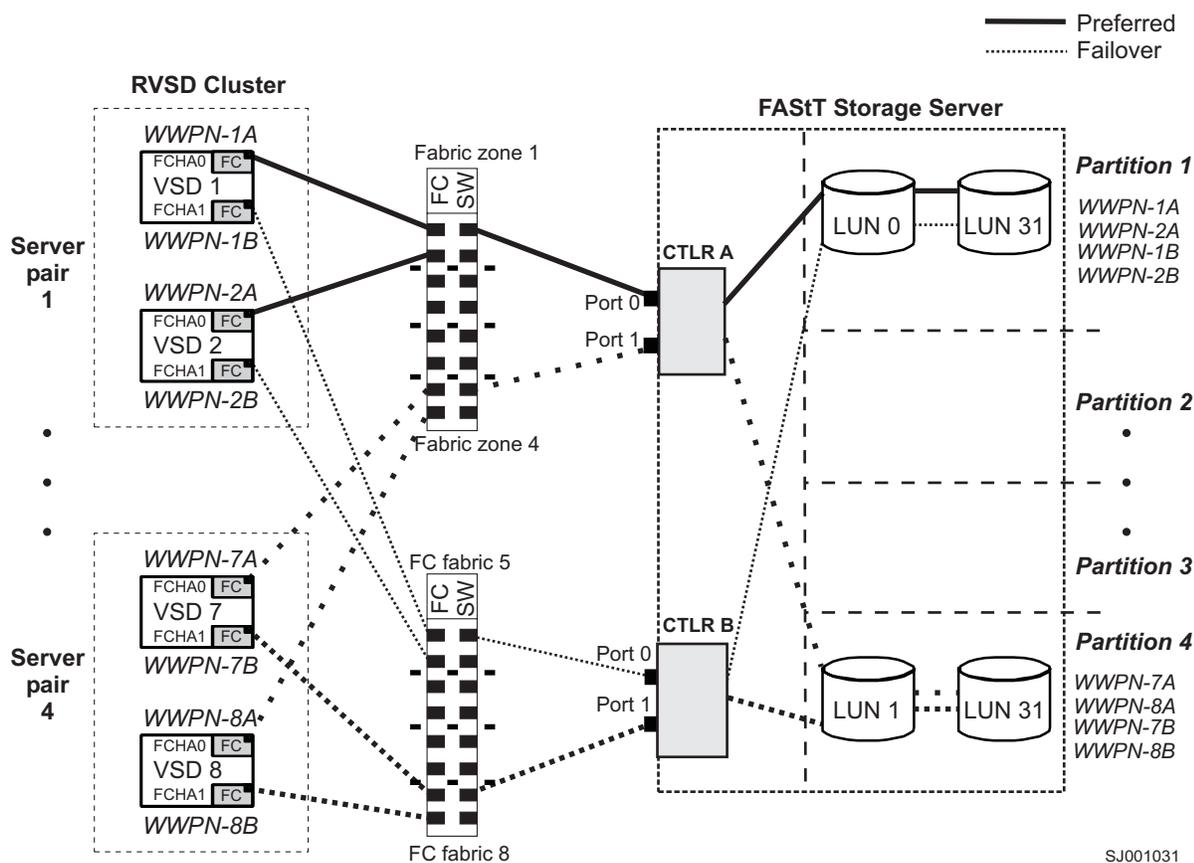
Figure 15. Cluster configuration with single FAStT storage server — one to four partitions
