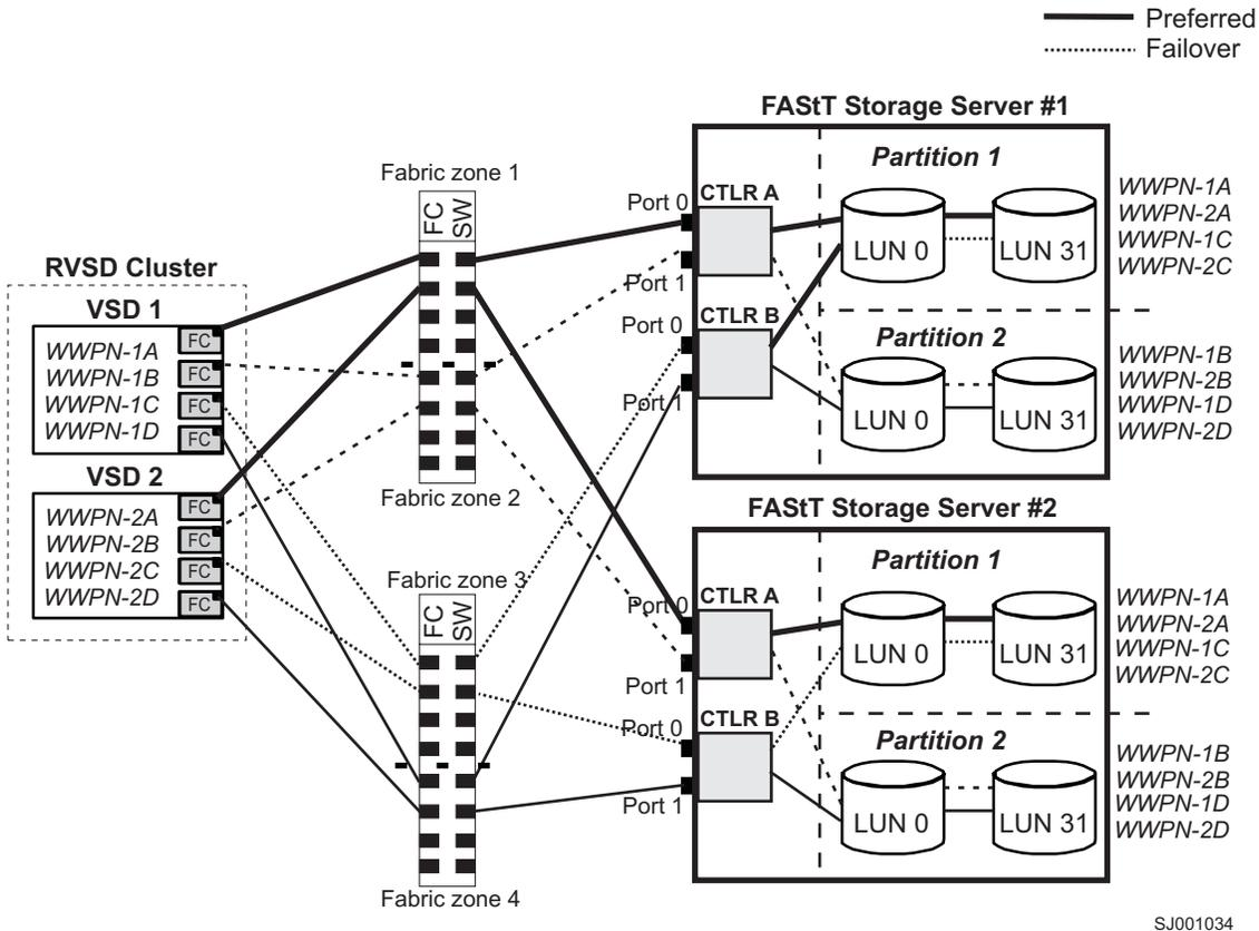
Figure 18. RVSD cluster configuration with two FASTt storage servers — two partitions per FASTt
