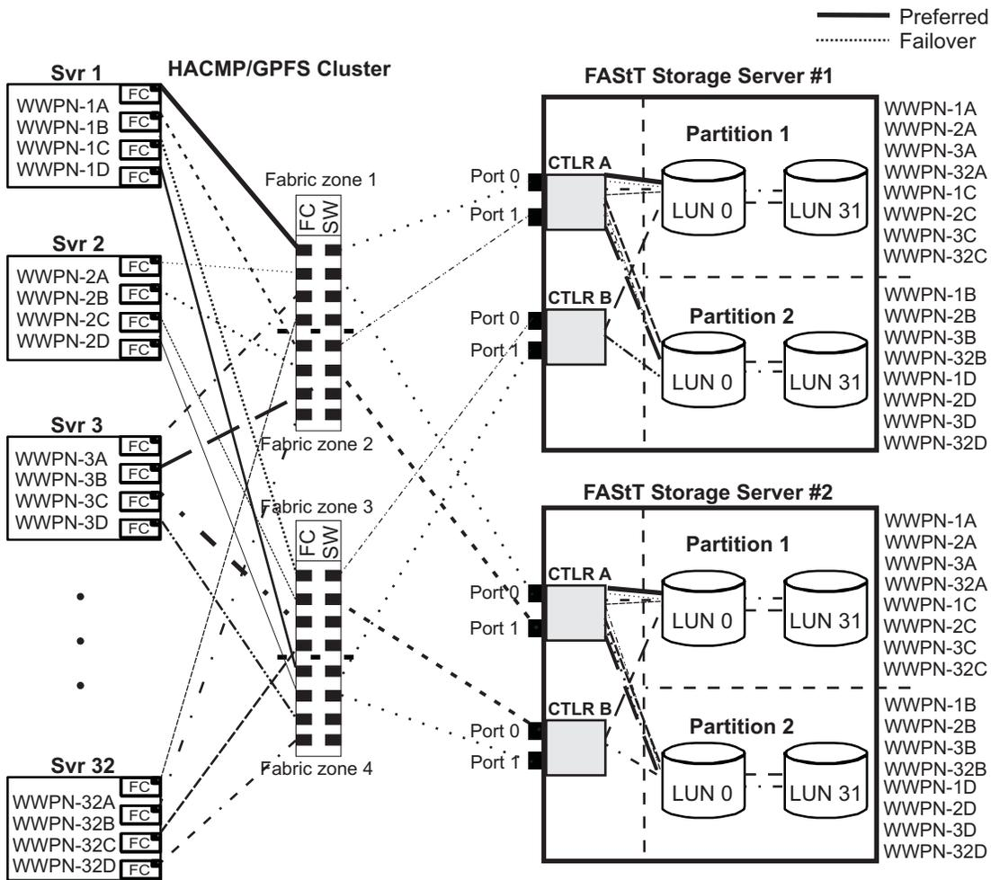
Figure 20. HACMP/GPFS cluster configuration with two FAST storage servers — two partitions per FAST
