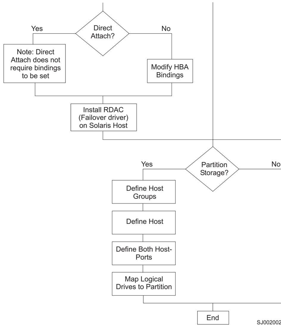
Figure 6. Installation process (part 3)
