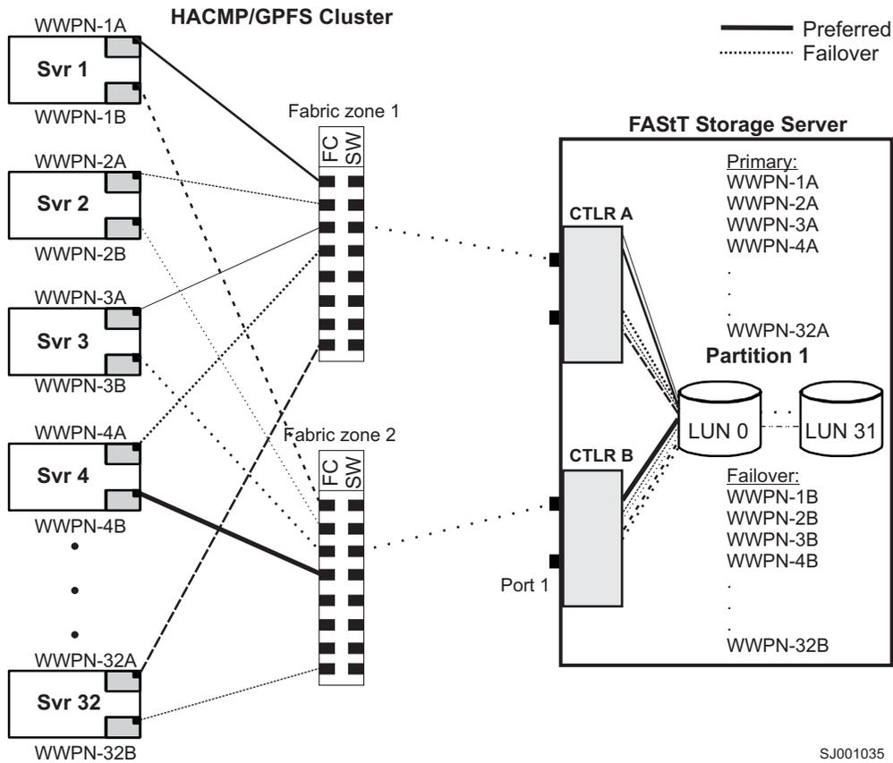
Figure 19. HACMP/GPFS cluster configuration with one FAST storage server — one partition
