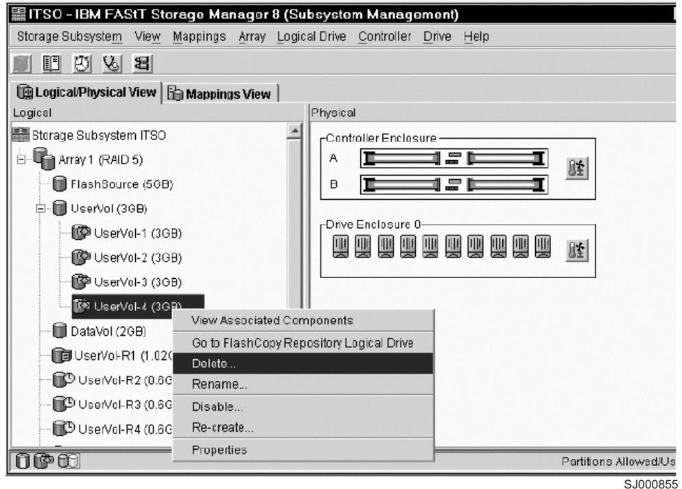
Figure 43. Deleting the FlashCopy logical drive
