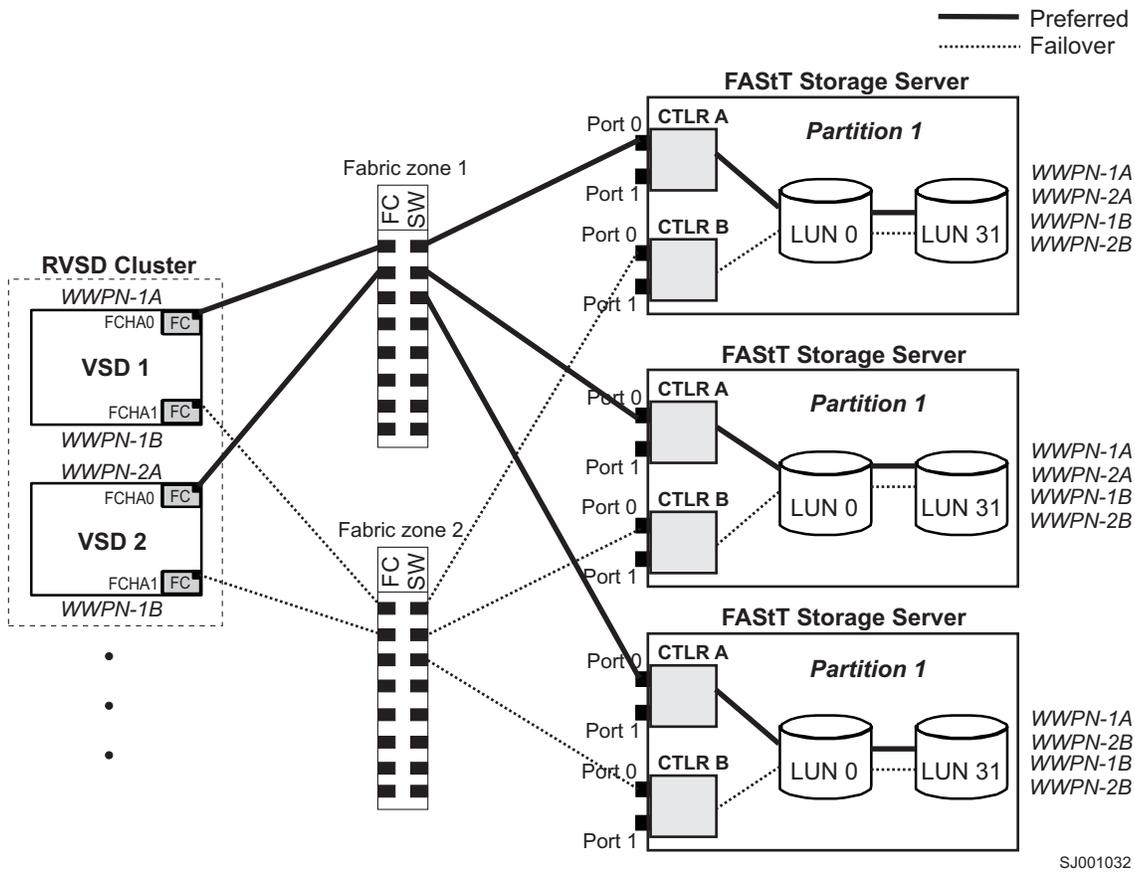
Figure 16. Cluster configuration with three FAST storage servers — one partition per FAST
