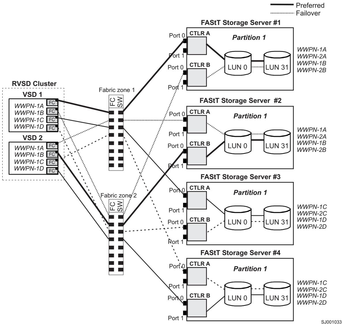
Figure 17. Cluster configuration with four FAST storage servers — one partition per FAST
