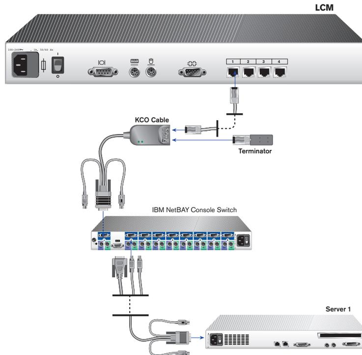
**Figure 2.5: LCM Configuration with a Legacy KVM Switch**
