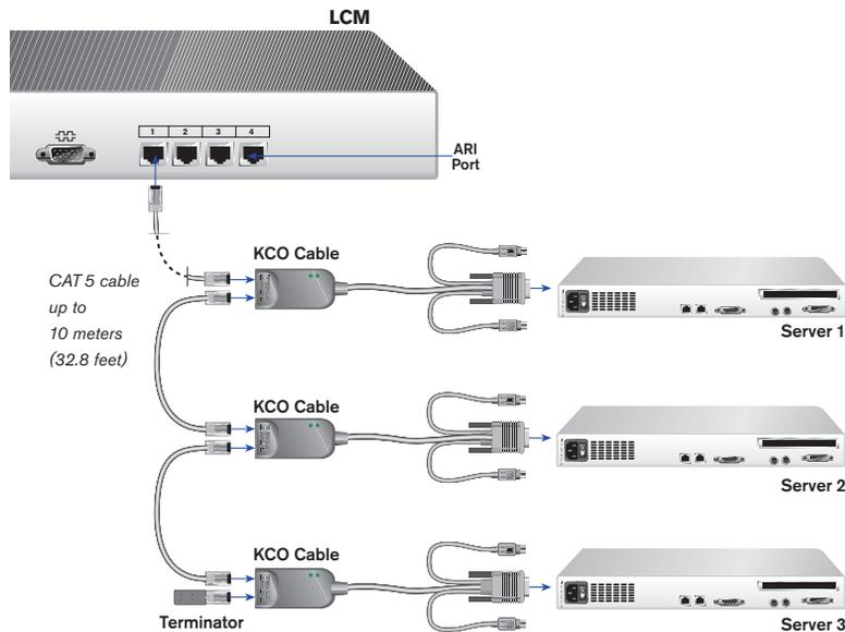
**Figure 2.4: Chaining Servers Together with KCO Cables**
