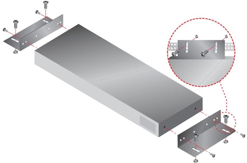
**Figure 2.1: LCM Vertical Installation**
