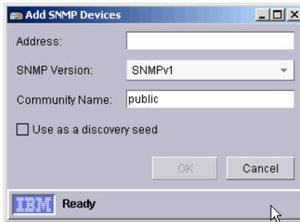
**Figure 8 – Add SNMP Device**
