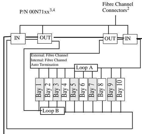
**IN** = primary or secondary (redundant) connection from FAStT500 Storage Server or previous FAStT EXP500 Storage Expansion Unit daisy-chained from the storage server
