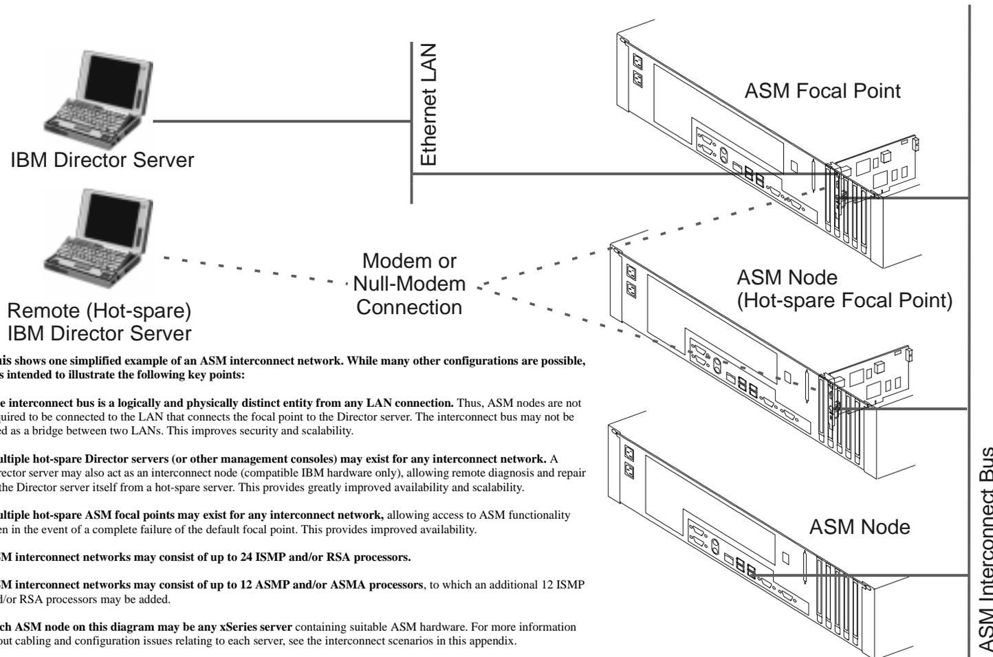
This shows one simplified example of an ASM interconnect network. While many other configurations are possible, it is intended to illustrate the following key points:
