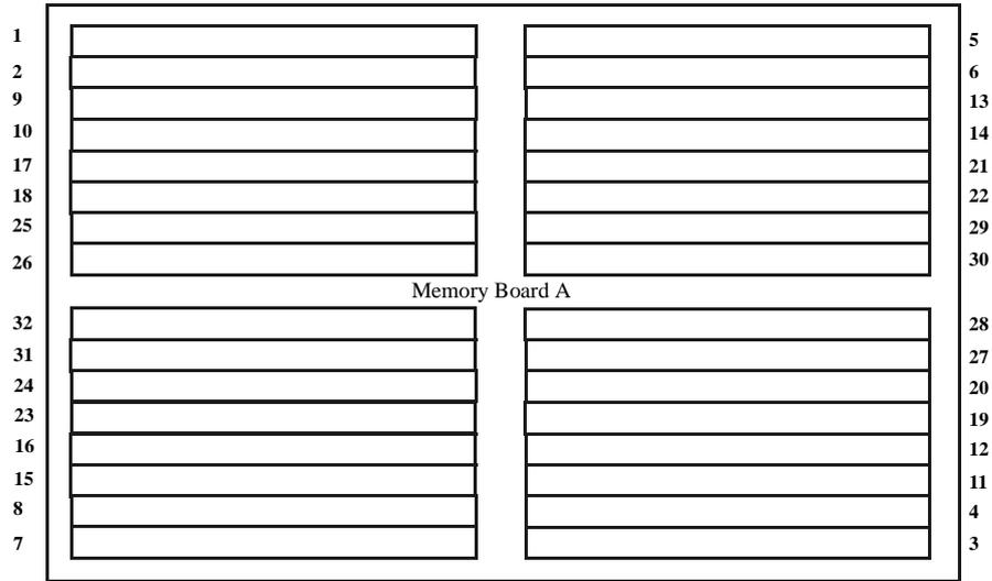
Install memory options according to the order shown for Memory Board A above. Repeat for Memory Board B.
