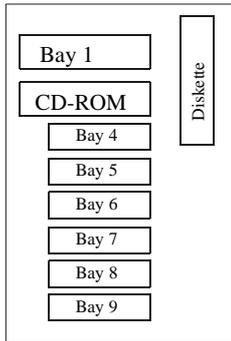
1. IDE models support a maximum of four IDE devices including CD-ROM drives, IDE hard disk drives and IDE tape drives.
