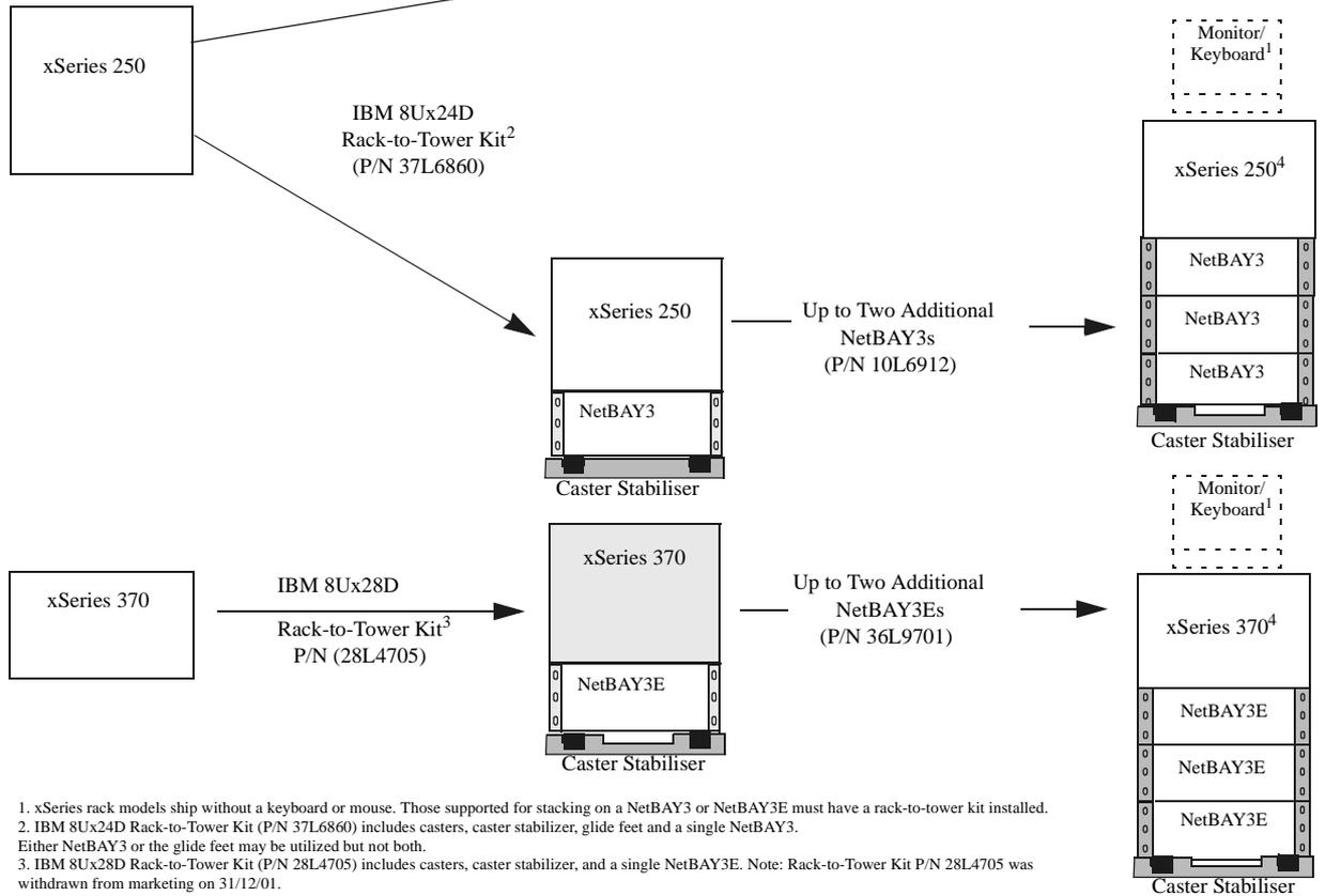
1. xSeries rack models ship without a keyboard or mouse. Those supported for stacking on a NetBAY3 or NetBAY3E must have a rack-to-tower kit installed.
