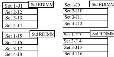
All RDIMMs installed in each set must be the same size, but all the sets do not have to contain RDIMMs of the same size. Install RDIMM sets in numerical sequence from one to four.
