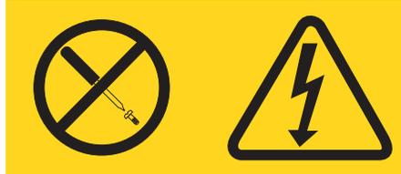
Hazardous voltage, current, and energy levels are present inside any component that has this label attached. There are no serviceable parts inside these components. If you suspect a problem with one of these parts, contact a service technician.
