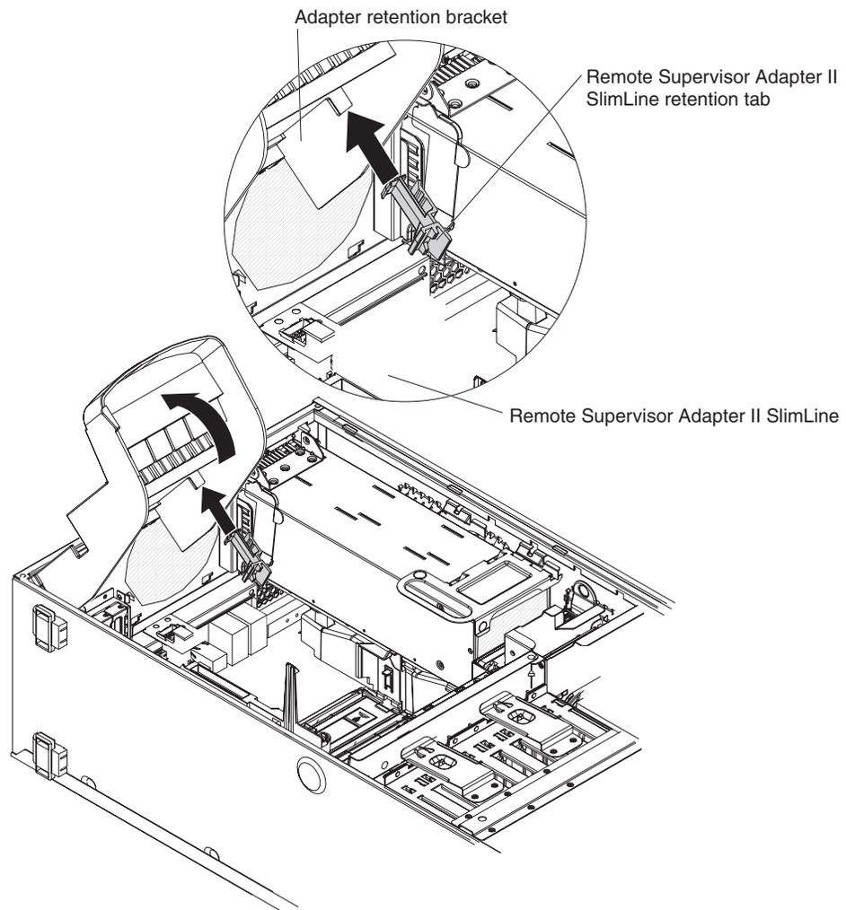
7. Carefully grasp the Remote Supervisor Adapter II SlimLine by its top edge or upper corners, and align it with the Remote Supervisor Adapter II SlimLine guide and the connector on the system board.
