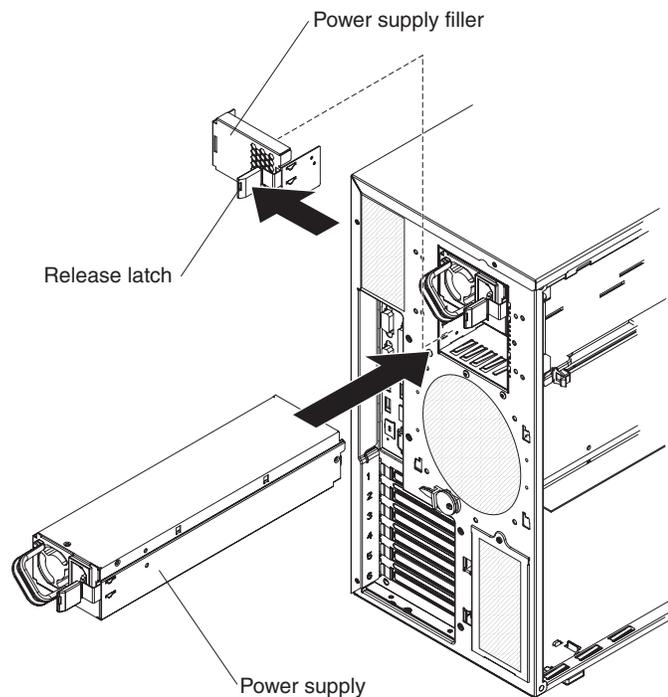
7. Press down on the orange release lever and push the power supply toward the front of the chassis until it locks into place.
