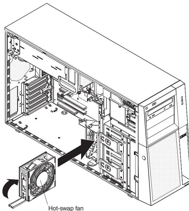
7. Lower the fan into the slot and press down on the fan until it locks into place; then close the handle to the locked position.
