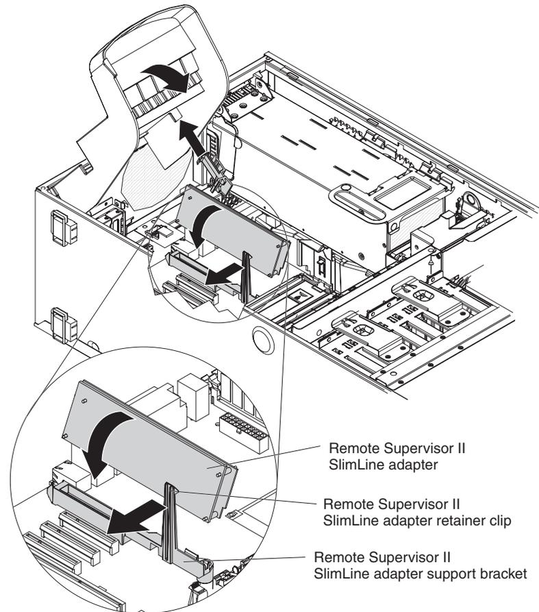
8. Press the Remote Supervisor Adapter II SlimLine firmly into the connector and under the retention clip on the Remote Supervisor Adapter II SlimLine support bracket.
