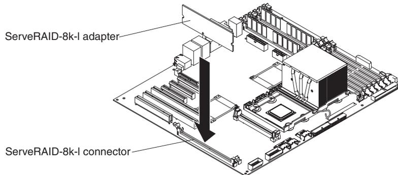
6. Press the ServeRAID 8k-I adapter firmly into the connector.
