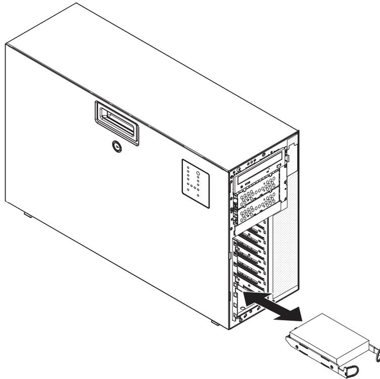
**Note:** If the server is configured for RAID operation using an optional ServeRAID adapter, you might have to reconfigure your disk arrays after installing hard disk drives. See the ServeRAID documentation on the *IBM ServeRAID Support CD* for additional information about RAID operation and complete instructions for using ServeRAID Manager.
