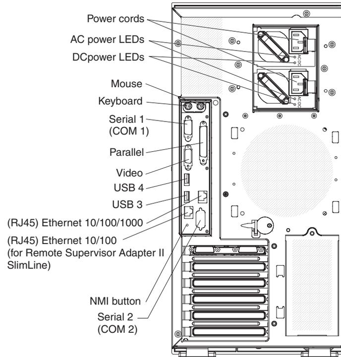
The following illustration shows the connectors on the rear of the non-hot-swap power supply models. For more information about these connectors, see “Server components” on page 17.
