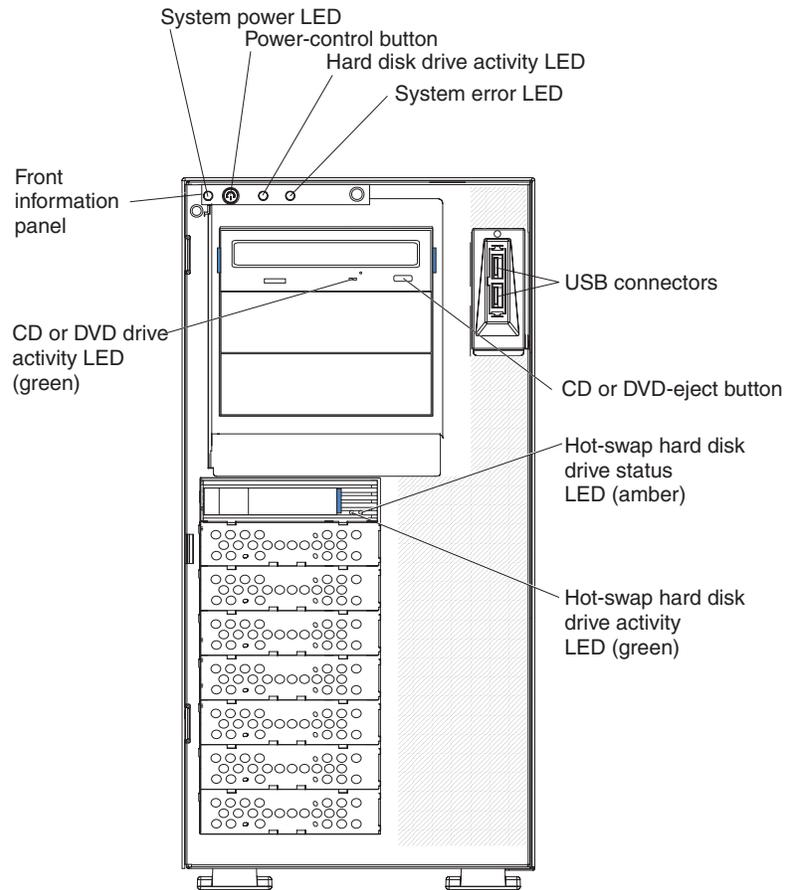
The following illustration shows the controls, LEDs, and connectors on the front of the simple-swap server models.
