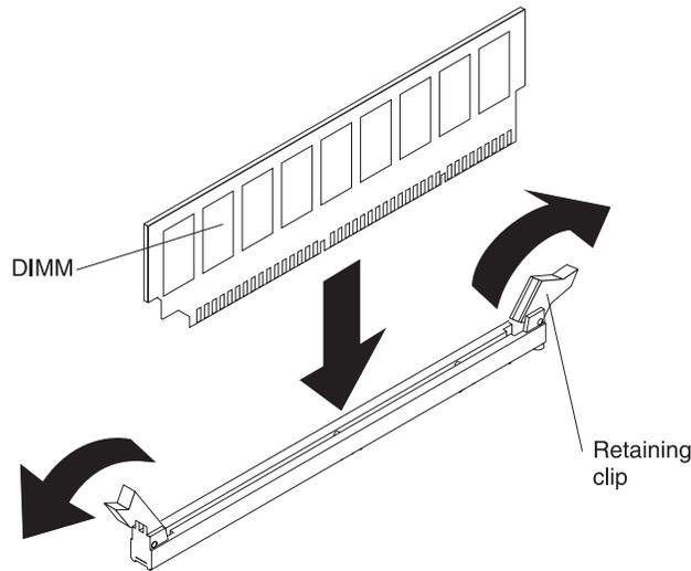
8. Touch the static-protective package that contains the DIMM to any unpainted metal surface on the server. Then, remove the new DIMM from the package.
