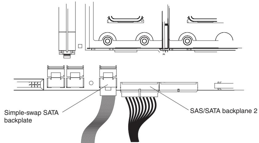
The following illustration shows how the cables must be connected when you install the ServeRAID-8k Controller into the simple-swap SATA model.
